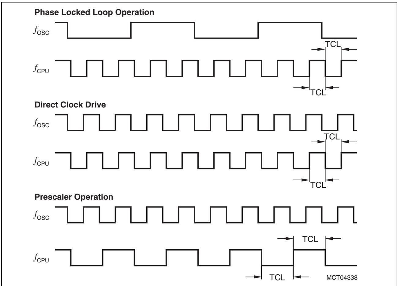
**Figure 10 Generation Mechanisms for the CPU Clock**
