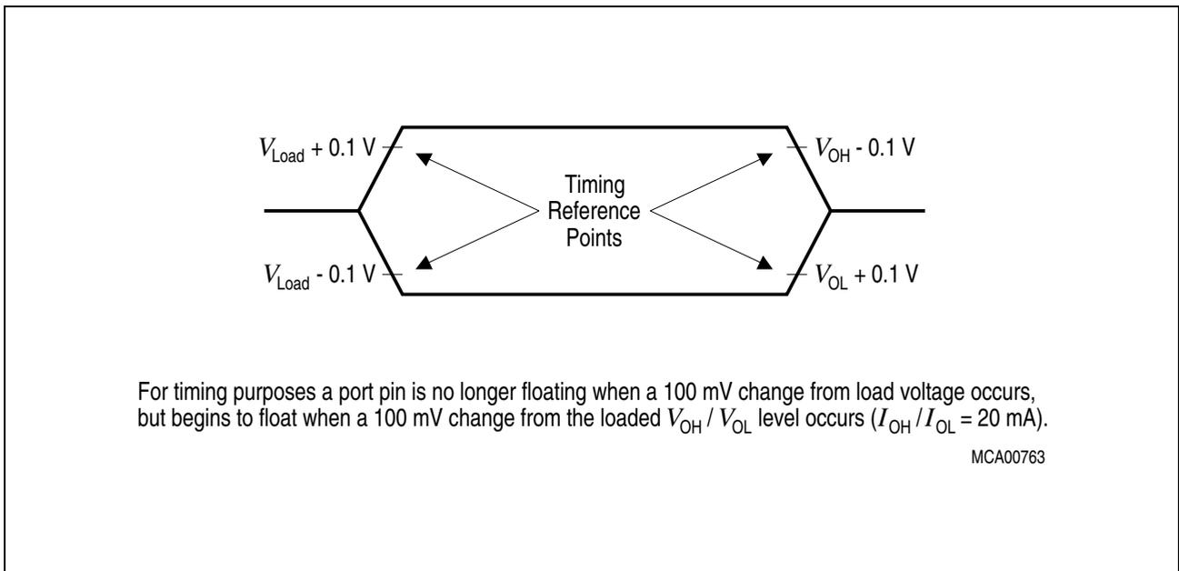
Figure 14 Float Waveforms
