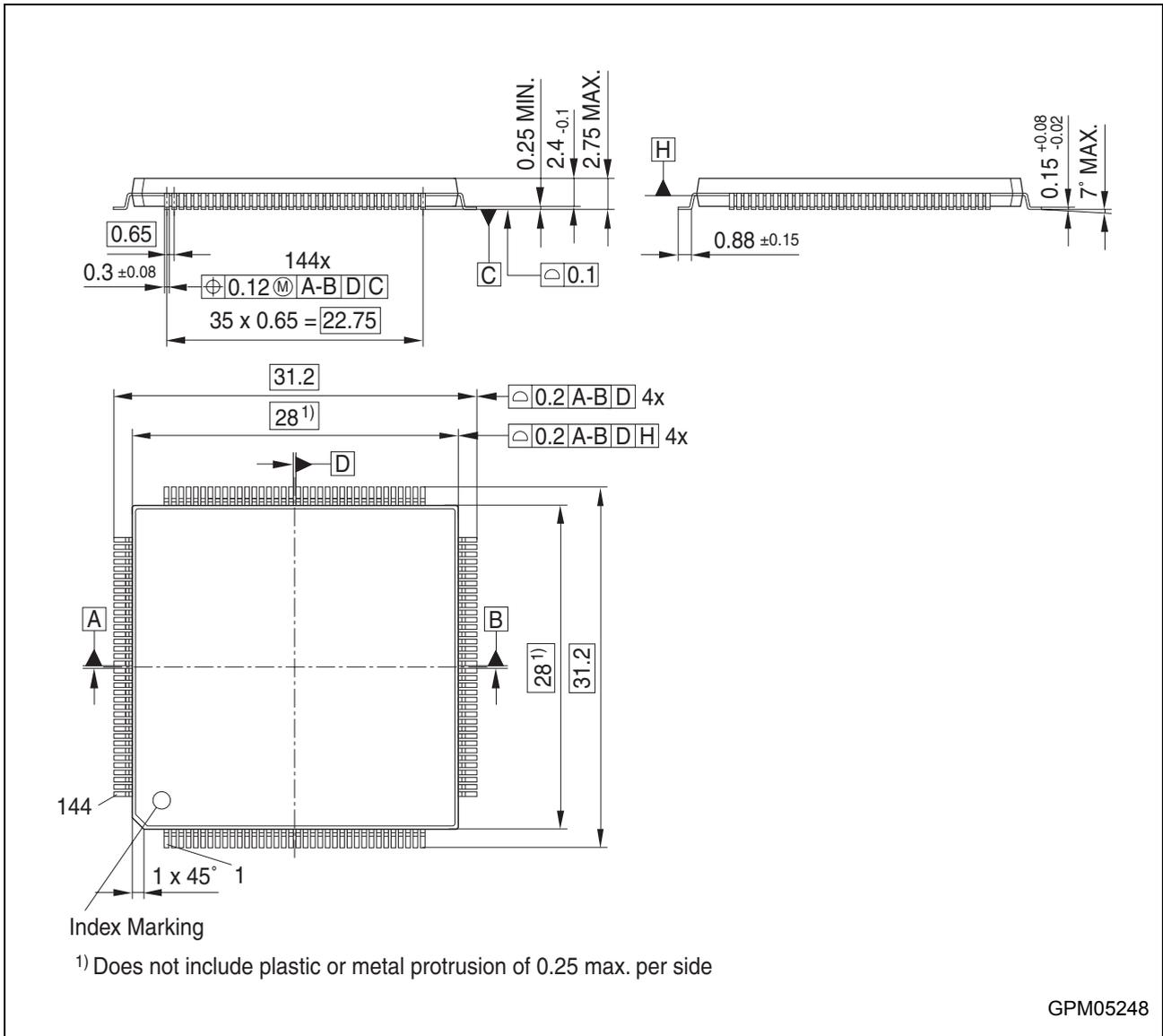
Figure 24 P-MQFP-144-8 (Plastic Metric Quad Flat Package)
