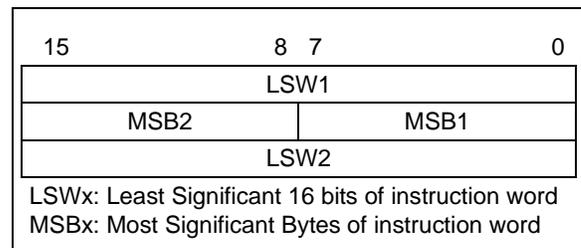
**Note:** When the number of instruction words transferred is odd, MSB2 is zero and LSW2 can not be transmitted.
