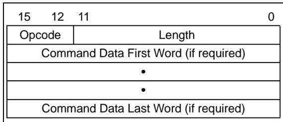
The command opcode must match one of those in the command set. Any command that is received which does not match the list in Table 5-1 will return a “NACK” response (see **Section 5.3.1.1 “Opcode Field”**).
