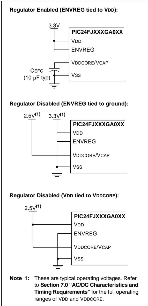
**FIGURE 2-3: CONNECTIONS FOR THE ON-CHIP REGULATOR (28/44-PIN DEVICES)**
