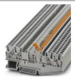
Feed-through terminal block, Connection method: Leg spring connection, Cross section: 0.2 mm² - 4 mm², AWG: 24 - 12, Width: 5.2 mm, Height: 35.3 mm, Color: gray, Mounting type: NS 35/7,5, NS 35/15
