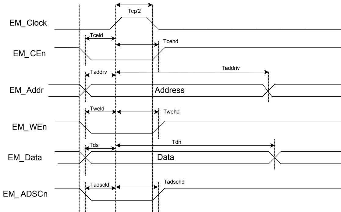
**Table 11-66. Synchronous Write Cycle Specifications**
