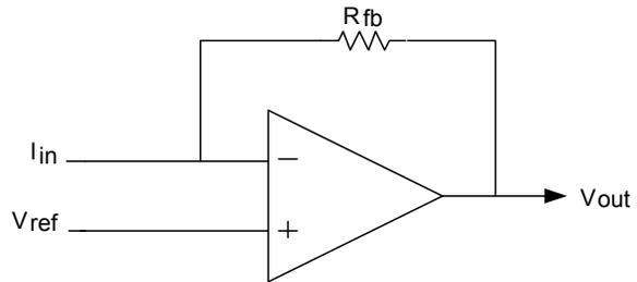
The TIA configuration is used for applications where an external sensor's output is current as a function of some type of stimulus such as temperature, light, magnetic flux etc. In a common application, the voltage DAC output can be connected to the  $V_{REF}$  TIA input to allow calibration of the external sensor bias current by adjusting the voltage DAC output voltage.
