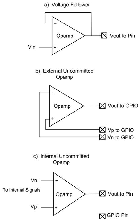
The opamp has three speed modes, slow, medium, and fast. The slow mode consumes the least amount of quiescent power and the fast mode consumes the most power. The inputs are able to swing rail-to-rail. The output swing is capable of rail-to-rail operation at low current output, within 50 mV of the rails. When driving high current loads (about 25 mA) the output voltage may only get within 500 mV of the rails.
