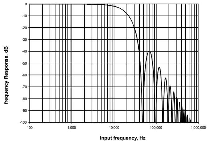
Resolution and sample rate are controlled by the Decimator. Data is pipelined in the decimator; the output is a function of the last four samples. When the input multiplexer is switched, the output data is not valid until after the fourth sample after the switch.
