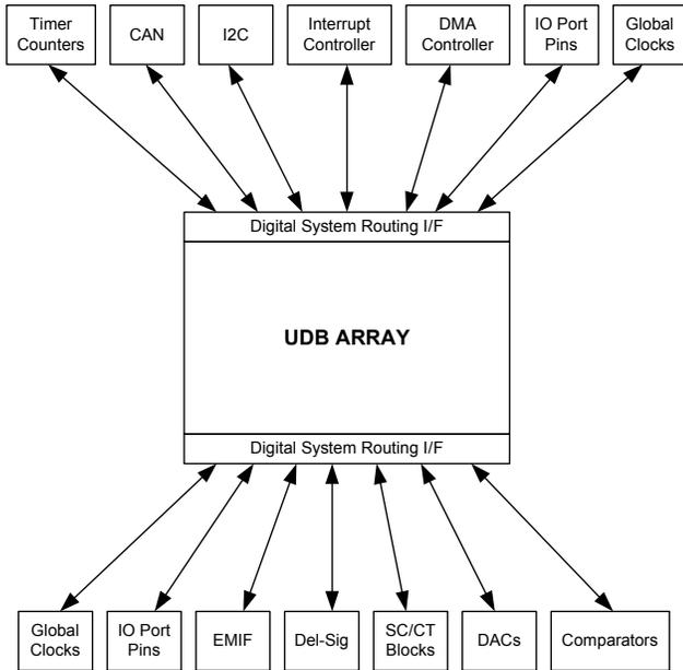
Interrupt and DMA routing is very flexible in the CY8C38 programmable architecture. In addition to the numerous fixed function peripherals that can generate interrupt requests, any data signal in the UDB array routing can also be used to generate a request. A single peripheral may generate multiple independent interrupt requests simplifying system and firmware design. Figure 7-14 shows the structure of the IDMUX (Interrupt/DMA Multiplexer).
