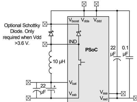
The switching frequency can be set to 100 kHz, 400 kHz, 2 MHz, or 32 kHz to optimize efficiency and component cost. The 100 kHz, 400 kHz, and 2 MHz switching frequencies are generated using oscillators internal to the boost converter block. When the 32-kHz switching frequency is selected, the clock is derived from a 32 kHz external crystal oscillator. The 32-kHz external clock is primarily intended for boost standby mode.
