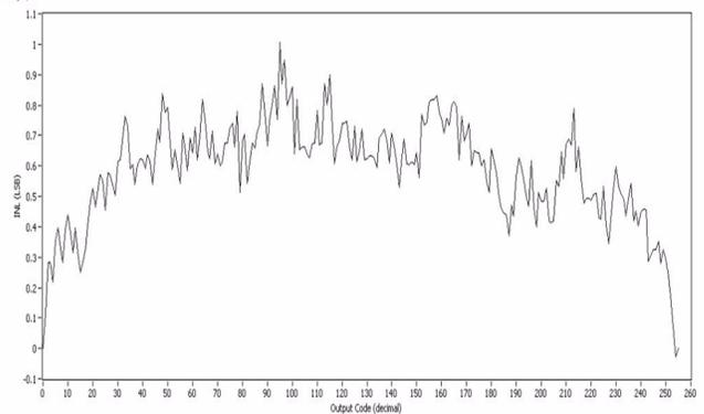
**Figure 11-27. IDAC DNL vs Input Code, Range = 255  $\mu$ A, Source Mode**
