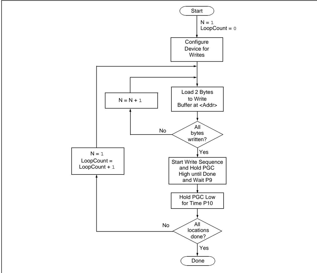
**FIGURE 3-5: TABLE WRITE AND START PROGRAMMING INSTRUCTION TIMING DIAGRAM (1111)**
