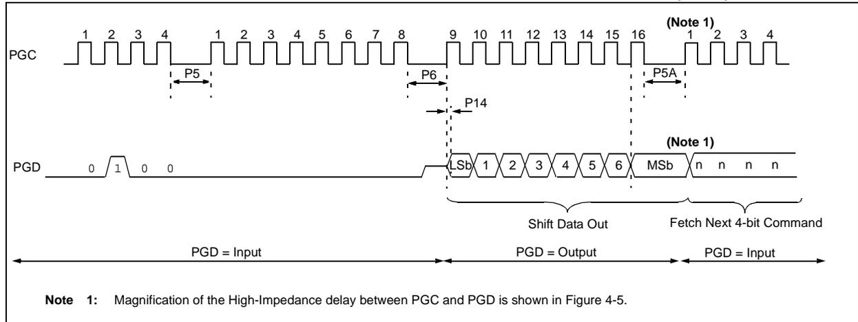
**FIGURE 4-5: HIGH-IMPEDANCE DELAY**
