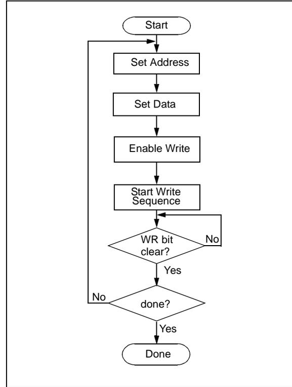
FIGURE 3-7: DATA EEPROM WRITE TIMING DIAGRAM
