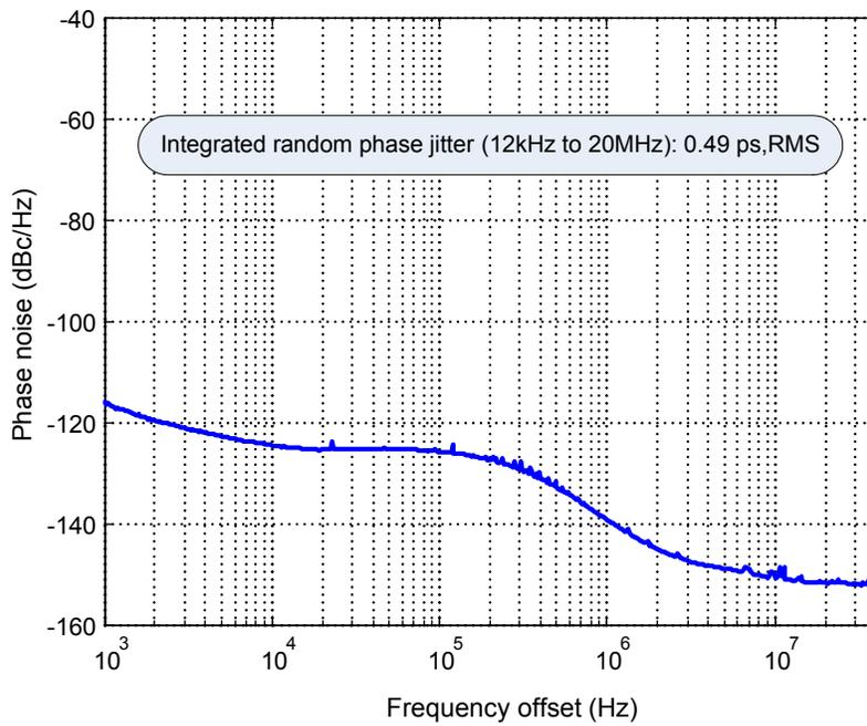
**Figure 1. Phase Noise, 156.25 MHz, 3.3V, LVCMOS Output**
