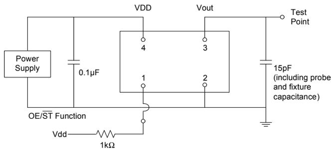
**Figure 2. Test Circuit**
