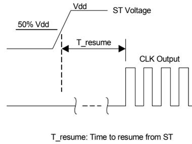
Figure 5. Standby Resume Timing (ST Mode Only)
