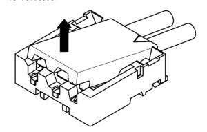
©Lift up to the upper direction and positive lock is released. Removal completes.
