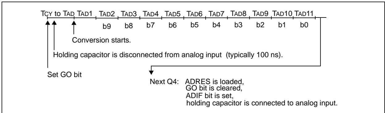
**FIGURE 16-5: FLOW CHART OF A/D OPERATION**
