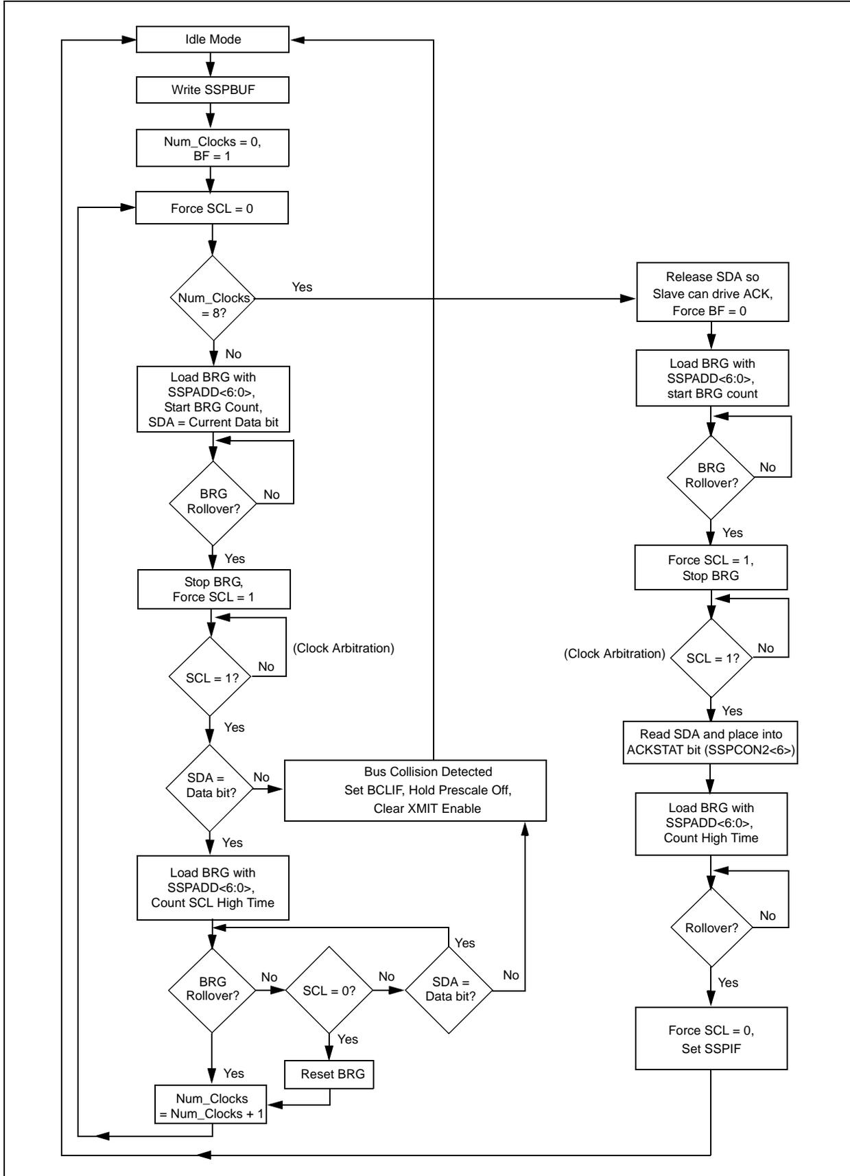
**FIGURE 15-26: I<sup>2</sup>C MASTER MODE TIMING (TRANSMISSION, 7 OR 10-BIT ADDRESS)**
