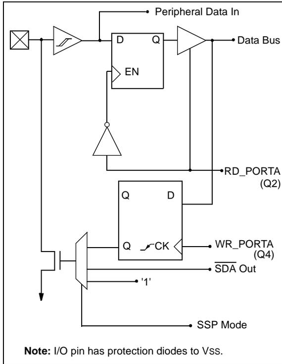
**FIGURE 10-4: RA4 AND RA5 BLOCK DIAGRAM**
