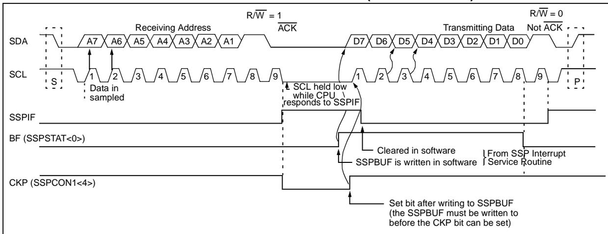
**FIGURE 15-14: I<sup>2</sup>C SLAVE-TRANSMITTER (10-BIT ADDRESS)**
