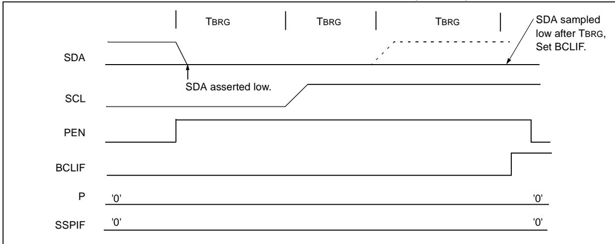
**FIGURE 15-41: BUS COLLISION DURING A STOP CONDITION (CASE 2)**
