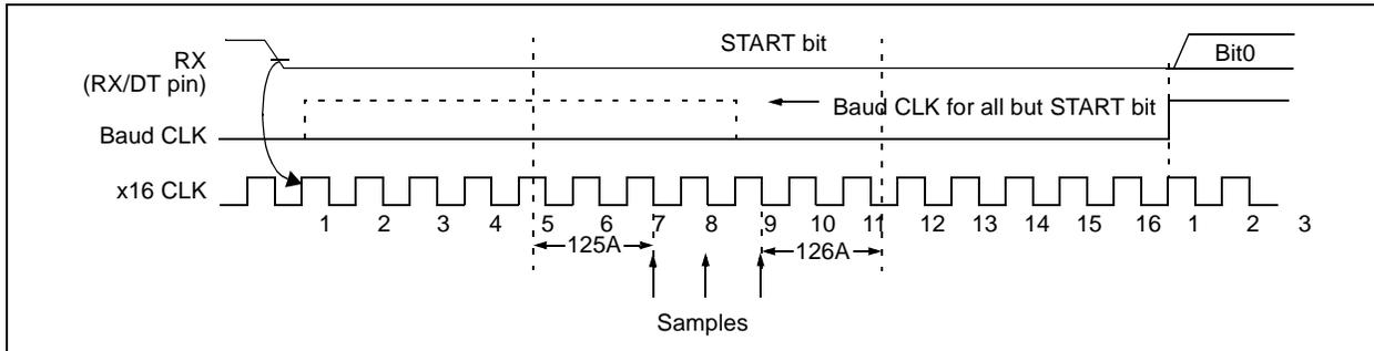
**TABLE 20-17: USART ASYNCHRONOUS RECEIVE SAMPLING REQUIREMENTS**
