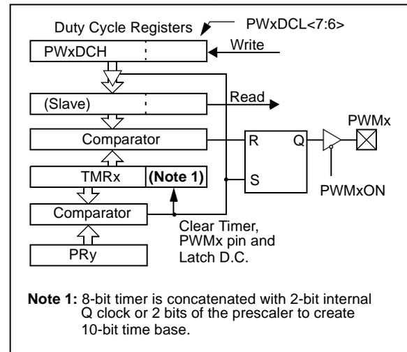
**FIGURE 13-4: PWM OUTPUT (NOT BUFFERED)**
