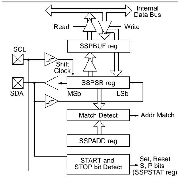
**FIGURE 15-11: I<sup>2</sup>C MASTER MODE BLOCK DIAGRAM**
