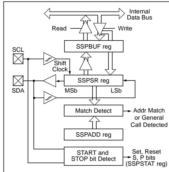
**FIGURE 15-3: I<sup>2</sup>C MASTER MODE BLOCK DIAGRAM**
