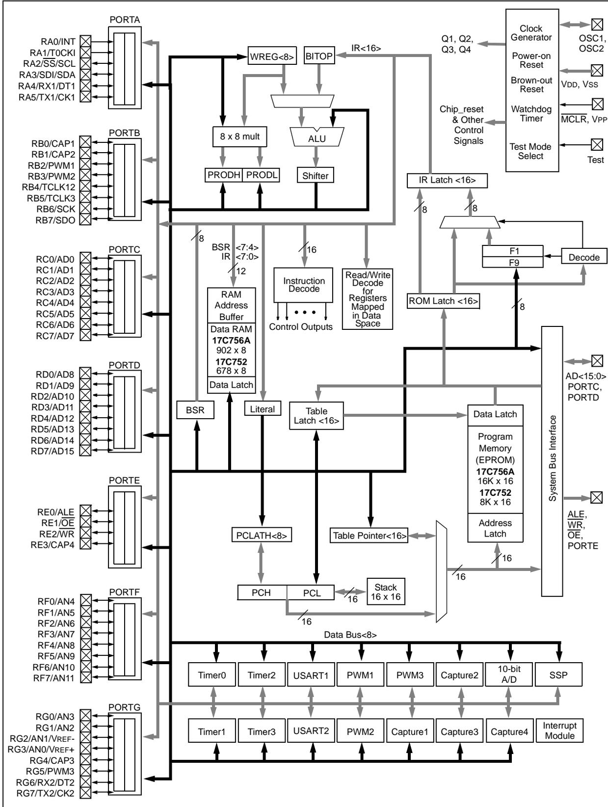
**FIGURE 3-2: PIC17C762/766 BLOCK DIAGRAM**
