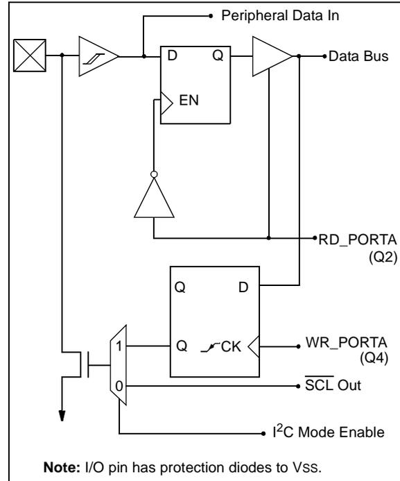
**FIGURE 10-3: RA3 BLOCK DIAGRAM**
