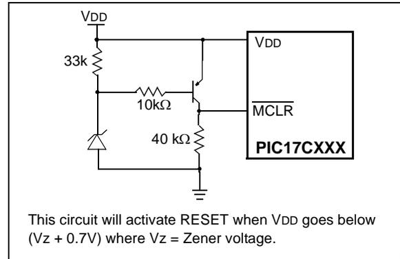
**FIGURE 5-9: EXTERNAL BROWN-OUT PROTECTION CIRCUIT 2**
