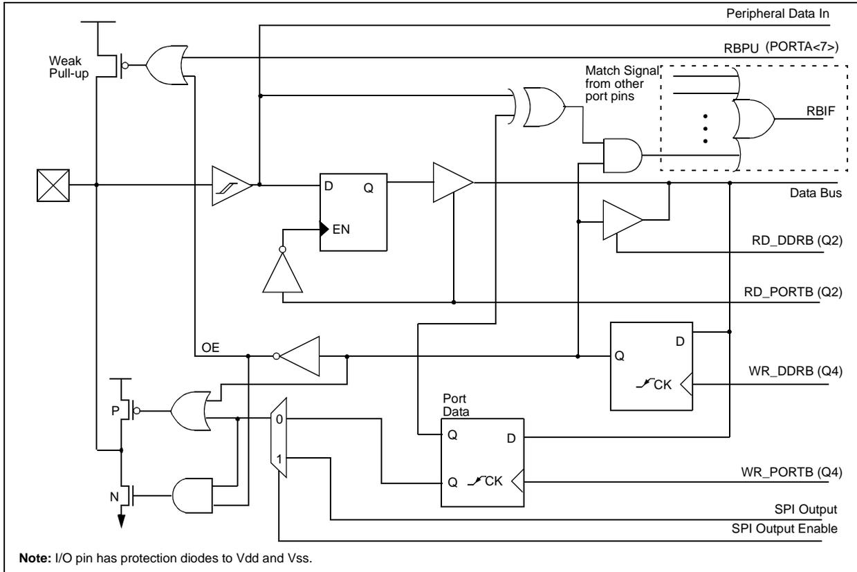
**FIGURE 10-8: BLOCK DIAGRAM OF RB7 PORT PIN**
