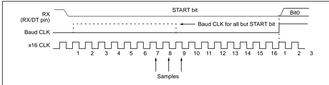
**FIGURE 14-6: START BIT DETECT**
