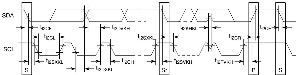
Figure 37. I<sup>2</sup>C Bus AC Timing Diagram
