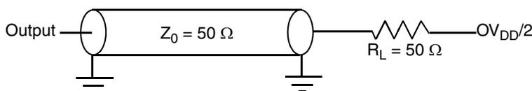
**Figure 36. I<sup>2</sup>C AC Test Load**
