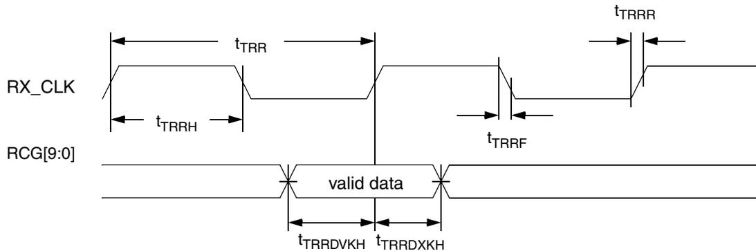
**Figure 18. TBI Single-Clock Mode Receive AC Timing Diagram**
