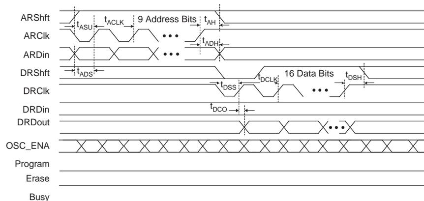
Figure 5-4. UFM Program Waveforms
