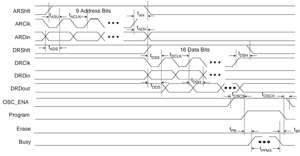
Figure 5-5. UFM Erase Waveform
