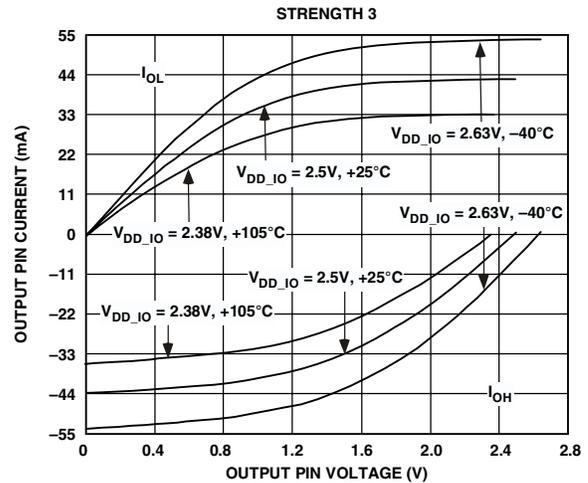
Figure 29. Typical Drive Currents at Strength 3
