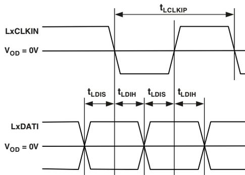
Figure 25. Link Ports—Data Input Setup and Hold<sup>1</sup>
