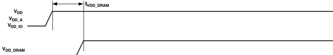
Figure 12. Power-Up Timing
