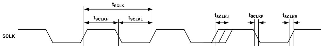
Figure 10. Reference Clocks—System Clock (SCLK) Cycle Time
