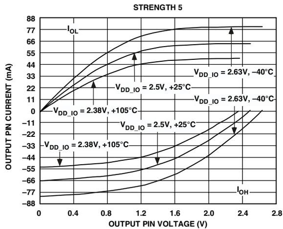
Figure 31. Typical Drive Currents at Strength 5
