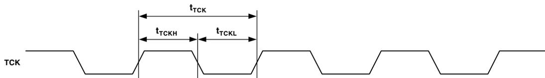
Figure 11. Reference Clocks—JTAG Test Clock (TCK) Cycle Time
