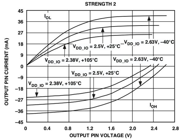
Figure 28. Typical Drive Currents at Strength 2
