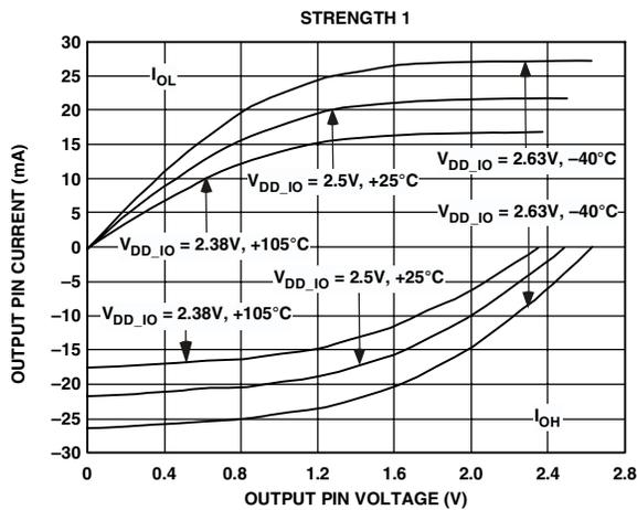
Figure 27. Typical Drive Currents at Strength 1
