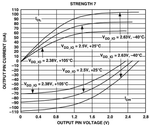
Figure 33. Typical Drive Currents at Strength 7
