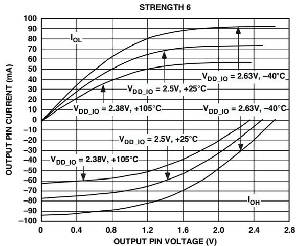
Figure 32. Typical Drive Currents at Strength 6
