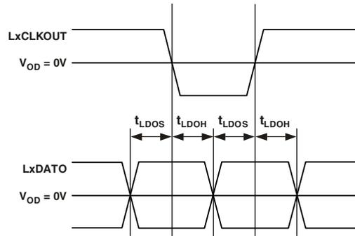
Figure 20. Link Ports—Data Output Setup and Hold<sup>1</sup>
