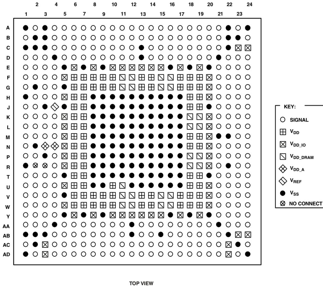
Figure 46. 576-Ball BGA\_ED Pin Configurations<sup>1</sup> (Top View, Summary)
