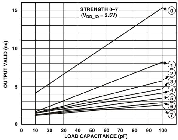
Figure 45. Typical Output Valid ( $V_{DD\_IO} = 2.5 V$ ) vs. Load Capacitance at Max Case Temperature and Strength 0 to 7<sup>1</sup>
