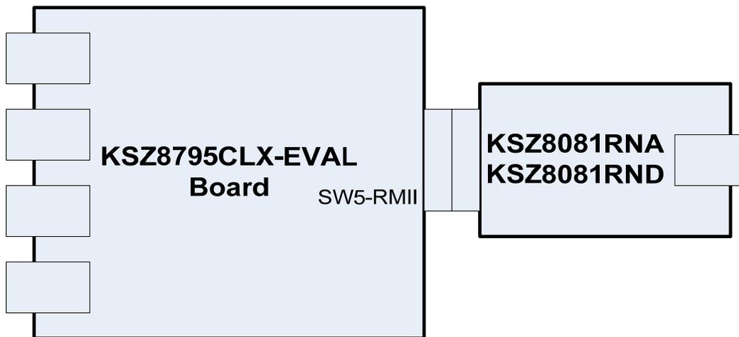
3. From the Figure shows above, when KSZ8795-EVAL board connect with KSZ8081 family PHY evaluation boards for RMII access.
