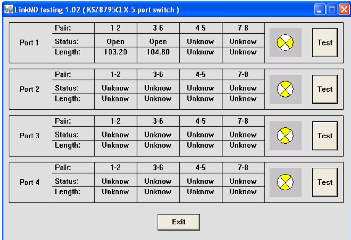
The test result shows both MDIX mode for pair 3-6 and MDI mode for 1-2 pair. The detail LinkMD diagnostic testing configuration is described in the datasheet.
