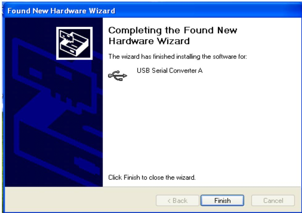
Click 'Finish' button. The Window will install another driver called 'USB Serial Converter B'. After the drivers installed, Window Device Manager will show 'USB Serial Converter A' and 'USB Serial Converter B' as below figure. That means the installation successful.
