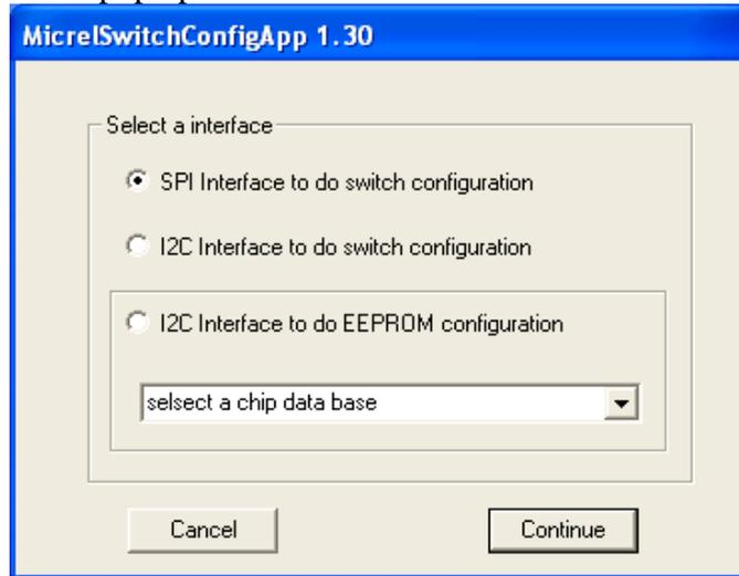
The default is SPI interface to do switch configuration. From the device selection window to select any devices then press 'Continue' button or click 'Continue' button directly, the software tool can detect devices automatically. A control Window will be pop up as follow.
