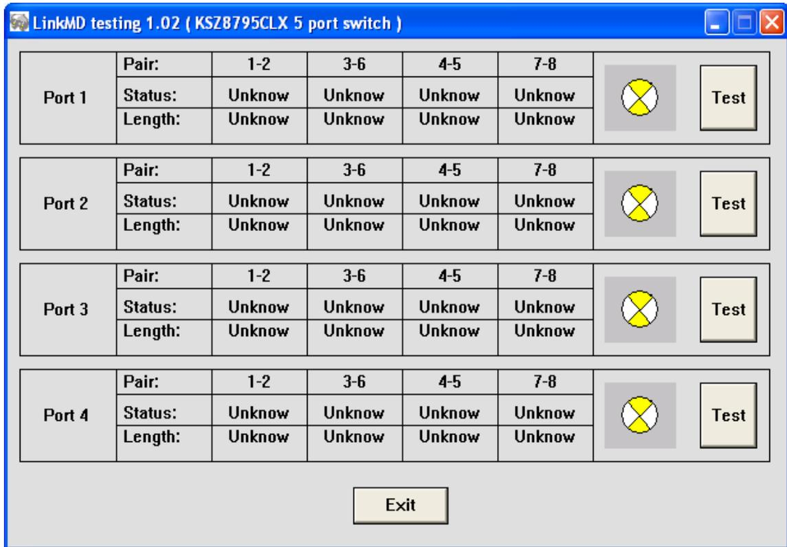
An example for CAT-5 cable diagnostic with open on port 1, just click 'TEST' button, a test result shows as below.
