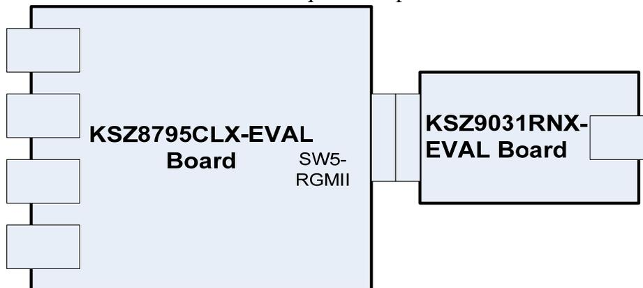
a). Both boards can set 1.8V, 2.5V and 3.3V VDDIO and can set register 86 bits[4:3] of KSZ8795CLX if it is necessary. Please see RGMII section of datasheet for details.
