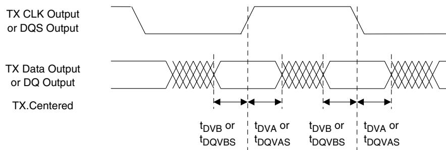
**Figure 3-9. GDDR71 Video Timing Waveforms**
