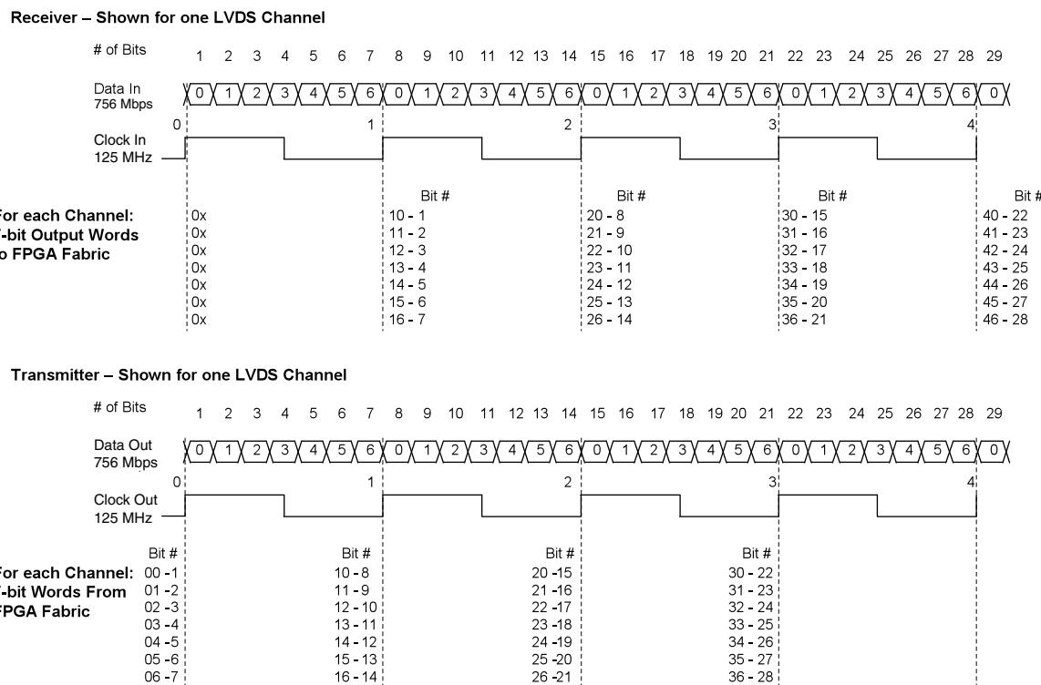
**Figure 3-10. Receiver GDDR71\_RX. Waveforms**
