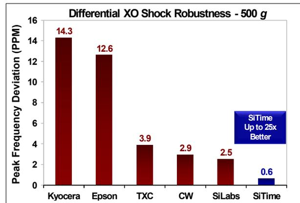
Figure 6. Shock Robustness<sup>[6]</sup>
