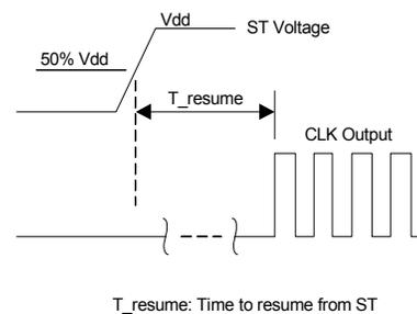
Figure 4. Standby Resume Timing (ST Mode Only)
