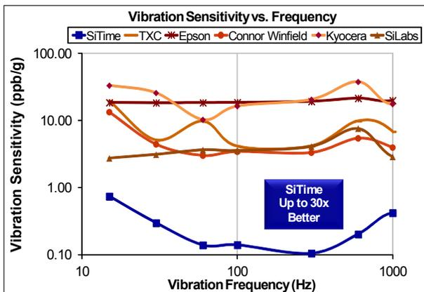
Figure 5. Vibration Robustness<sup>[5]</sup>
