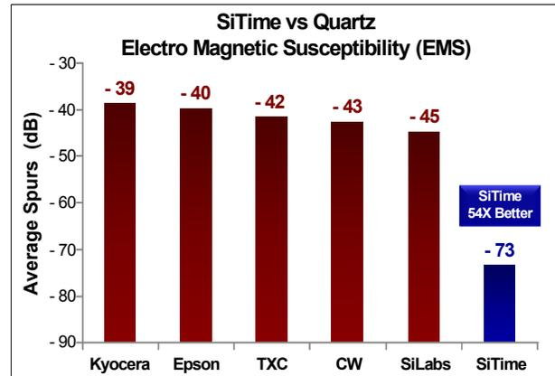
Figure 3. Electro Magnetic Susceptibility (EMS)<sup>[3]</sup>
