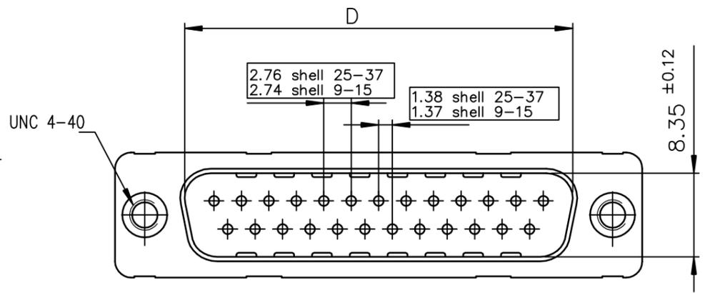
PC board drilling dimensions(after plating)
