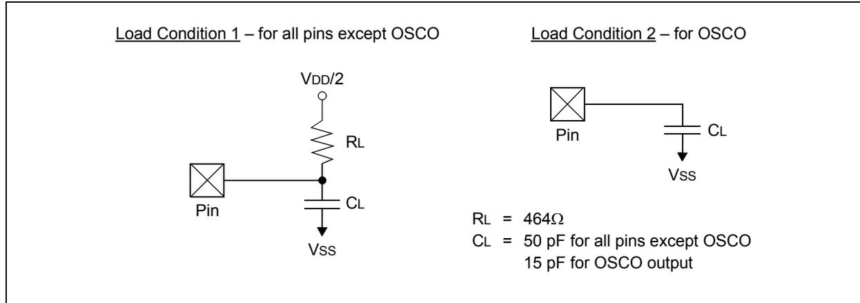
**TABLE 33-17: CAPACITIVE LOADING REQUIREMENTS ON OUTPUT PINS**
