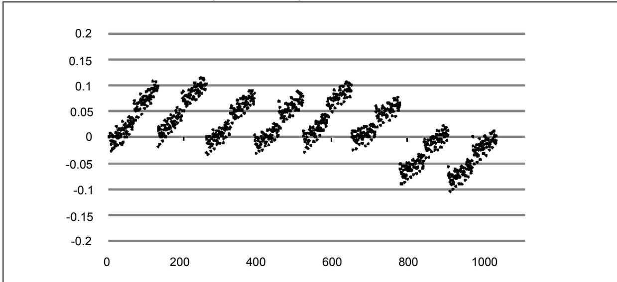
FIGURE 33-6: DNL vs. CODE (10-BIT MODE)
