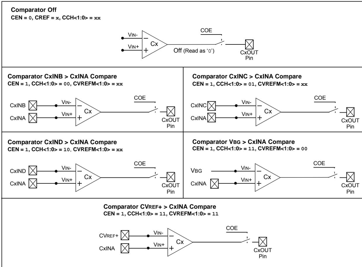
**FIGURE 26-3: INDIVIDUAL COMPARATOR CONFIGURATIONS WHEN CREF = 1 AND CVREFP = 0**
