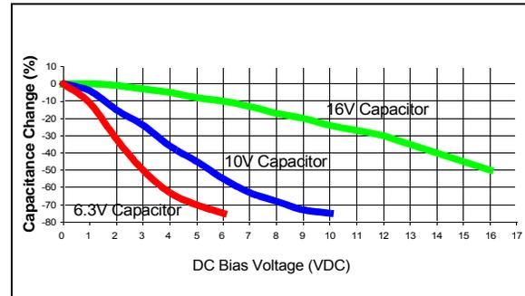
When selecting a ceramic capacitor to be used with the internal voltage regulator, it is suggested to select a high-voltage rating so that the operating voltage is a small percentage of the maximum rated capacitor voltage. For example, choose a ceramic capacitor rated at a minimum of 16V for the 1.8V core voltage. Suggested capacitors are shown in [Table 2-1](#).
