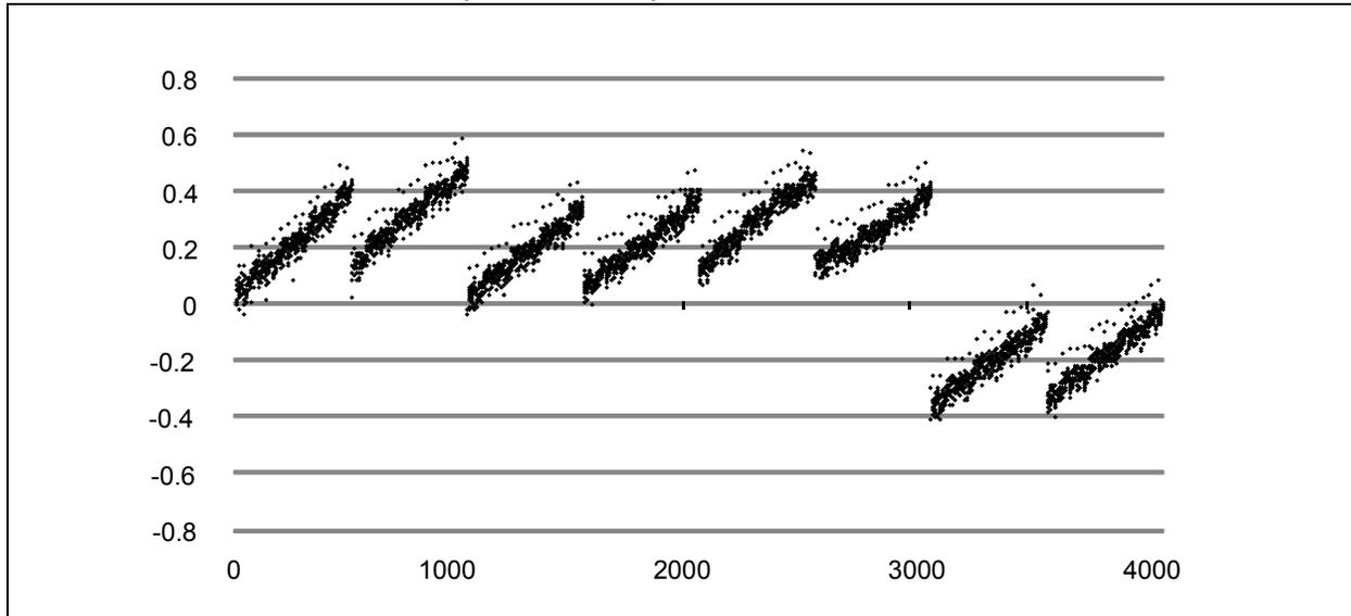
**FIGURE 33-8: DNL vs. CODE (12-BIT MODE)<sup>(1)</sup>**
