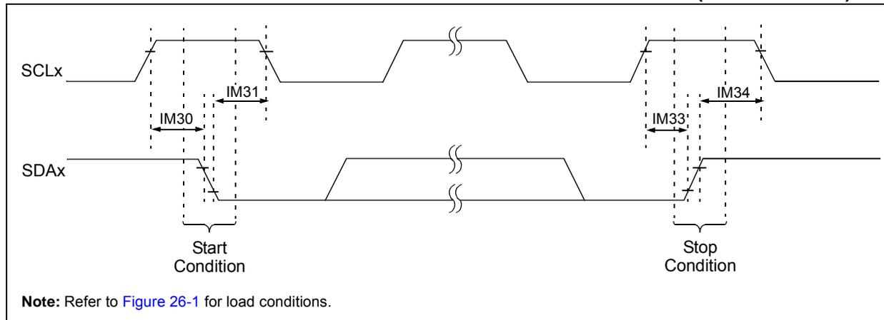
**FIGURE 26-23: I2Cx BUS DATA TIMING CHARACTERISTICS (MASTER MODE)**
