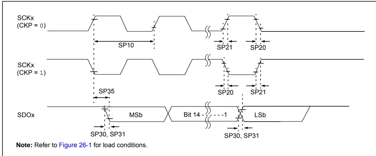
**FIGURE 26-15: SPIx MASTER MODE (HALF-DUPLEX, TRANSMIT ONLY CKE = 1) TIMING CHARACTERISTICS**
