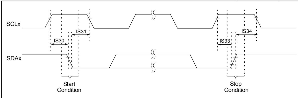
**FIGURE 26-25: I2Cx BUS DATA TIMING CHARACTERISTICS (SLAVE MODE)**
