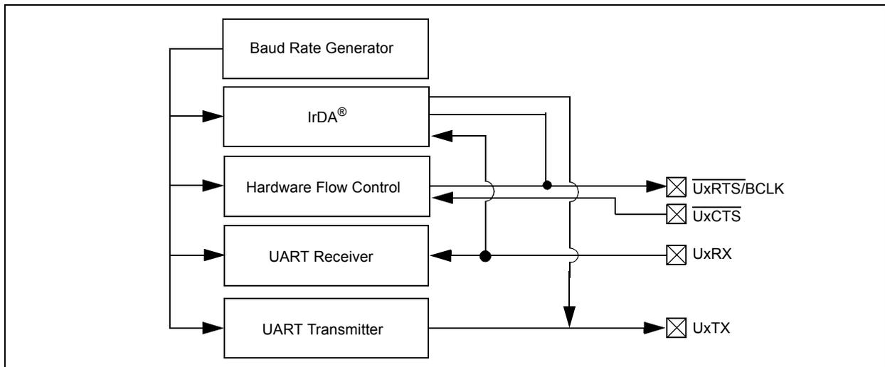
**Note 1:** Both UART1 and UART2 can trigger a DMA data transfer. If U1TX, U1RX, U2TX or U2RX is selected as a DMA IRQ source, a DMA transfer occurs when the U1TXIF, U1RXIF, U2TXIF or U2RXIF bit gets set as a result of a UART1 or UART2 transmission or reception.
