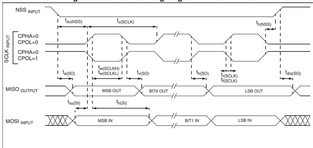
Figure 31. SPI slave timing diagram with CPHA = 1
