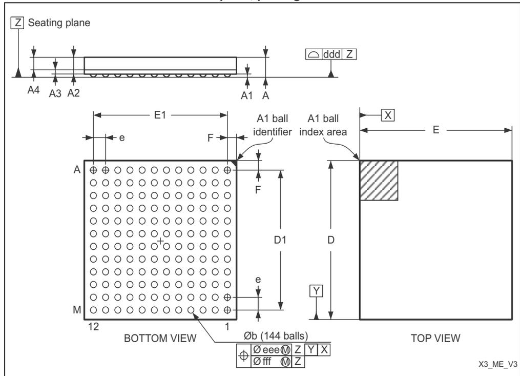
Table 52.LFBGA144 – 144-ball low profile fine pitch ball grid array, 10 x 10 mm, 0.8 mm pitch, package mechanical data
