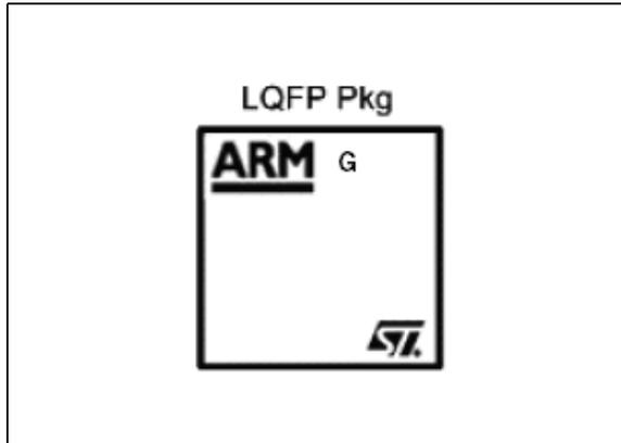
Figure 35. Device marking for revision G
