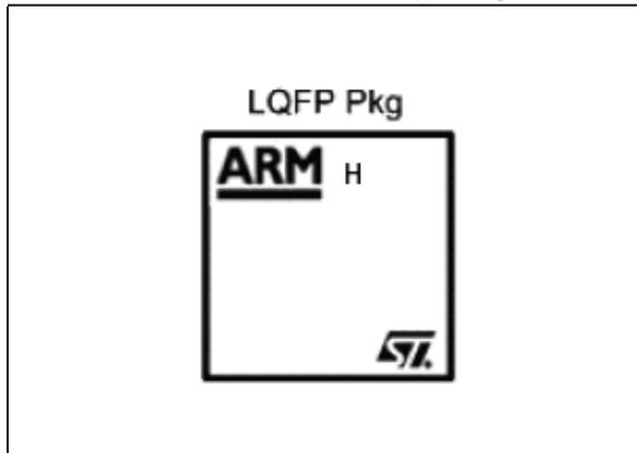
Figure 37. Device marking for revision H
