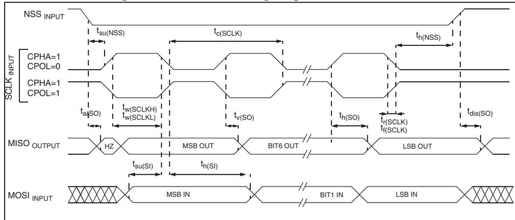
Figure 32. SPI master timing diagram
