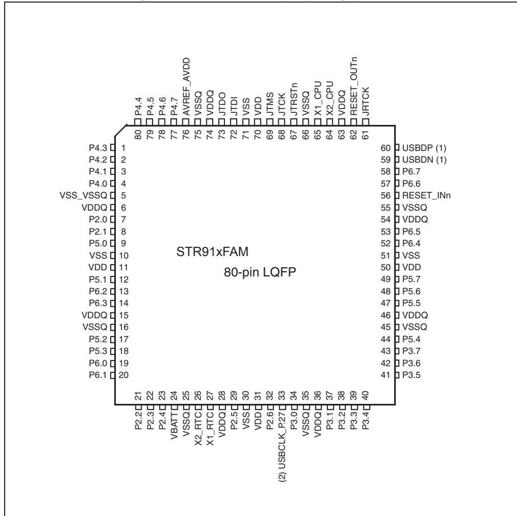
1. NU (Not Used) on STR910FAM devices. Pin 59 is not connected, pin 60 must be pulled up by a 1.5Kohm resistor to VDDQ.
