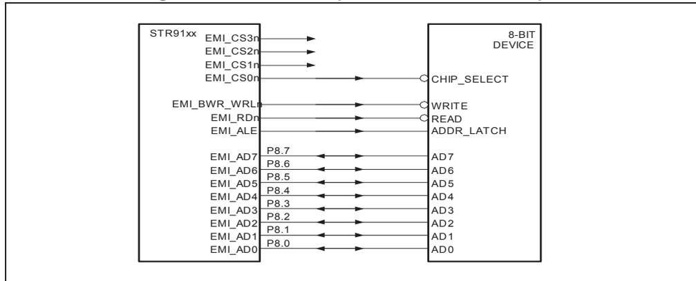
Figure 6. EMI 8-bit non-multiplexed connection example
