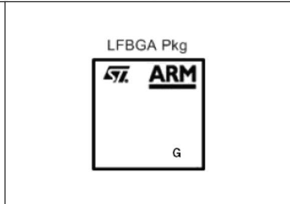
Figure 36. Device marking for revision H
