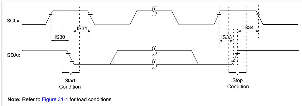
**FIGURE 31-17: I2Cx BUS DATA TIMING CHARACTERISTICS (SLAVE MODE)**
