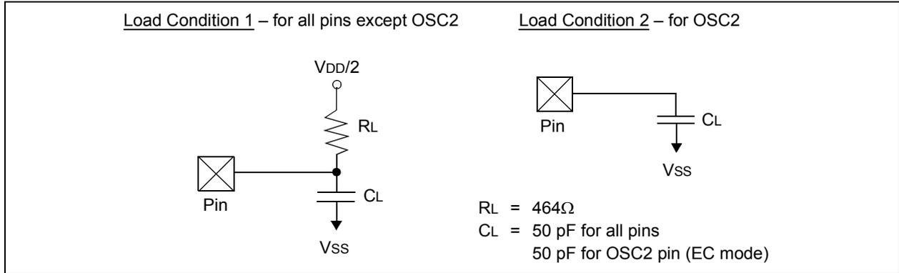
**TABLE 31-16: CAPACITIVE LOADING REQUIREMENTS ON OUTPUT PINS**
