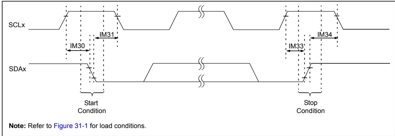
**FIGURE 31-15: I2Cx BUS DATA TIMING CHARACTERISTICS (MASTER MODE)**
