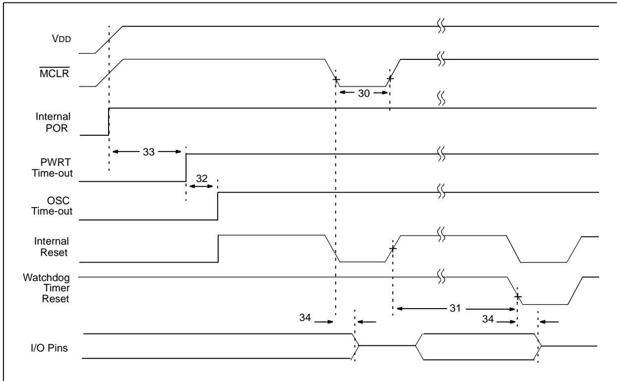
**TABLE 9-4: RESET, WATCHDOG TIMER, OSCILLATOR START-UP TIMER AND POWER-UP TIMER REQUIREMENTS**
