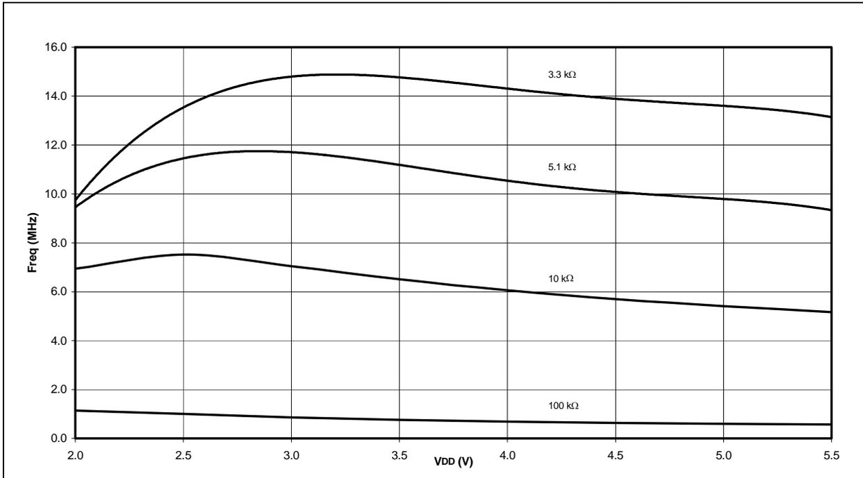
**FIGURE 10-8: AVERAGE  $F_{osc}$  vs.  $V_{DD}$  FOR R (RC MODE,  $C = 100\text{ pF}$ ,  $25^\circ\text{C}$ )**
