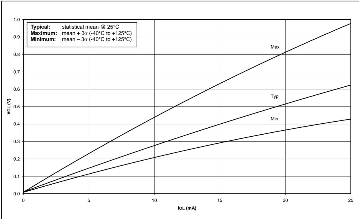
**FIGURE 10-16: TYPICAL, MINIMUM AND MAXIMUM  $V_{OL}$  vs.  $I_{OL}$  ( $V_{DD} = 3V$ ,  $-40^{\circ}C$  TO  $+125^{\circ}C$ )**
