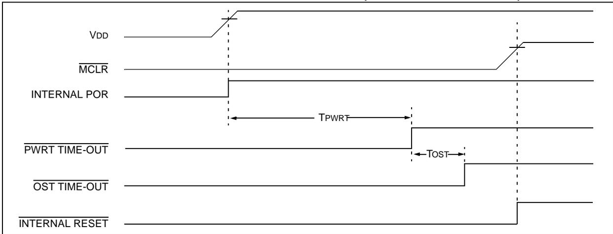
**FIGURE 6-8: TIME-OUT SEQUENCE ON POWER-UP ( $\overline{\text{MCLR}}$  TIED TO  $V_{\text{DD}}$ ): FAST  $V_{\text{DD}}$  RISE TIME**
