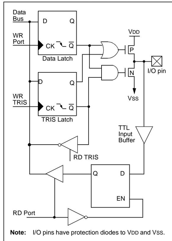
**FIGURE 4-2: BLOCK DIAGRAM OF PIN RA4**
