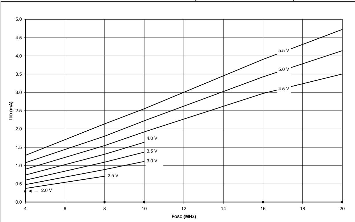
**FIGURE 10-3: TYPICAL  $I_{DD}$  vs.  $F_{osc}$  OVER  $V_{DD}$  (XT MODE, 25°C)**
