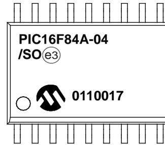
20-Lead SSOP (5.30 mm)
