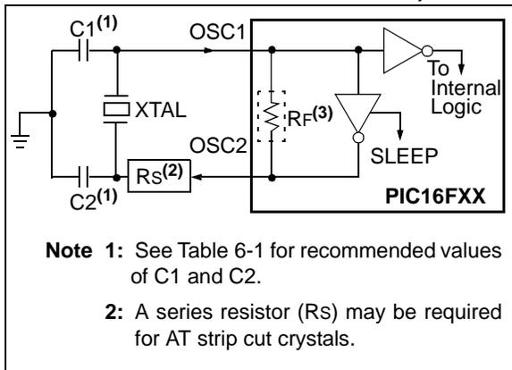
The PIC16F84A oscillator design requires the use of a parallel cut crystal. Use of a series cut crystal may give a frequency out of the crystal manufacturers specifications. When in XT, LP, or HS modes, the device can have an external clock source to drive the OSC1/CLKIN pin (Figure 6-2).
