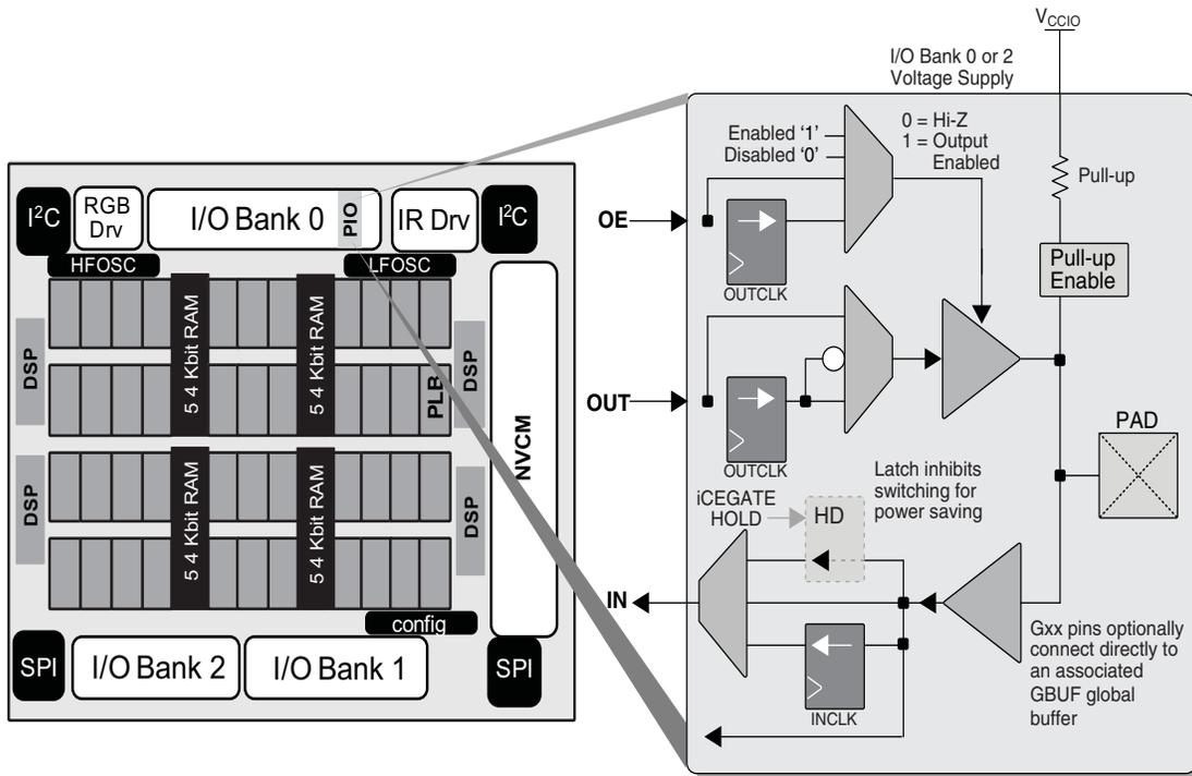
The PIO contains three blocks: an input register block, output register block iCEGate™ and tri-state register block. To save power, the optional iCEGate™ latch can selectively freeze the state of individual, non-registered inputs within an I/O bank. Note that the freeze signal is common to the bank. These blocks can operate in a variety of modes along with the necessary clock and selection logic.
