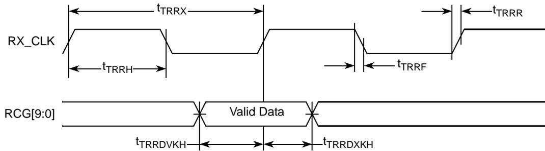
Figure 16. TBI Single-Clock Mode Receive AC Timing Diagram
