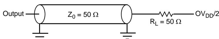
Figure 33. I<sup>2</sup>C AC Test Load
