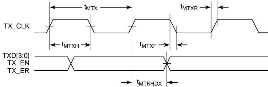
Figure 11. MII Transmit AC Timing Diagram
