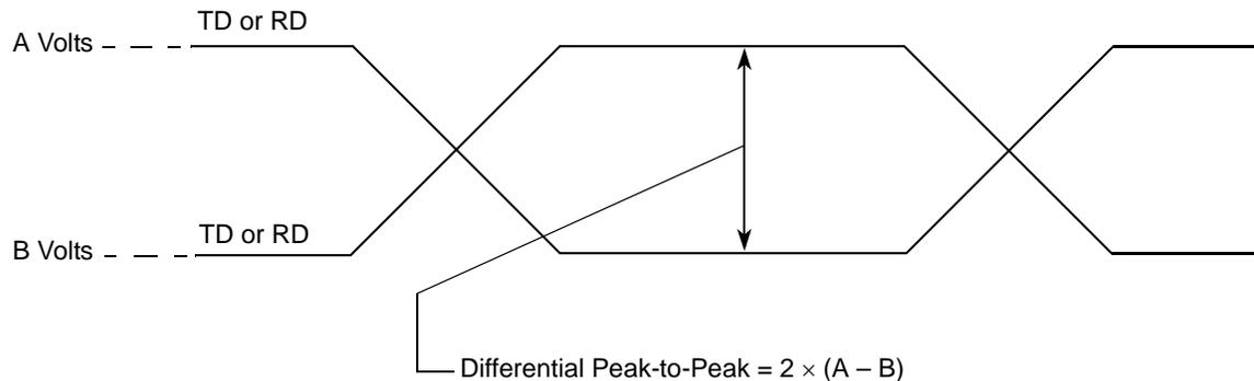
**Figure 51. Differential Peak-Peak Voltage of Transmitter or Receiver**
