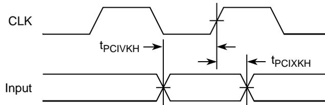
Figure 36. PCI/PCI-X Input AC Timing Measurement Conditions
