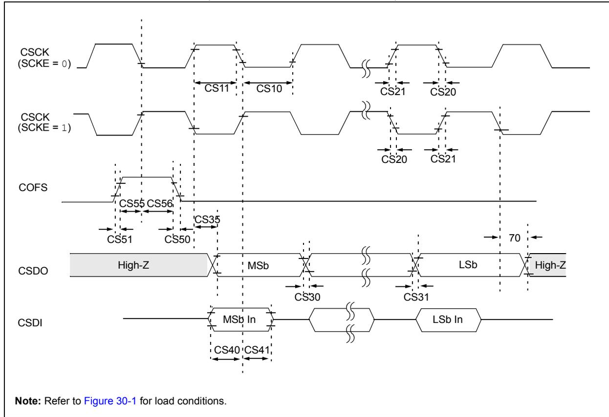
TABLE 30-38: DCI MODULE (MULTI-CHANNEL, I<sup>2</sup>S MODES) TIMING REQUIREMENTS
