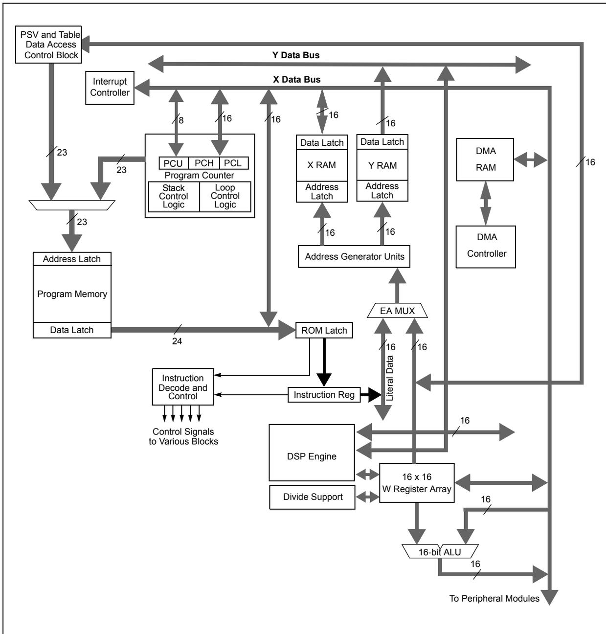
FIGURE 3-2: dsPIC33FJ32GP302/304, dsPIC33FJ64GPX02/X04, AND dsPIC33FJ128GPX02/X04 PROGRAMMER'S MODEL
