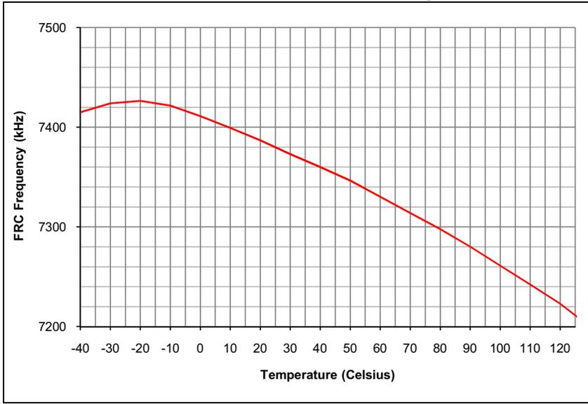
**FIGURE 32-14: TYPICAL LPRC FREQUENCY @ VDD = 3.3V**
