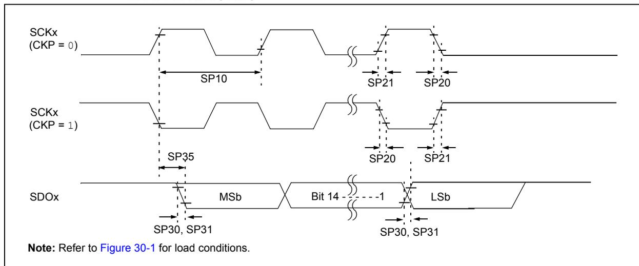
FIGURE 30-10: SPIx MASTER MODE (HALF-DUPLEX, TRANSMIT ONLY CKE = 1) TIMING CHARACTERISTICS
