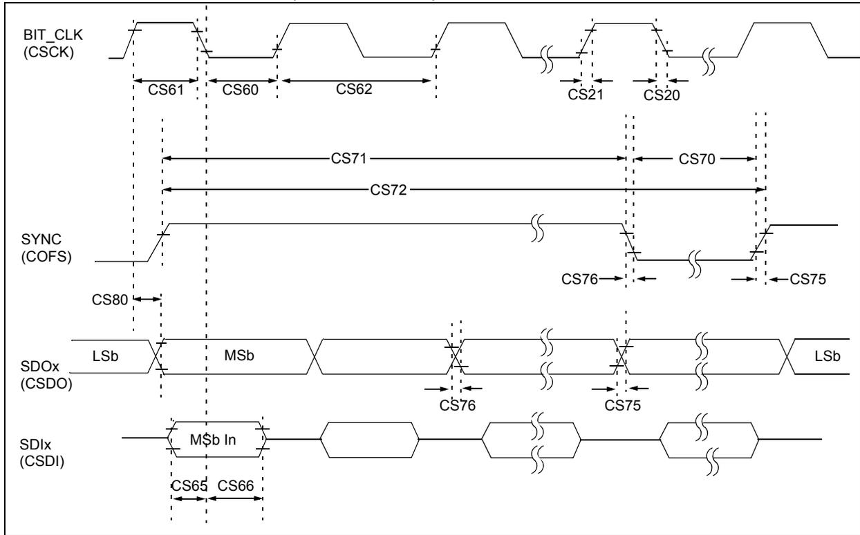
TABLE 30-39: DCI MODULE (AC-LINK MODE) TIMING REQUIREMENTS
