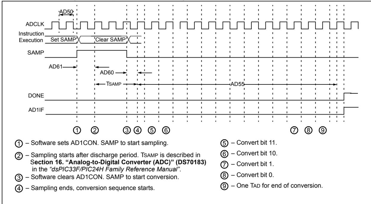
TABLE 30-44: ADC CONVERSION (12-BIT MODE) TIMING REQUIREMENTS
