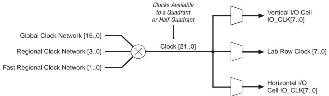
IOE clocks have horizontal and vertical block regions that are clocked by eight I/O clock signals chosen from the 22 quadrant or half-quadrant clock resources. [Figures 2–47](#) and [2–48](#) show the quadrant and half-quadrant relationship to the I/O clock regions, respectively. The vertical regions (column pins) have less clock delay than the horizontal regions (row pins).
