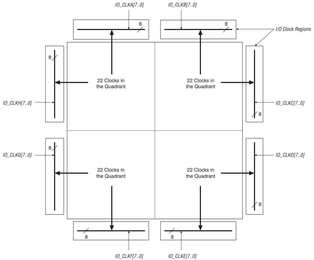
**Figure 2–48. EP1S30, EP1S40, EP1S60, EP1S80 Device I/O Clock Groups**
