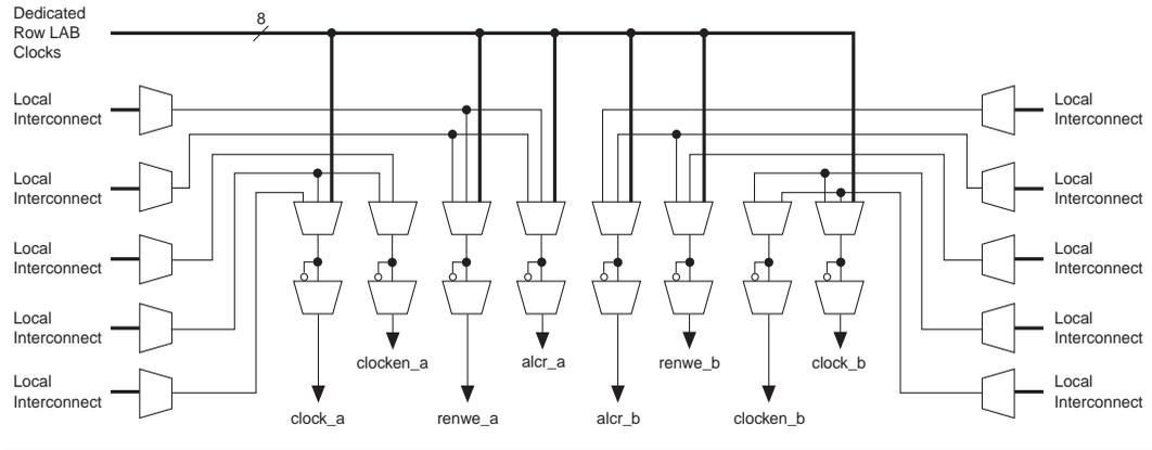
**Figure 2-18. M4K RAM Block LAB Row Interface**
