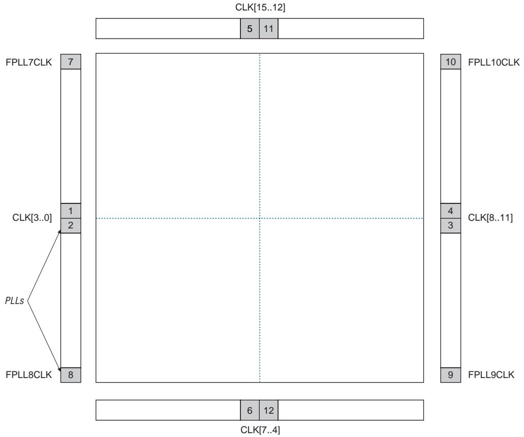
Figure 2–50 shows the global and regional clocking from the PLL outputs and the CLK pins.
