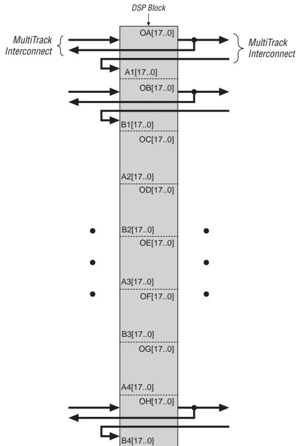
Figure 2–41. DSP Block Interface to Interconnect
