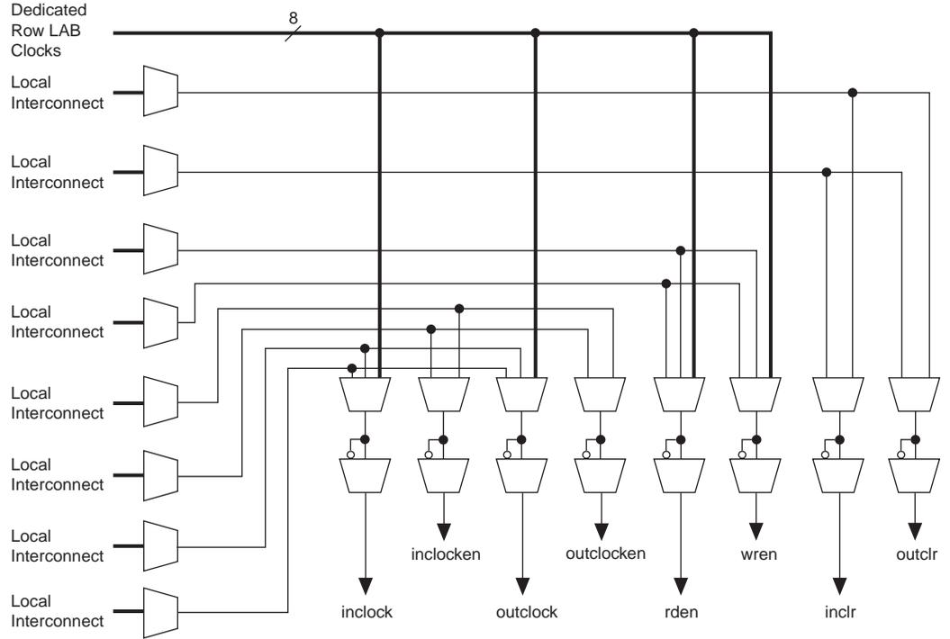
Figure 2–16. M512 RAM Block LAB Row Interface
