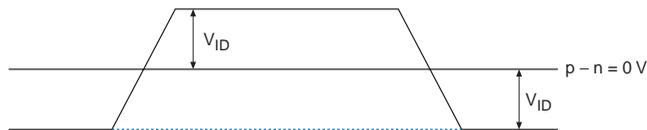
**Figure 4–2. Transmitter Output Waveforms for Differential I/O Standards**
