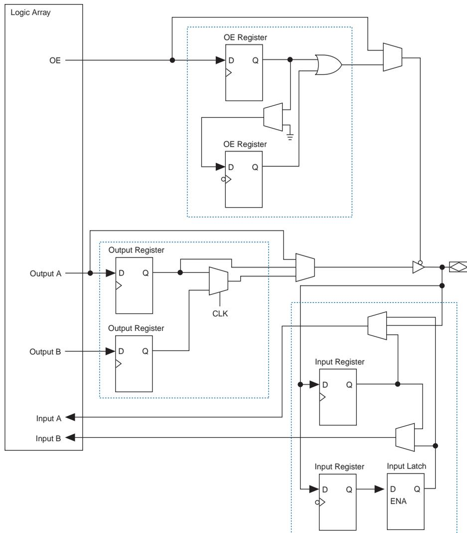
The IOEs are located in I/O blocks around the periphery of the Stratix device. There are up to four IOEs per row I/O block and six IOEs per column I/O block. The row I/O blocks drive row, column, or direct link interconnects. The column I/O blocks drive column interconnects.
