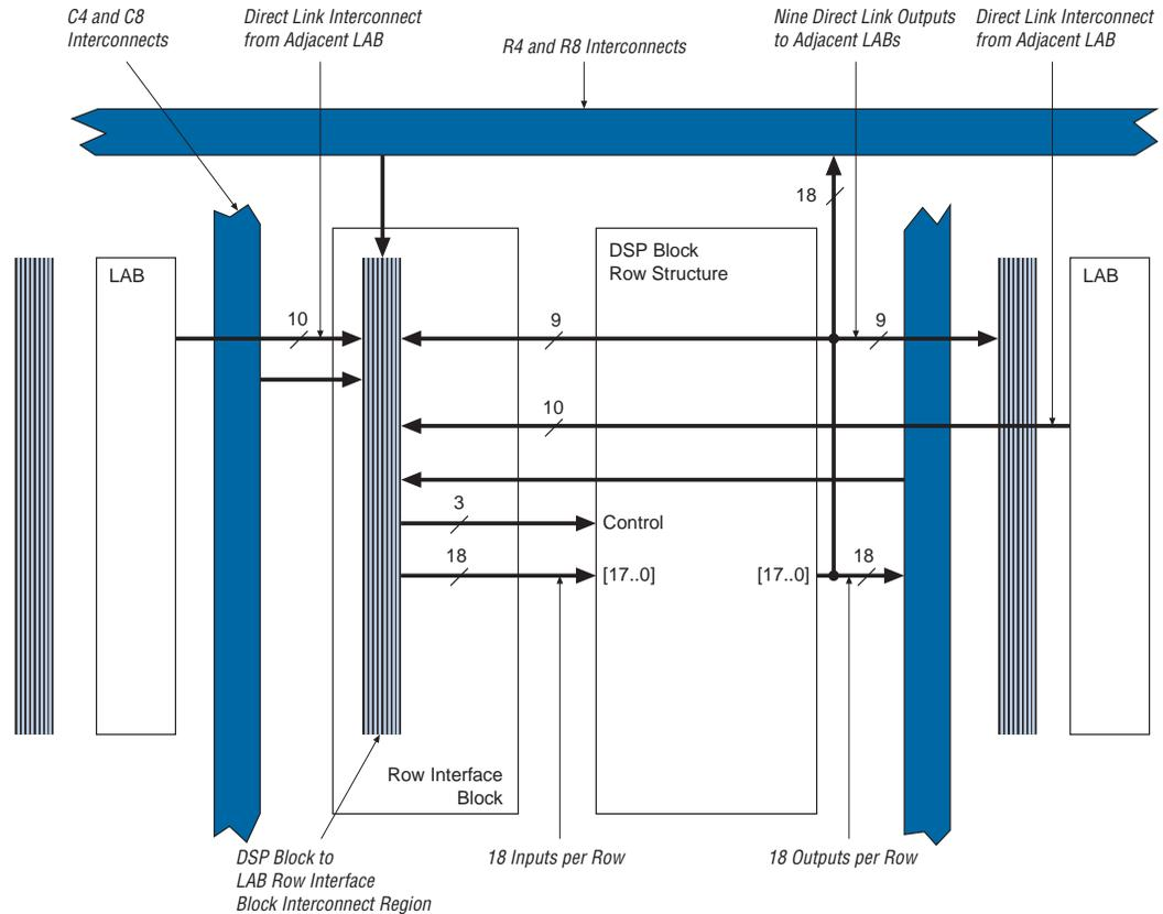
A bus of 18 control signals feeds the entire DSP block. These signals include `clock[0..3]` clocks, `aclr[0..3]` asynchronous clears, `ena[1..4]` clock enables, `signa`, `signb` signed/unsigned control signals, `addnsub1` and `addnsub3` addition and subtraction control signals, and `accum_sload[0..1]` accumulator synchronous loads. The
