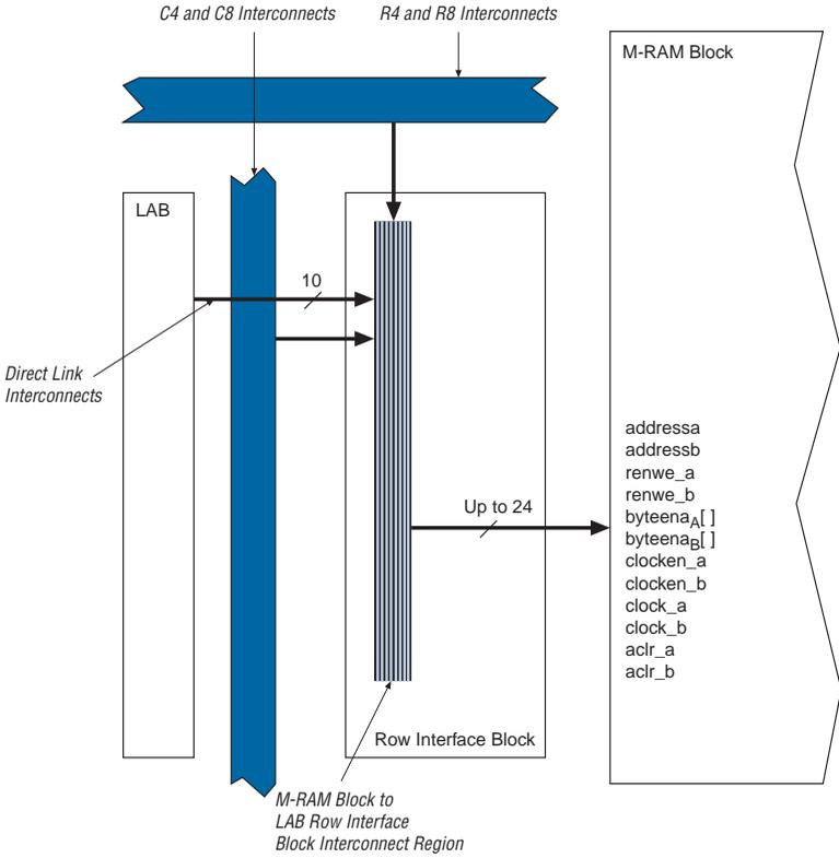
**Figure 2-23. M-RAM Column Unit Interface to Interconnect**
