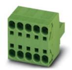
PCB connector, nominal current: 41 A, rated voltage (III/2): 1000 V, number of positions: 3, pitch: 7.62 mm, connection method: Push-in spring connection, color: green, contact surface: Tin
