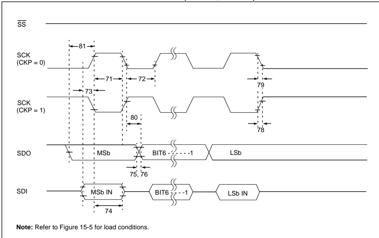
**FIGURE 15-15: SPI SLAVE MODE TIMING (CKE = 0)**
