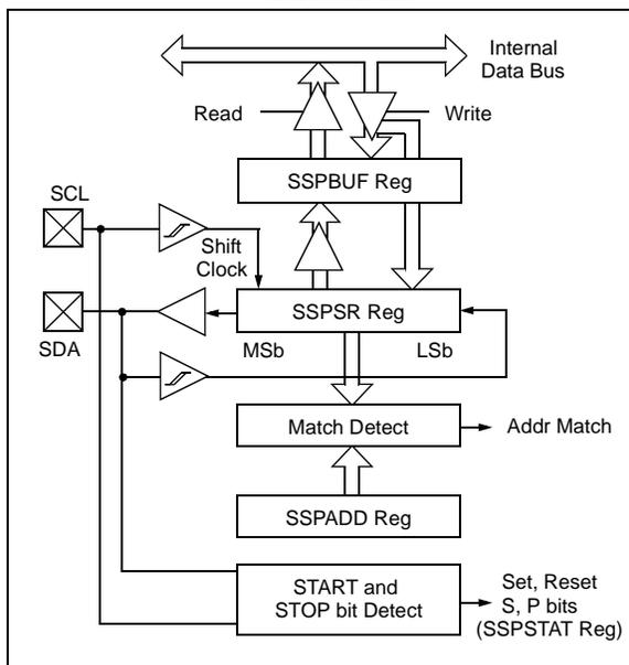
Two pins are used for data transfer. These are the SCL pin, which is the clock, and the SDA pin, which is the data. The SDA and SCL pins are automatically configured when the I<sup>2</sup>C mode is enabled. The SSP module functions are enabled by setting SSP Enable bit SSPEN (SSPCON<5>).
