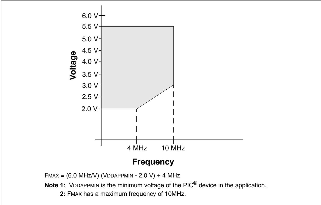
**FIGURE 15-3: PIC16F87X-04 VOLTAGE-FREQUENCY GRAPH (ALL TEMPERATURE RANGES)**
