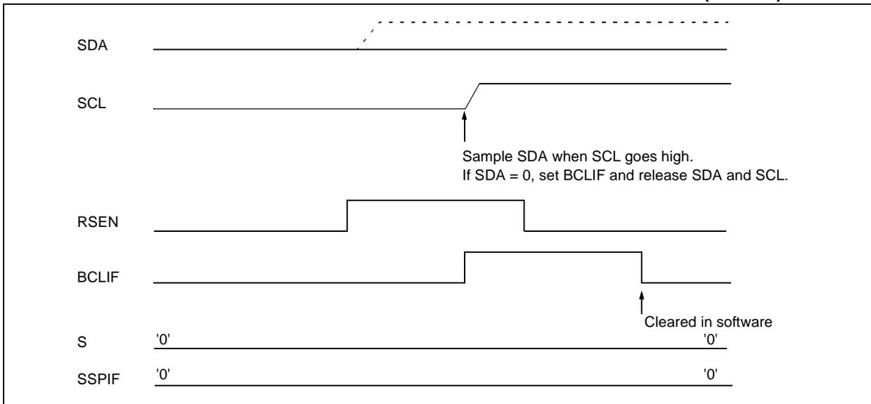
**FIGURE 9-24: BUS COLLISION DURING REPEATED START CONDITION (CASE 2)**
