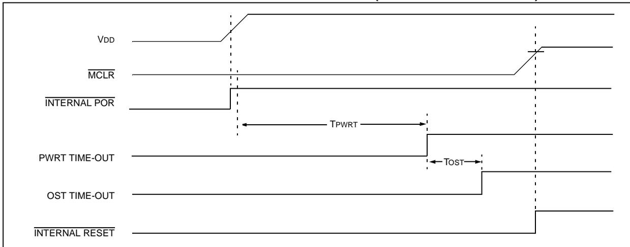
**FIGURE 12-8: SLOW RISE TIME ( $\overline{\text{MCLR}}$  TIED TO  $V_{DD}$ )**
