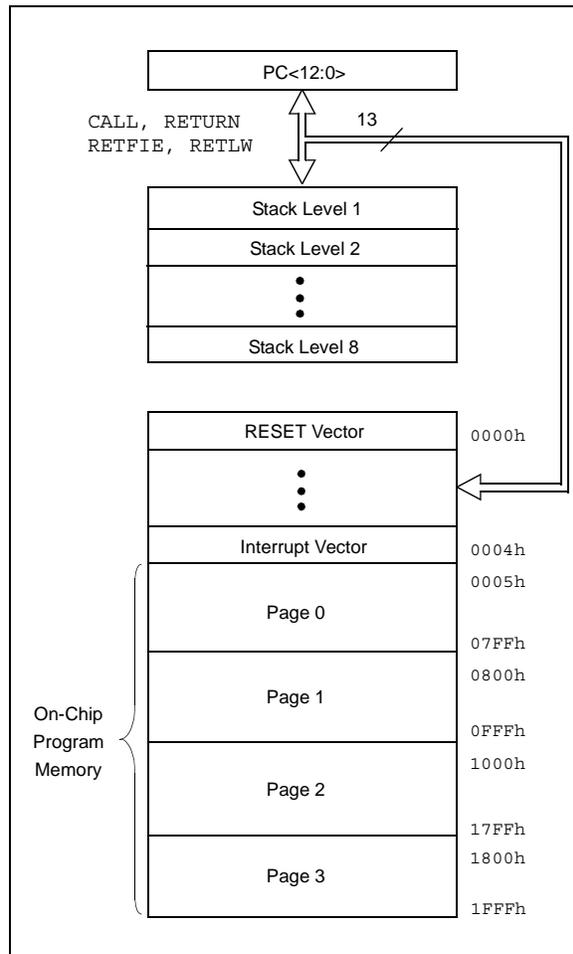
**FIGURE 2-2: PIC16F874/873 PROGRAM MEMORY MAP AND STACK**
