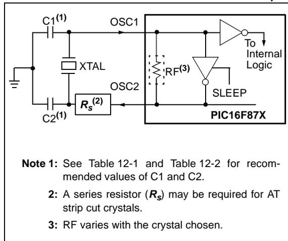
**FIGURE 12-2: EXTERNAL CLOCK INPUT OPERATION (HS, XT OR LP OSC CONFIGURATION)**
