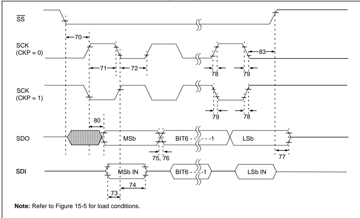
**FIGURE 15-16: SPI SLAVE MODE TIMING (CKE = 1)**
