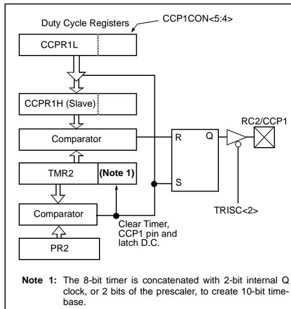
A PWM output (Figure 8-4) has a time-base (period) and a time that the output stays high (duty cycle). The frequency of the PWM is the inverse of the period (1/period).
