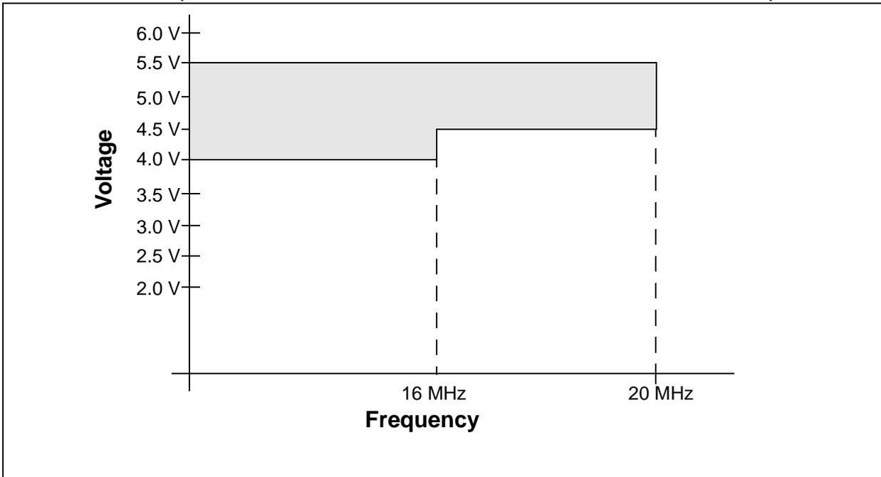
**FIGURE 15-2: PIC16LF87X-04 VOLTAGE-FREQUENCY GRAPH
