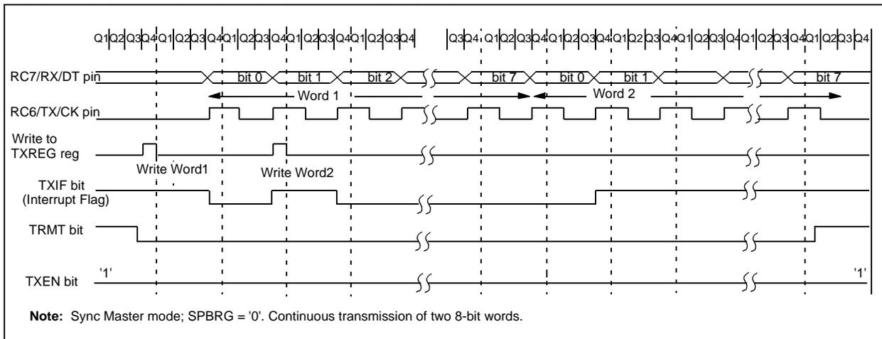
**FIGURE 10-10: SYNCHRONOUS TRANSMISSION (THROUGH TXEN)**
