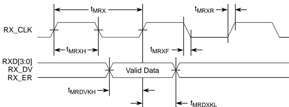
Figure 14. MII Receive AC Timing Diagram
