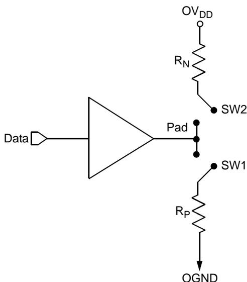
Figure 64. Driver Impedance Measurement
