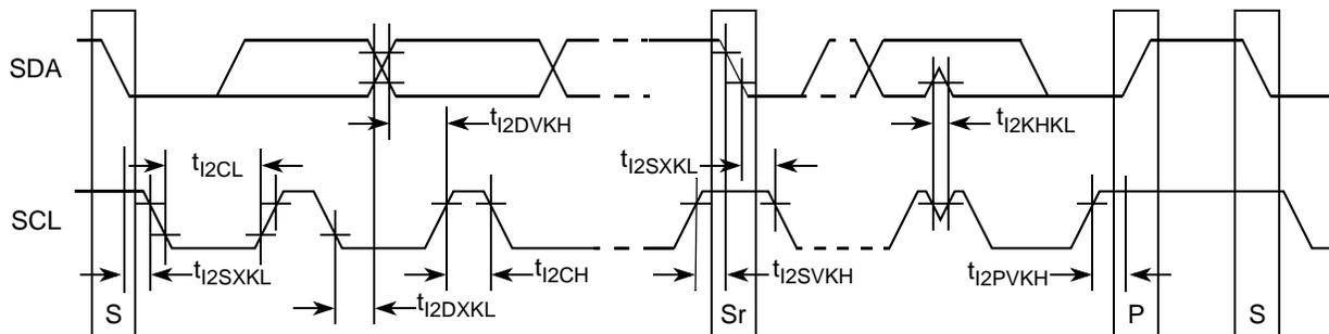
**Figure 41. I<sup>2</sup>C Bus AC Timing Diagram**
