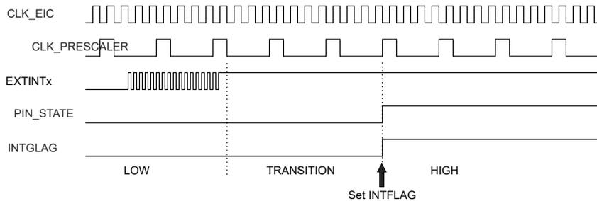
In the synchronous edge detection mode, the EIC clock is required. The synchronous edge detection mode can be used in Idle and Standby sleep modes.
