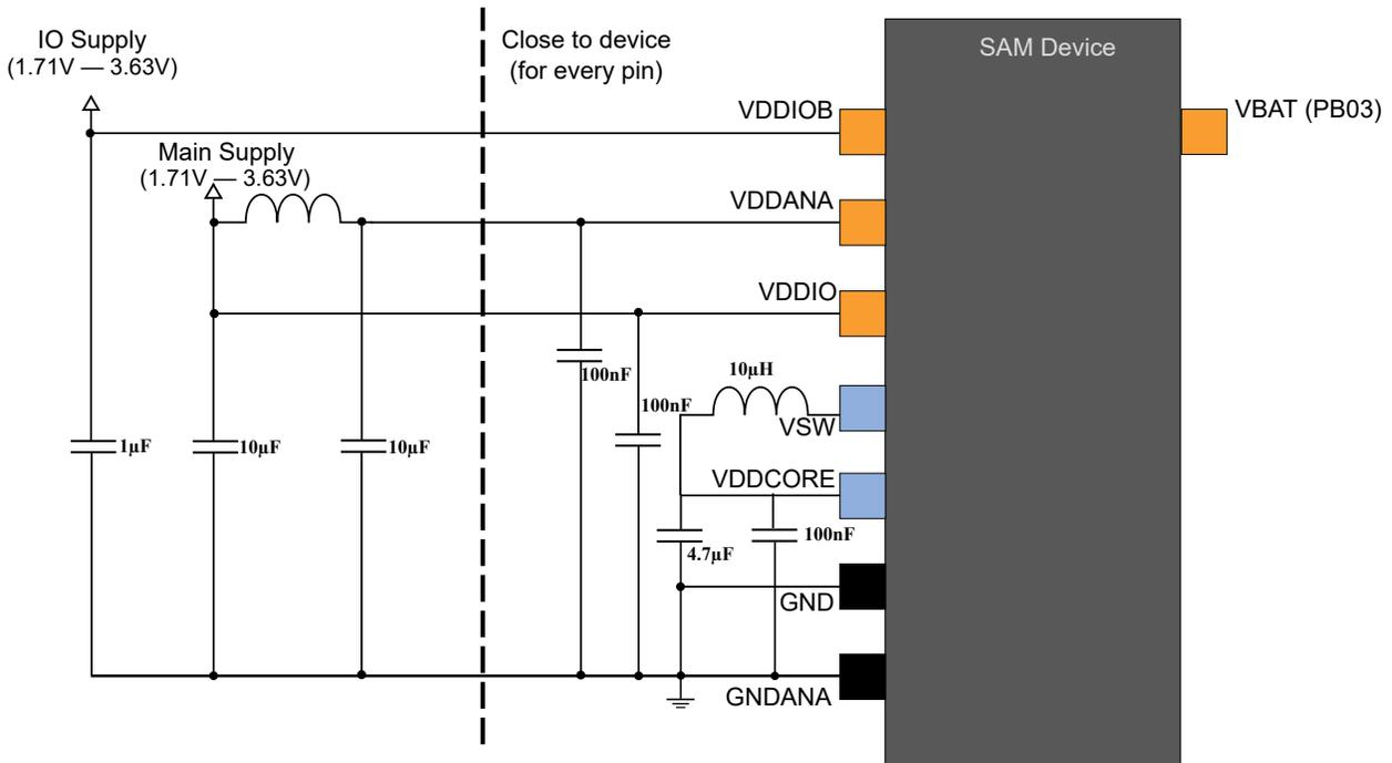
**Figure 56-2. Power Supply Connection for Linear Mode Only**
