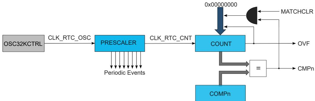
Figure 21-2. RTC Block Diagram (Mode 1 — 16-Bit Counter)
