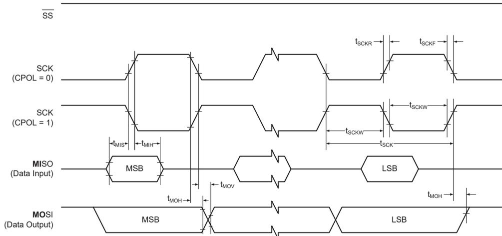
**Figure 54-10. SPI Timing Requirements in Slave Mode**
