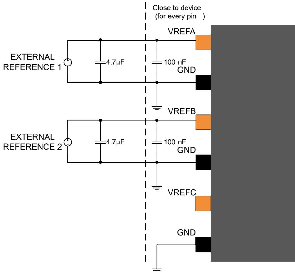
**Figure 56-6. External Analog Reference Schematic With One Reference**
