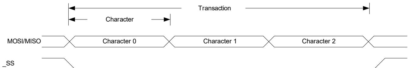
The SPI master must pull the slave select line ( $\overline{SS}$ ) of the desired slave low to initiate a transaction. The master and slave prepare data to send via their respective shift registers, and the master generates the serial clock on the SCK line.
