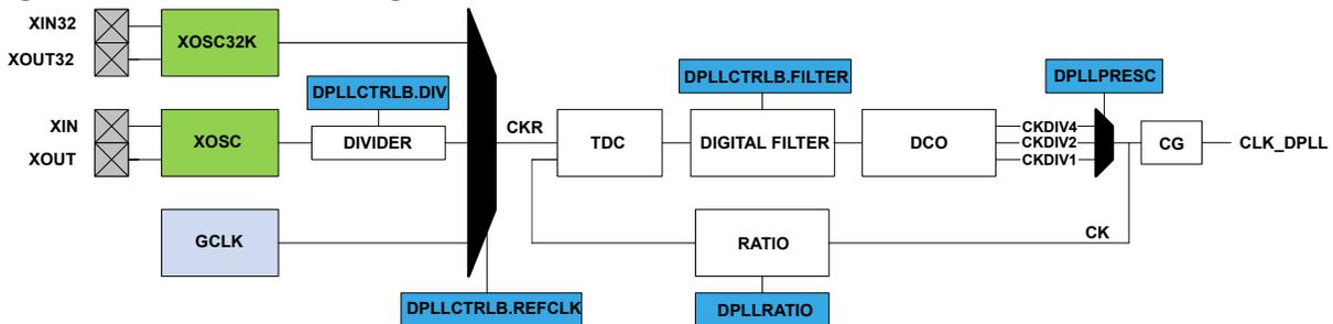
When the controller is disabled, the output clock is low. If the Loop Divider Ratio Fractional part bit field in the DPLL Ratio register (DPLL.RATIO.LDRFRAC) is zero, the DPLL works in Integer mode. Otherwise, the fractional mode is activated. Note that the fractional part has a negative impact on the jitter of the DPLL.
