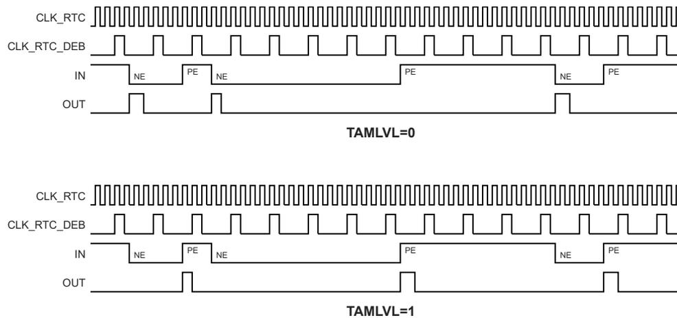
**Figure 21-7. Edge Detection with Synchronous Stability Debouncing**
