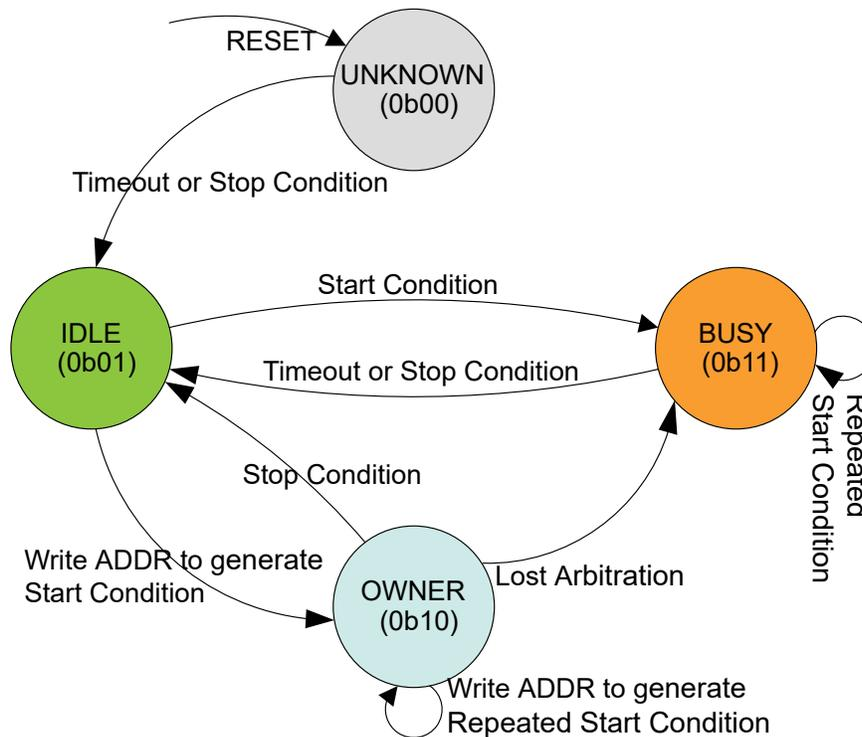
The bus state machine is active when the I<sup>2</sup>C master is enabled.
