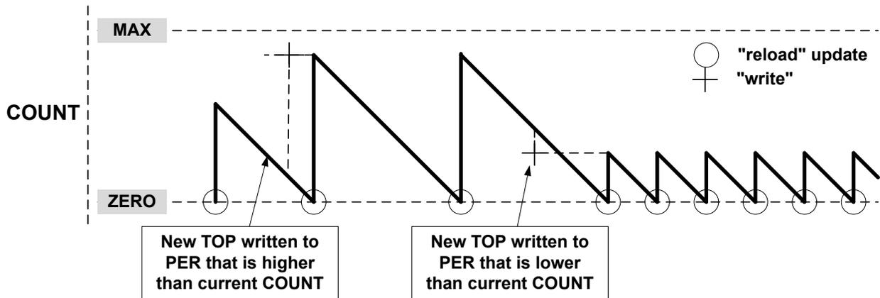
When double buffering is used, the buffer can be written at any time and the counter will still maintain correct operation. The period register is always updated on the update condition, as shown in [Figure 48-10](#). This prevents wraparound and the generation of odd waveforms.
