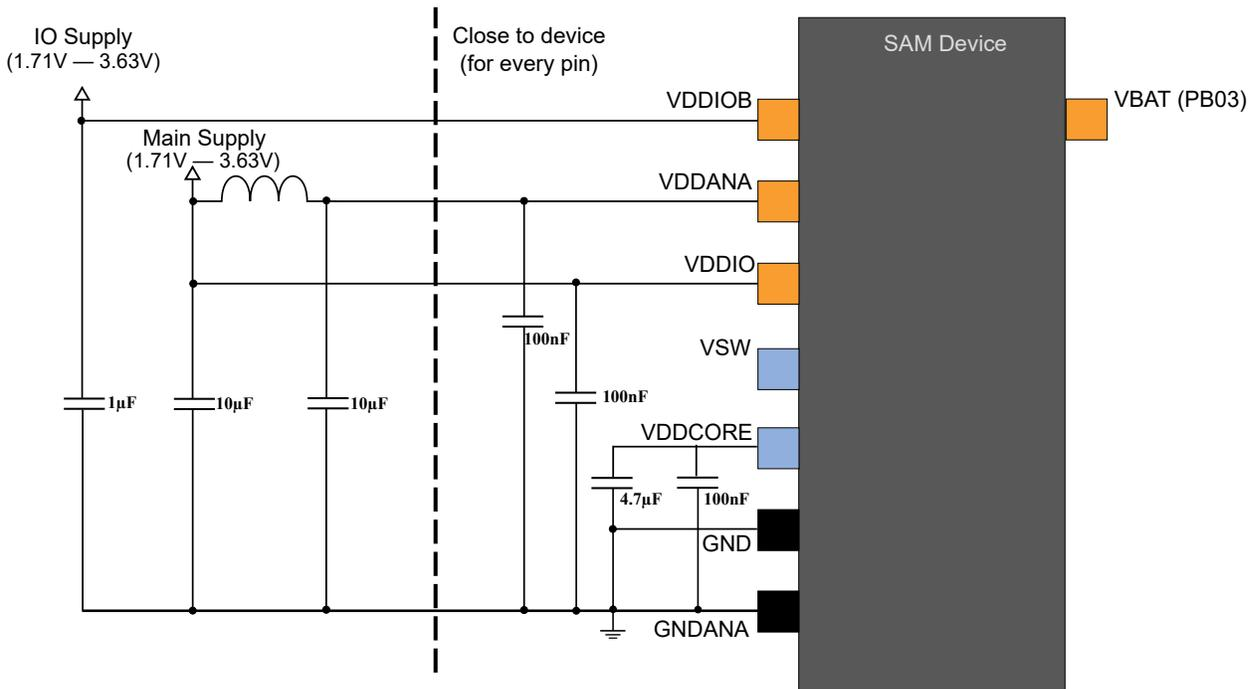
**Figure 56-3. Power Supply Connection for Battery Backup**
