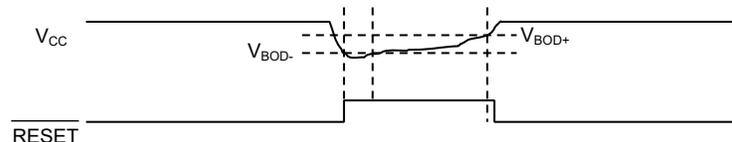
Enabling the BOD12 hysteresis by writing the Hysteresis bit in the BOD12 register (BOD12.HYST) to '1' will add hysteresis to the BOD12 threshold level.
