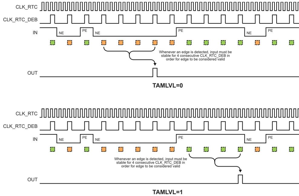
**Figure 21-8. Edge Detection with Asynchronous Stability Debouncing**
