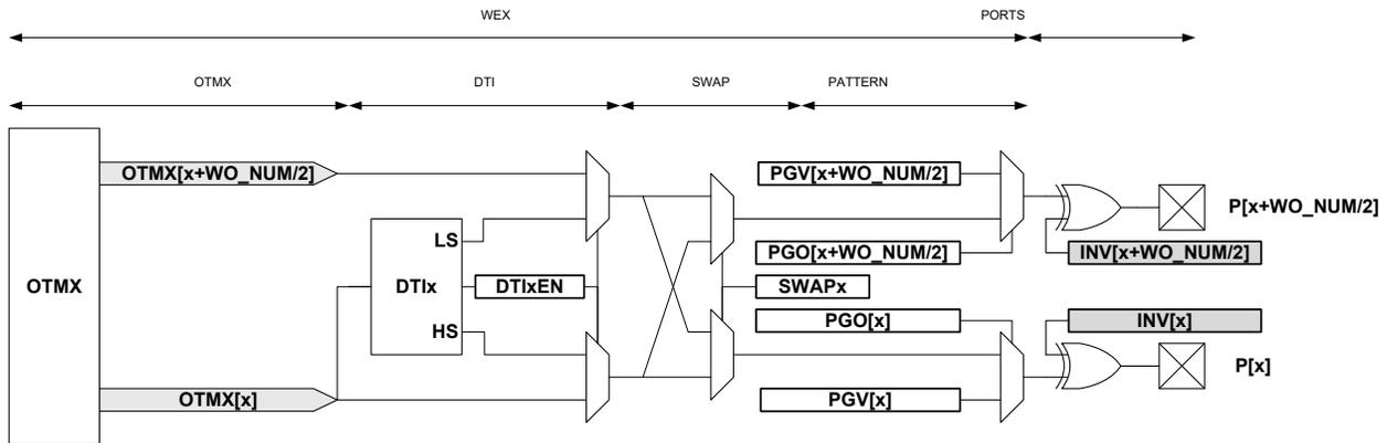
The output matrix (OTMX) unit distributes compare channels, according to the selectable configurations in [Table 49-4](#).
