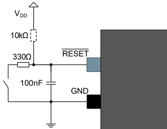
A pull-up resistor makes sure that the Reset does not go low and unintentionally causing a device Reset. An additional resistor has been added in series with the switch to safely discharge the filtering capacitor, i.e. preventing a current surge when shorting the filtering capacitor which again can cause a noise spike that can have a negative effect on the system.
