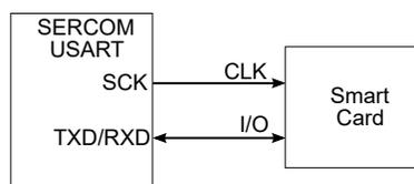
ISO 7816 characters are specified as 8 bits with even parity. The USART must be configured accordingly.
