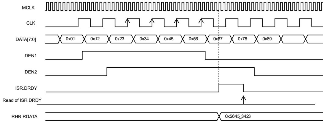
**Figure 52-4. PCC Waveforms (ISIZE=10\_BITS, DSIZE=2\_DATA, ALWAYS = 0, HALFS = 0, SCALE = 0)**
