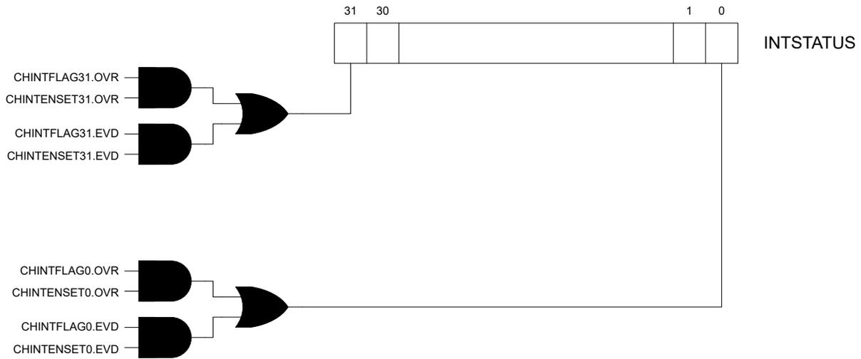
The Event System can arbitrate between all channels with pending interrupts. The arbiter can be configured to prioritize statically or dynamically the incoming events. The priority is evaluated each time a new channel has an interrupt pending, or an interrupt has been cleared. The Channel Pending Interrupt register (INTPEND) will provide the channel number with the highest interrupt priority, and the corresponding channel interrupt flags and status bits.
