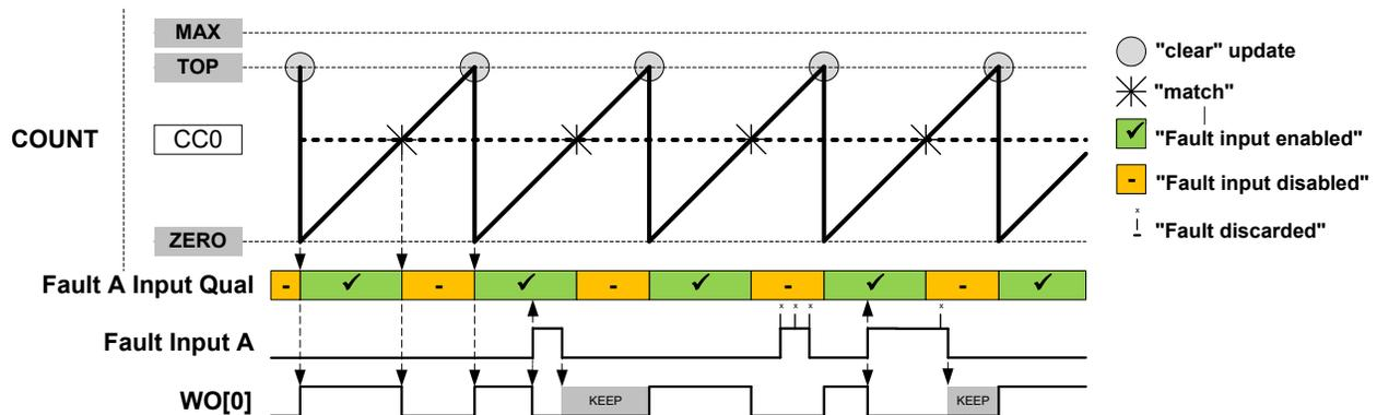
**Restart Action** This is enabled by writing the Fault n Restart bit in Recoverable Fault n Configuration register (FCTRLn.RESTART) to '1'. When enabled, the timer/counter will be restarted as soon as the corresponding fault condition is present. The ongoing cycle is stopped and the timer/counter starts a new cycle, see [Figure 49-26](#). In Ramp 1 mode, when the new cycle starts, the compare outputs will be clamped to inactive level as long as the fault condition is present.
