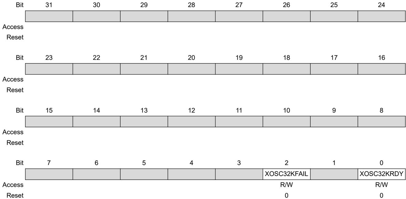
**Bit 2 – XOSC32KFAIL** XOSC32K Clock Failure Detector
