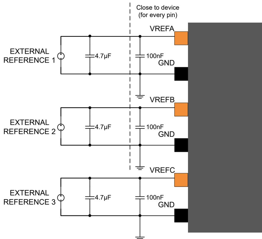
Figure 56-5. External Analog Reference Schematic With Two References
