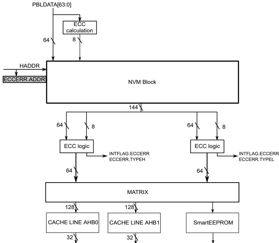
Note that the ECC correction is disabled when access is performed by the SmartEEPROM interface.
