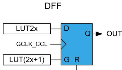
When the even LUT is disabled (`LUTCTRL0.ENABLE=0` / `LUTCTRL2.ENABLE=0`), the flip-flop is asynchronously cleared. The reset command (R) is kept enabled for one APB clock cycle. In all other cases, the flip-flop output (OUT) is refreshed on rising edge of the `GCLK_CCL`, as shown in [Table 41-2](#).
