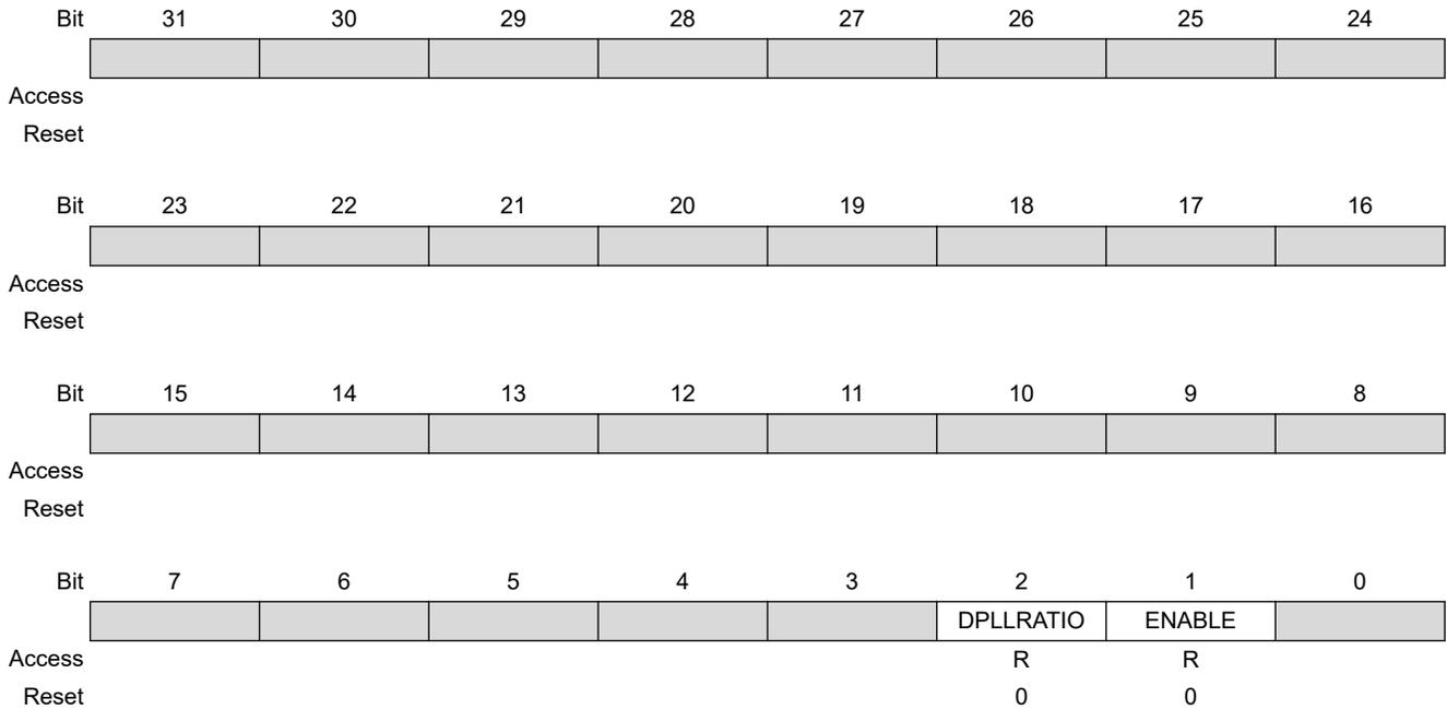
**Bit 2 – DPLL RATIO** DPLL Loop Divider Ratio Synchronization Status
