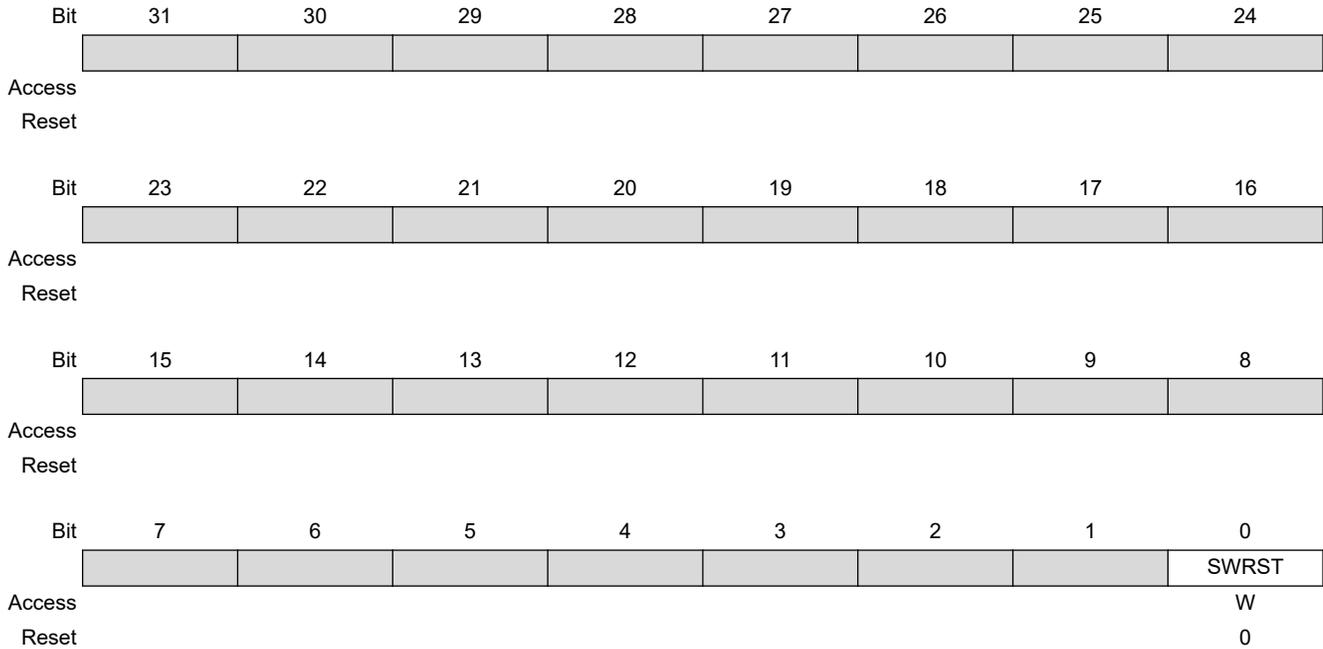
**Bit 0 – SWRST** Cache Controller Software Reset
