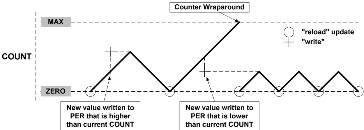
When double buffering is used, the buffer can be written at any time and the counter will still maintain correct operation. The period register is always updated on the update condition, as shown in [Figure 49-13](#). This prevents wraparound and the generation of odd waveforms.
