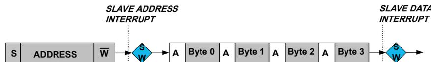
The LENGTH register can be written before the frame begins, or when the AMATCH interrupt is set. If the frame size is not LENGTH.LEN Bytes, the Length Error status bit (STATUS.LENERR) is raised. If LENGTH.LEN is not a multiple of 4 Bytes, the final INTFLAG.DRDY interrupt is raised when the last Byte is received for master reads. For master writes, the last data byte will be automatically NACKed. On address recognition, the internal length counter is reset in preparation for the incoming frame.
