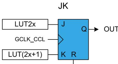
When the even LUT is disabled (`LUTCTRL0.ENABLE=0` / `LUTCTRL2.ENABLE=0`), the flip-flop is asynchronously cleared. The reset command (R) is kept enabled for one APB clock cycle. In all other cases, the flip-flop output (OUT) is refreshed on rising edge of the `GCLK_CCL`, as shown in [Table 41-3](#).
