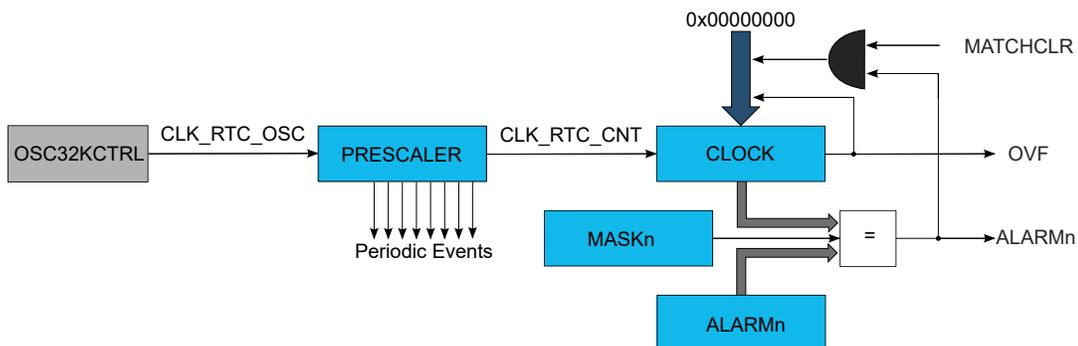
**Figure 21-4. RTC Block Diagram (Tamper Detection)**
