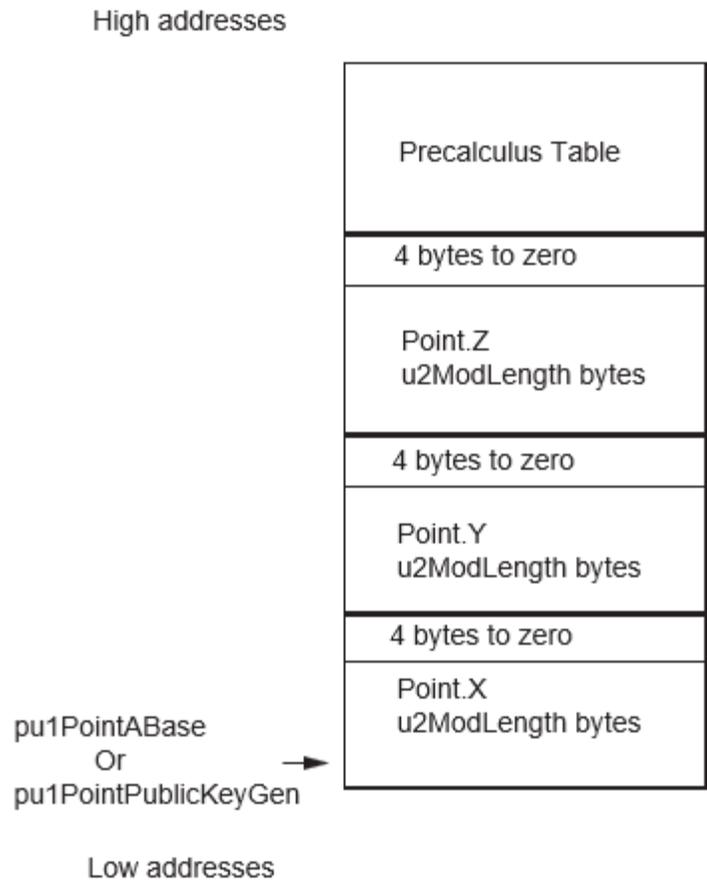
**Figure 43-13. PointSignature {pu1PointSignature,  $2 \cdot u2ScalarLength + 8$ }**
