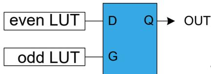
When the even LUT is disabled (LUTCTRL0.ENABLE=0 / LUTCTRL2.ENABLE=0), the latch output will be cleared. The G-input is forced enabled for one more APB clock cycle, and the D-input to zero. In all other cases, the latch output (OUT) is refreshed as shown in [Table 41-4](#).
