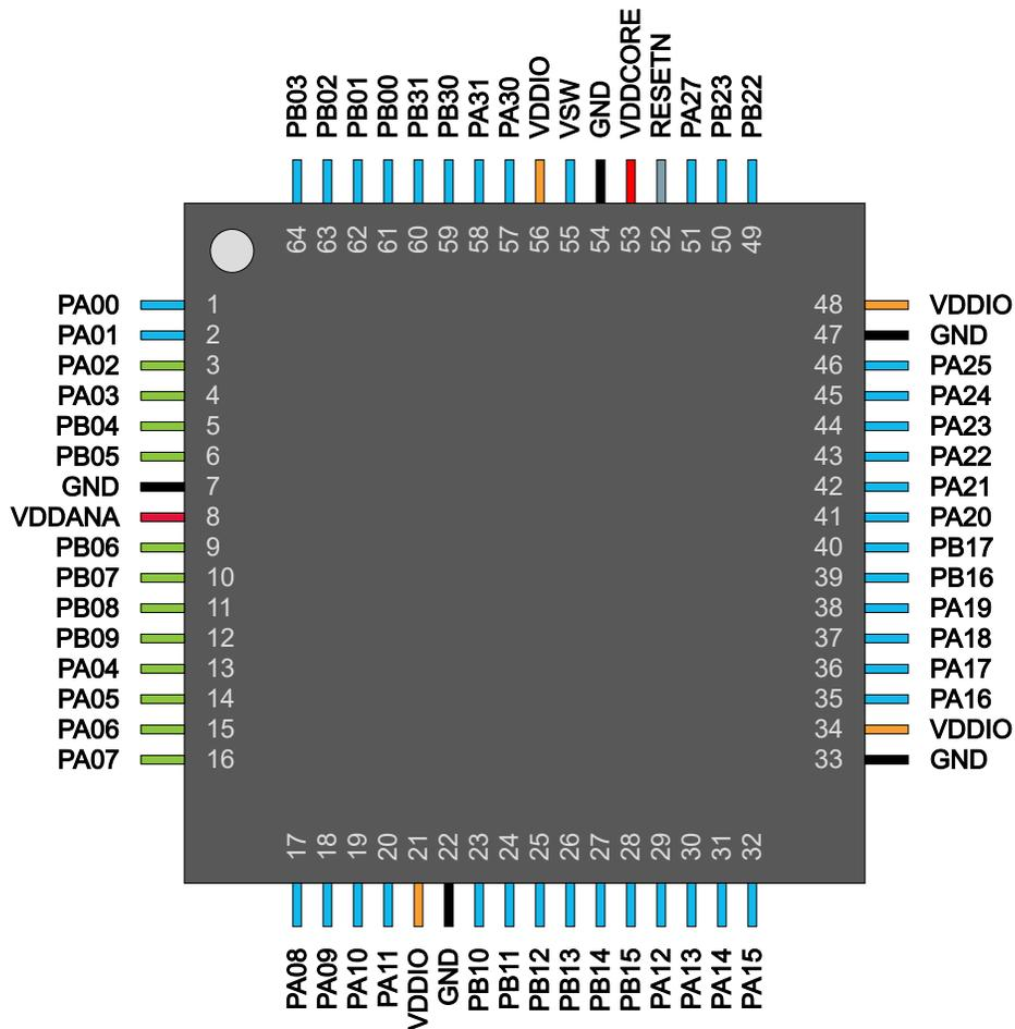
Figure 4-2. 64-Pin WLCSP Package
