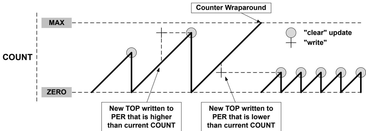
A counter wraparound can occur in any operation mode when up-counting without buffering, see [Figure 48-8](#).
