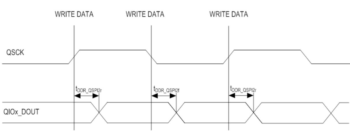
**Figure 54-16. QSPI DDR Mode 0 WRITE**
