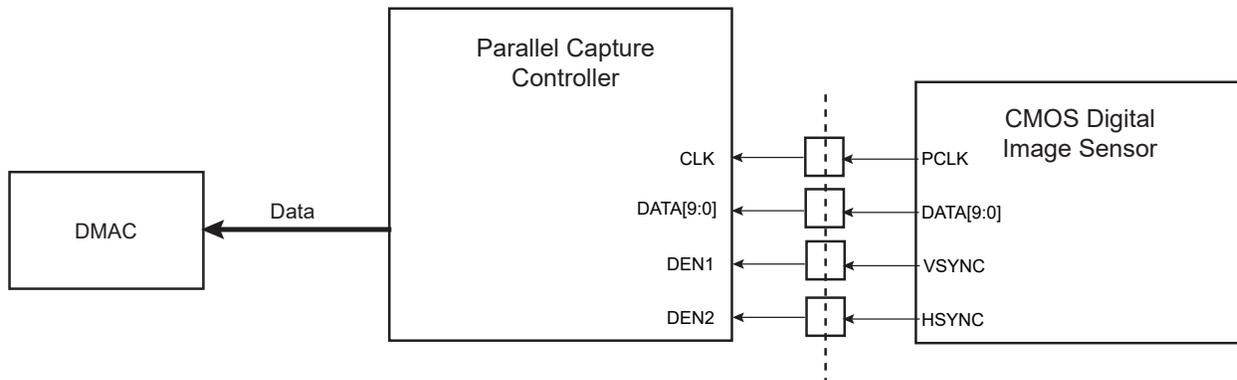
The PCC must be configured first, and is enabled by writing a '1' to the Parallel Capture Enable bit in the Mode Register (MR.PCEN).
