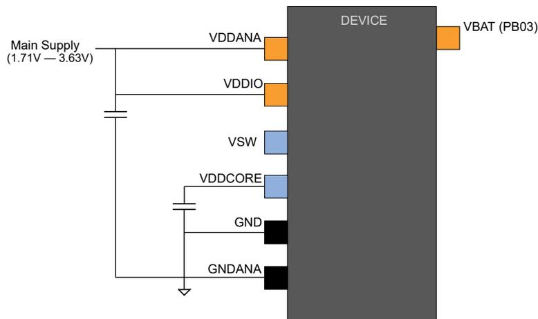
**Figure 7-3. Power Supply Connection for Switching/Linear Mode**
