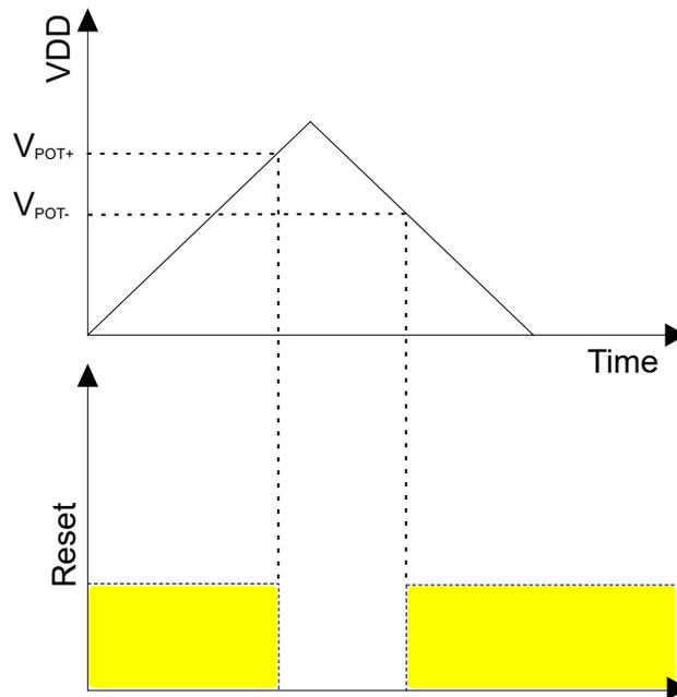
**Note:** The shaded area indicates that the device is in a Reset state.
