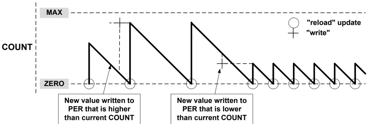
A counter wraparound can occur in any operation mode when up-counting without buffering, see [Figure 49-10](#). COUNT and TOP are continuously compared, so when a new value that is lower than the current COUNT is written to TOP, COUNT will wrap before a compare match.
