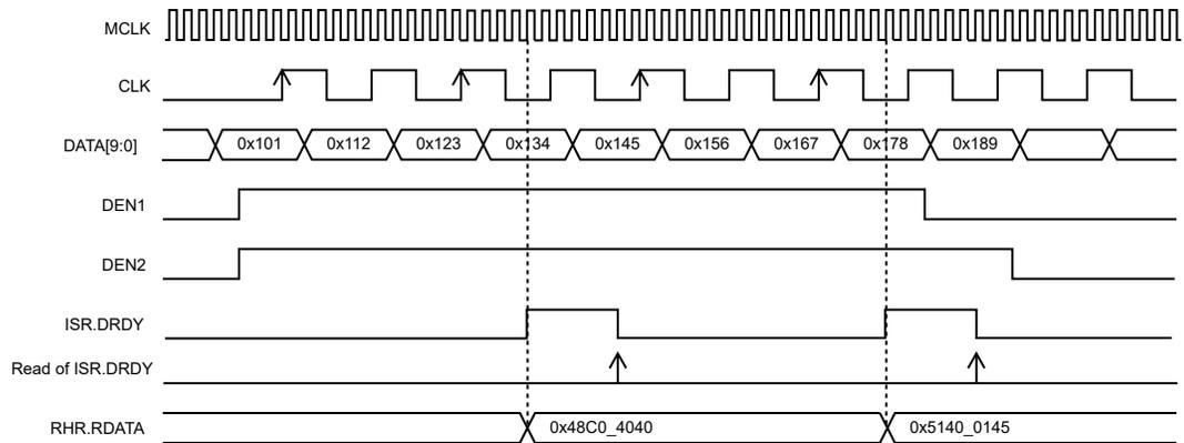
**Figure 52-12. PCC Waveforms (DSIZE=4\_DATA, ALWAYS = 0, HALFS = 1, FRSTS = 1)**
