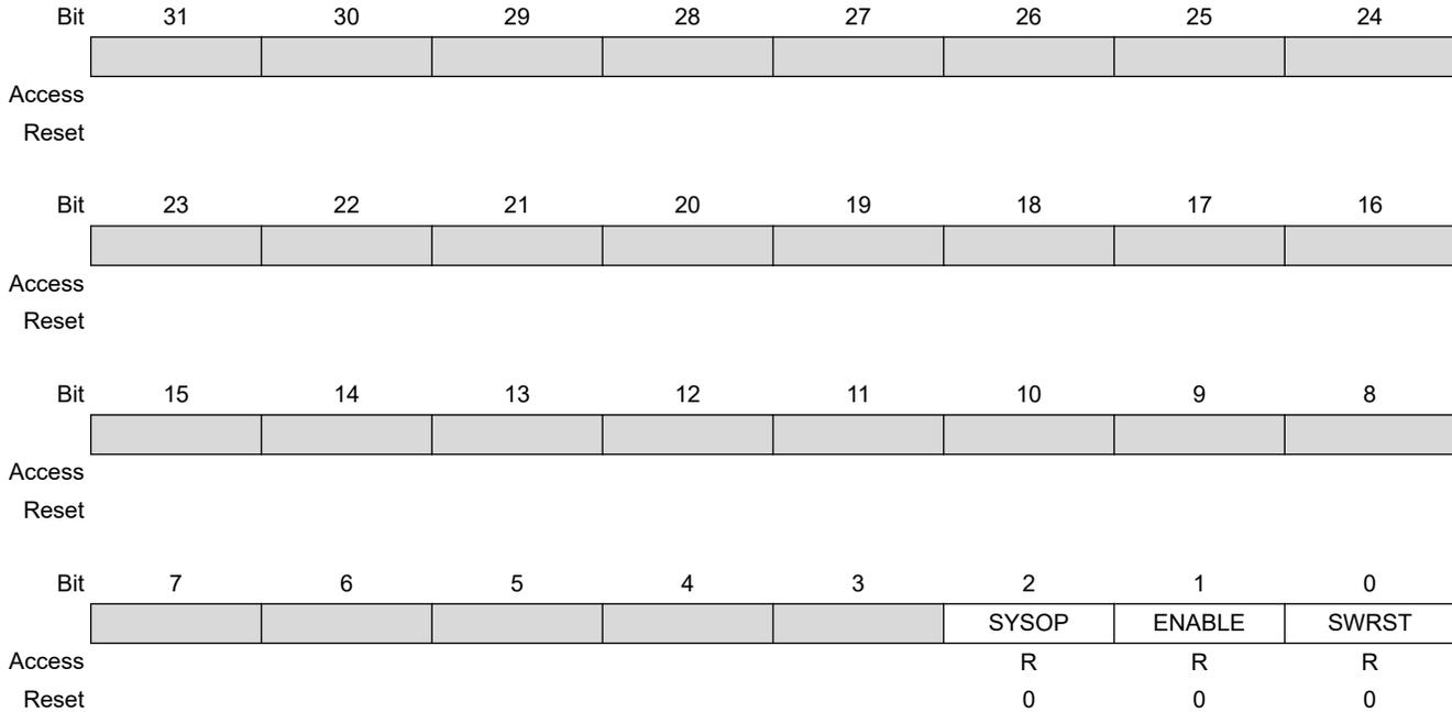
**Bit 2 – SYSOP** System Operation Synchronization Busy
