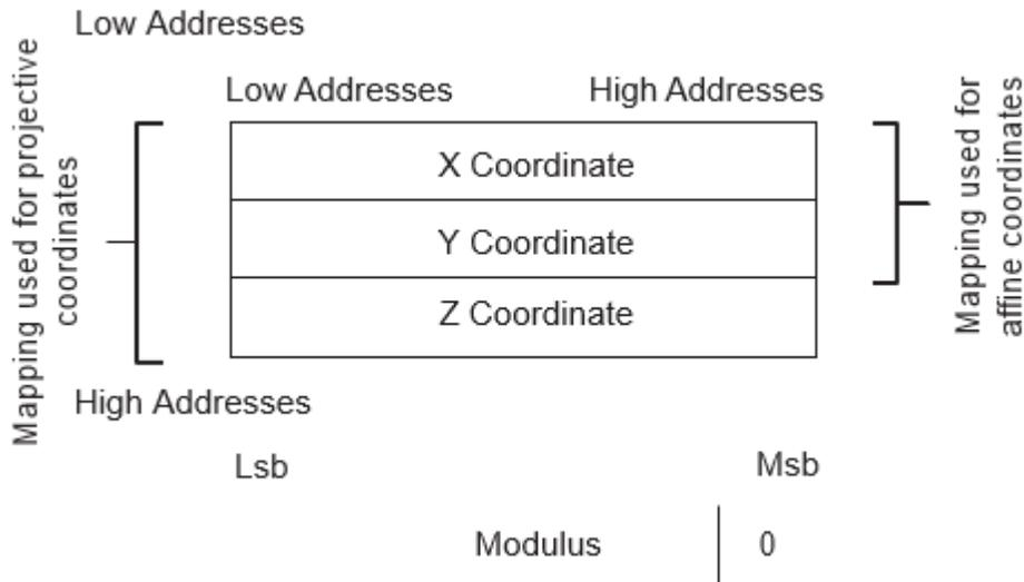
In this figure, the modulus is represented as a reference, and to show that coordinates are always to be provided on the length of the modulus plus one 32-bit word.
