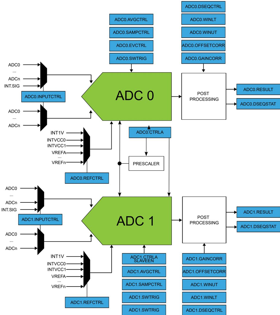
In this mode of operation, the slave ADC1 is enabled by accessing the CTRLA register of the master ADC0. In the same way, the master ADC event inputs will be automatically routed to the slave ADC, meaning that the input events configuration must be done in the master ADC (ADC0.EVCTRL).
