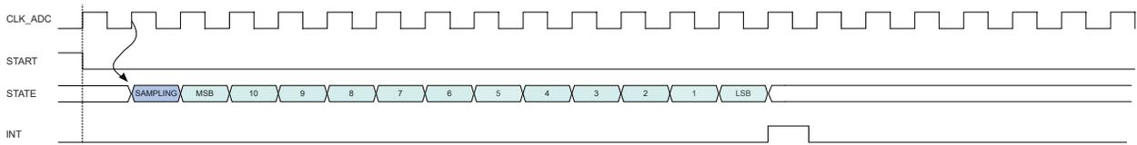
The sampling time can be increased by using the Sampling Time Length bit group in the Sampling Time Control register (SAMPCTRL.SAMPLEN). As example, the next figure is showing the timing conversion with sampling time increased to six CLK\_ADC cycles.
