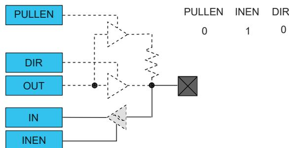
**Figure 32-5. I/O Configuration - Input with Pull**
