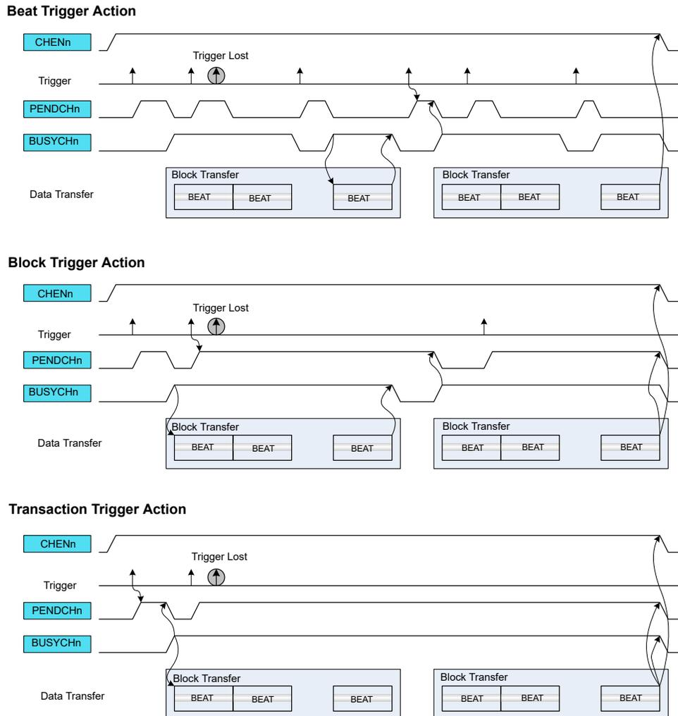
If the trigger source generates a transfer request for a channel during an ongoing transfer, the new transfer request will be kept pending (CHSTATUSn.PEND=1), and the new transfer can start after the ongoing one is done. Only one pending transfer can be kept per channel. If the trigger source generates more transfer requests while one is already pending, the additional ones will be lost. All channels pending status flags are also available in the Pending Channels register (PENDCH).
