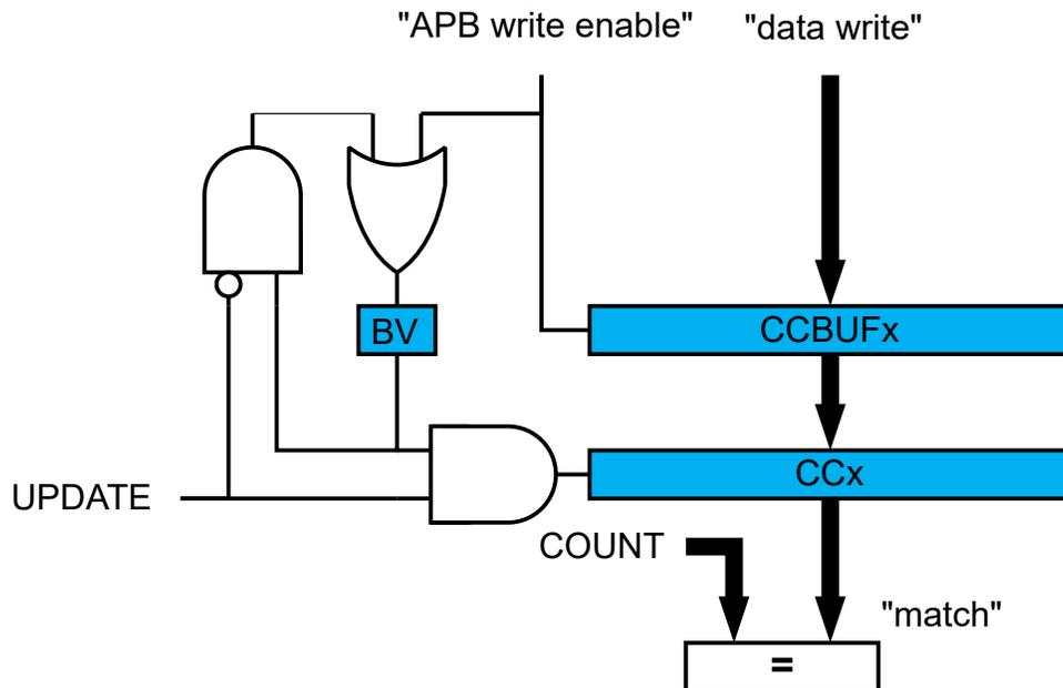
Both the registers (PATT/PER/CC<sub>x</sub>) and corresponding buffer registers (PATTBUFPERBUF/CCBUF<sub>x</sub>) are available in the I/O register map, and the double buffering feature is not mandatory. The double buffering is disabled by writing a '1' to CTRLSET.LUPD.
