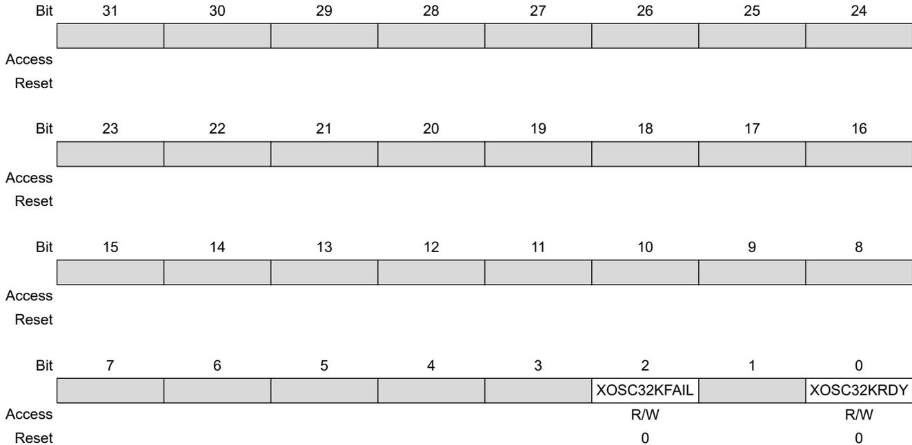
**Bit 2 – XOSC32KFAIL** XOSC32K Clock Failure Detector Interrupt Enable
