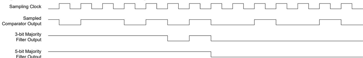
**Figure 46-7. Single-Shot Filtering**
