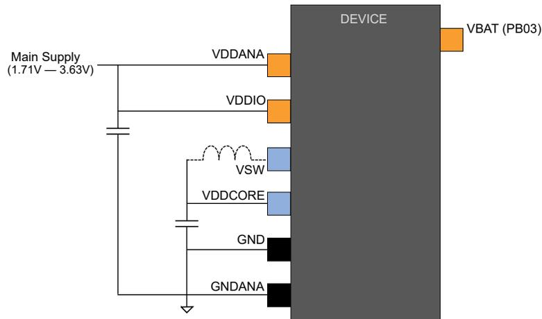
**Figure 7-4. Power Supply Connection for Battery Backup**
