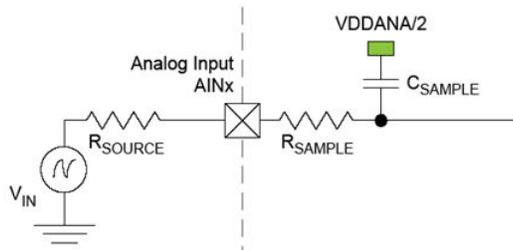
The minimum sampling time  $t_{\text{samplehold}}$  for a given  $R_{\text{source}}$  can be found using a general formula:
