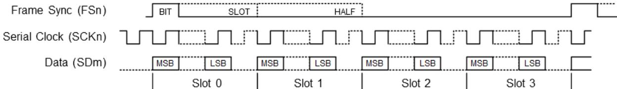
Data bits are sent on the falling edge of the Serial Clock and sampled on the rising edge of the Serial Clock. The FSn pin provides a frame synchronization signal, at the beginning of slot 0. The delay between the frame start and the first data bit is defined by writing the CLKCTRLn.BITDELAY field.
