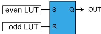
When the even LUT is disabled (LUTCTRL0.ENABLE=0 / LUTCTRL2.ENABLE=0), the latch output will be cleared. The R-input is forced enabled for one more APB clock cycle and S-input to zero. In all other cases, the latch output (OUT) is refreshed as shown in [Table 41-5](#).
