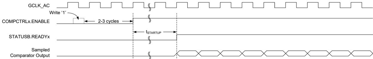
For low-power operation, comparisons can be performed during sleep modes without a clock. The comparator is enabled continuously, and changes of the comparator state are detected asynchronously. When a toggle occurs, the Power Manager will start GCLK\_AC to register the appropriate peripheral events and interrupts. The GCLK\_AC clock is then disabled again automatically, unless configured to wake up the system from sleep.
