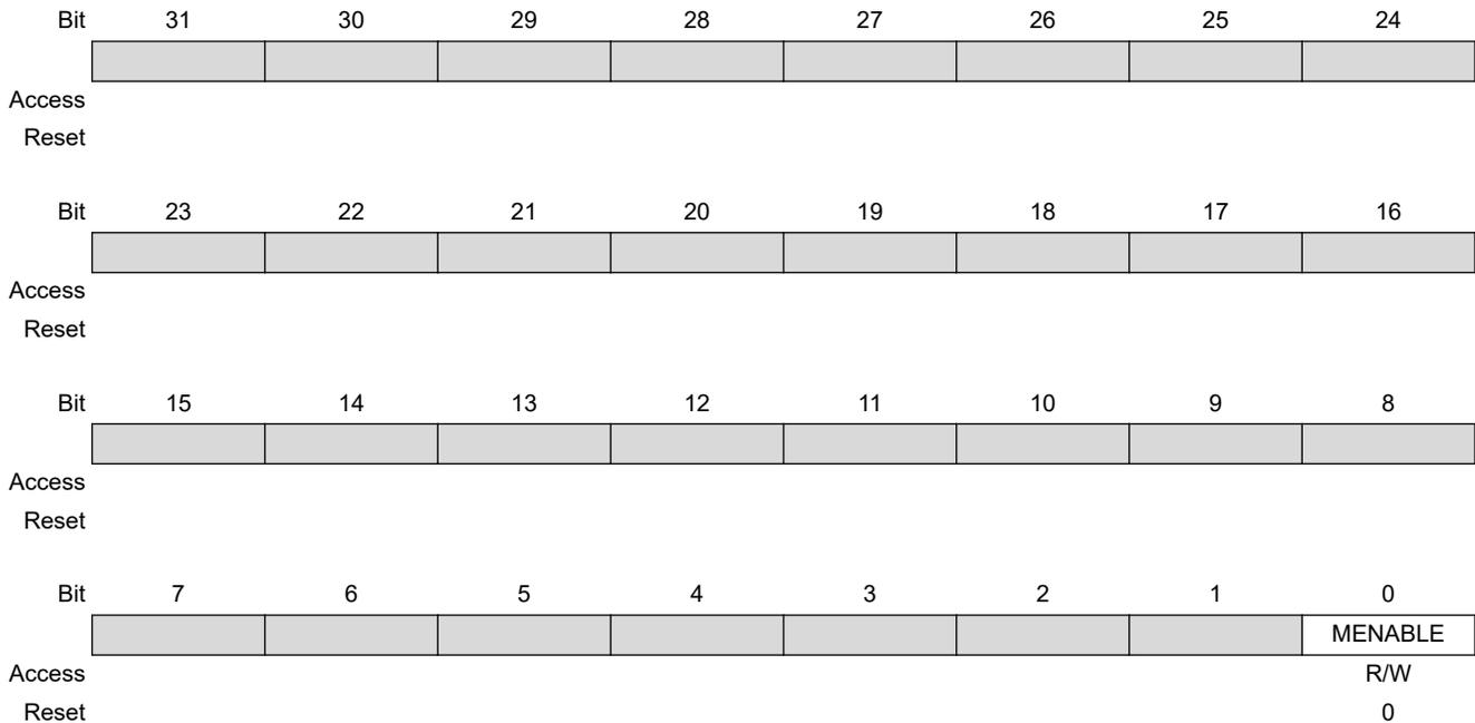
**Bit 0 – MENABLE** Cache Controller Monitor Enable
