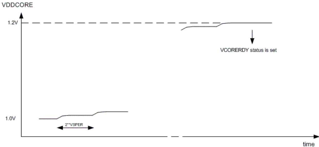
The STATUS.VCORERDY bit is set to '1' as soon as the VDDCORE voltage has reached the target voltage. During voltage transition, STATUS.VCORERDY will read '0'. The Voltage Ready interrupt (VCORERDY) can be used to detect a 0-to-1 transition of STATUS.VCORERDY, see also [19.5.5 Interrupts](#).
