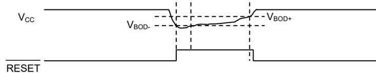
Enabling the BOD33 hysteresis by writing the Hysteresis bit field in the BOD33 register (BOD33.HYST) to a non-null value will add hysteresis to the BOD33 threshold level.
