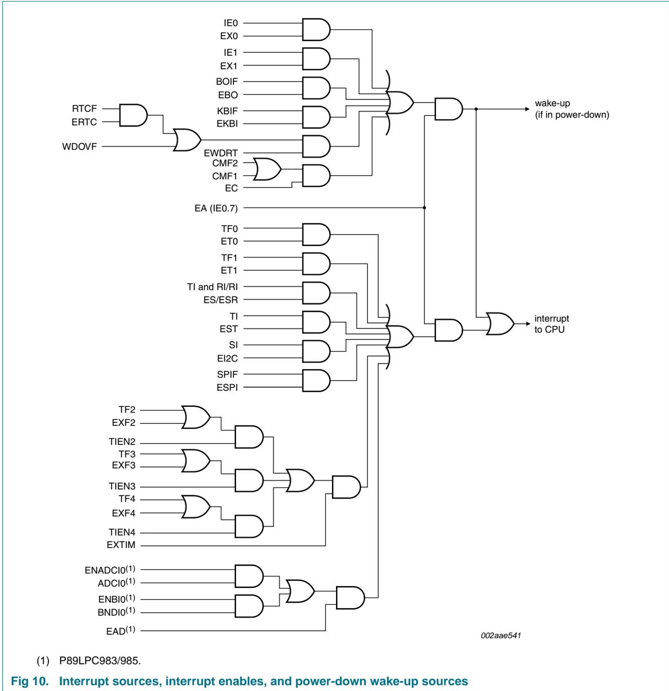
Fig 10. Interrupt sources, interrupt enables, and power-down wake-up sources
