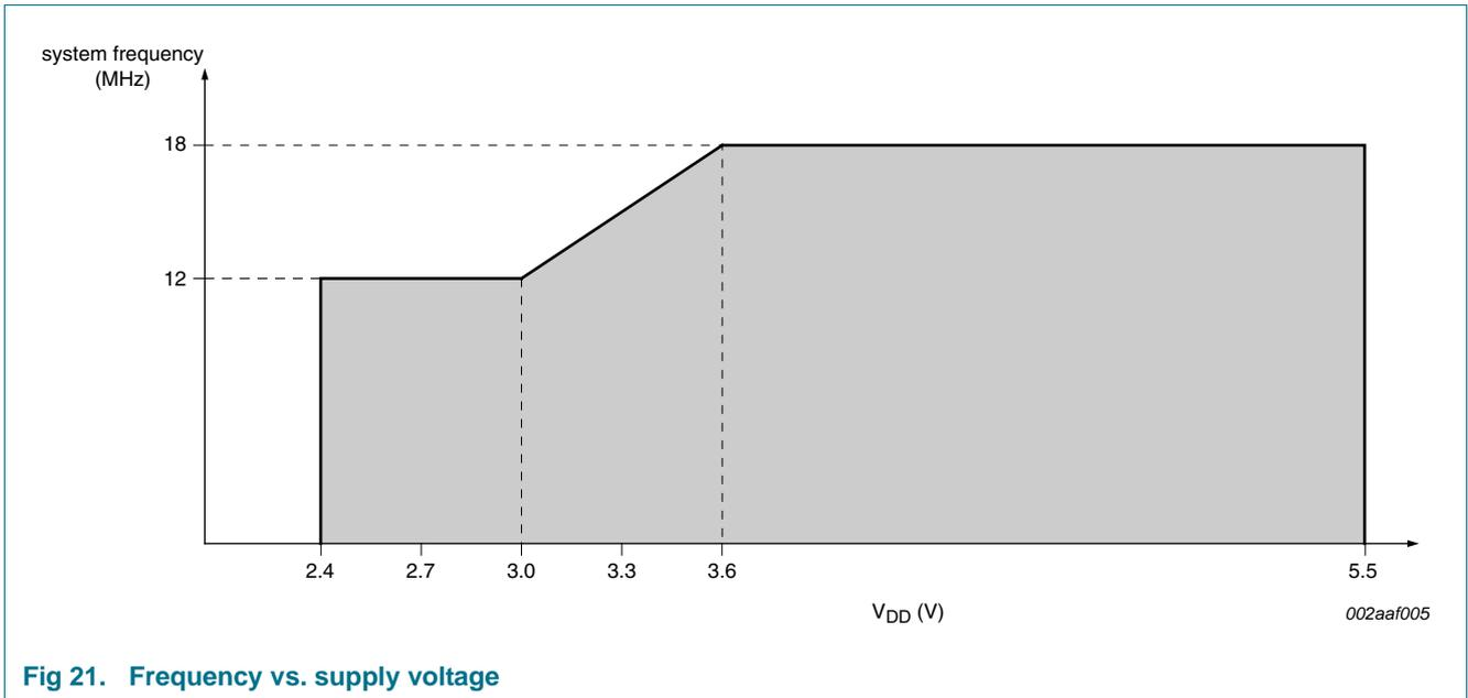
Fig 21. Frequency vs. supply voltage
