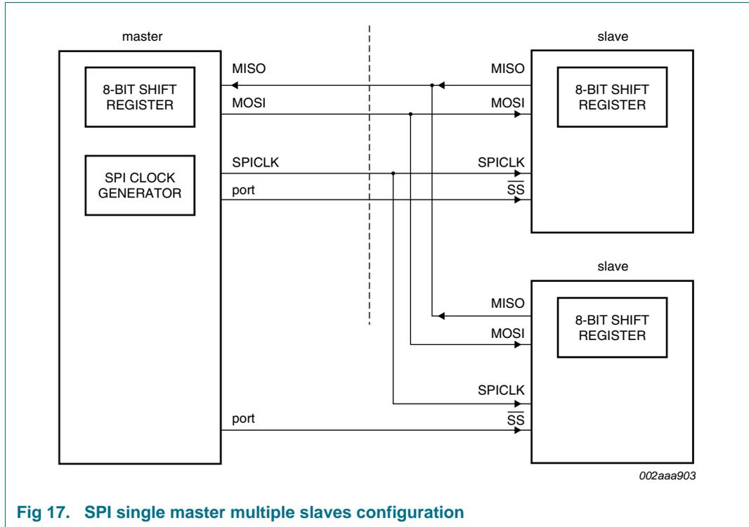
**Fig 17. SPI single master multiple slaves configuration**
