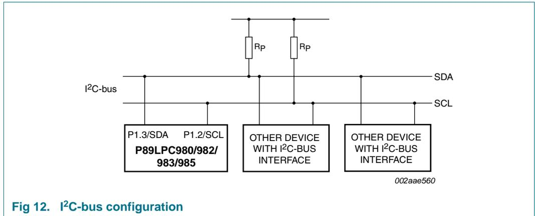
**Fig 12.** I<sup>2</sup>C-bus configuration
