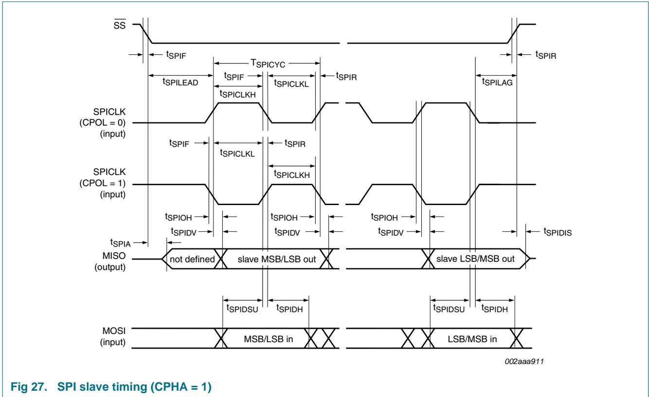
Fig 27. SPI slave timing (CPHA = 1)
