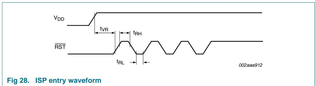
Fig 28. ISP entry waveform
