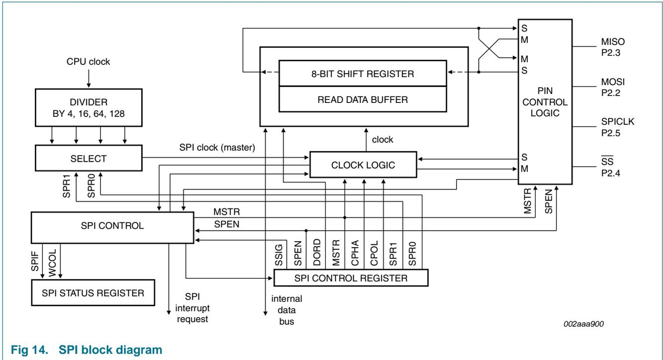
Fig 14. SPI block diagram
