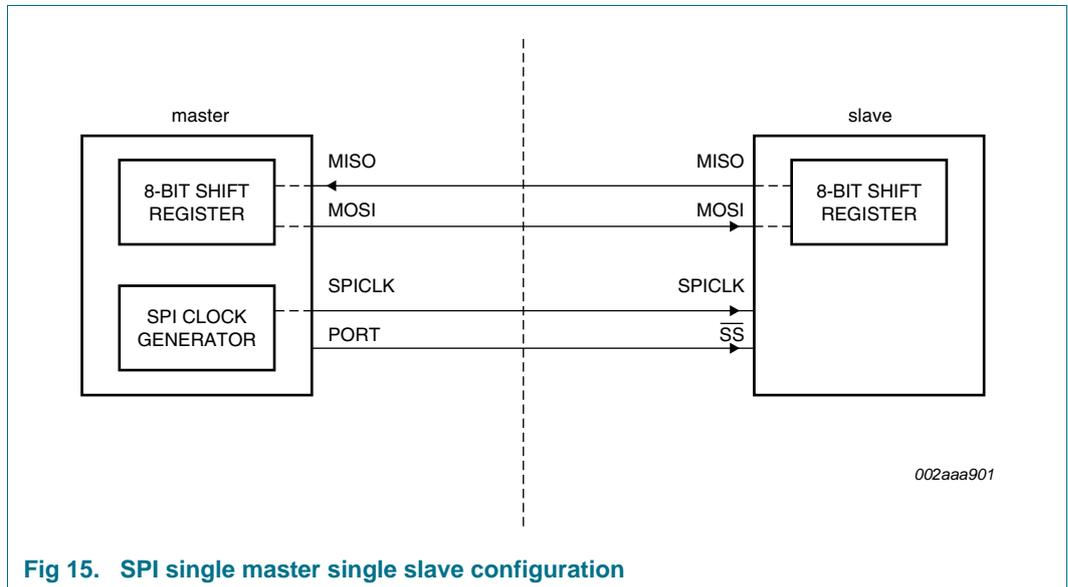
**Fig 15. SPI single master single slave configuration**
