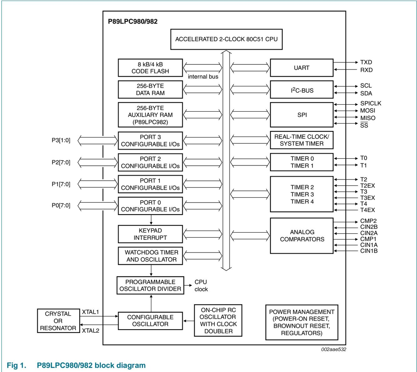
Fig 1. P89LPC980/982 block diagram
