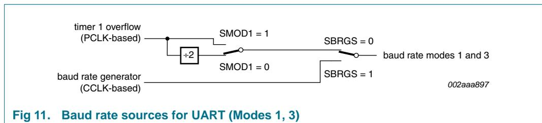
**Fig 11. Baud rate sources for UART (Modes 1, 3)**
