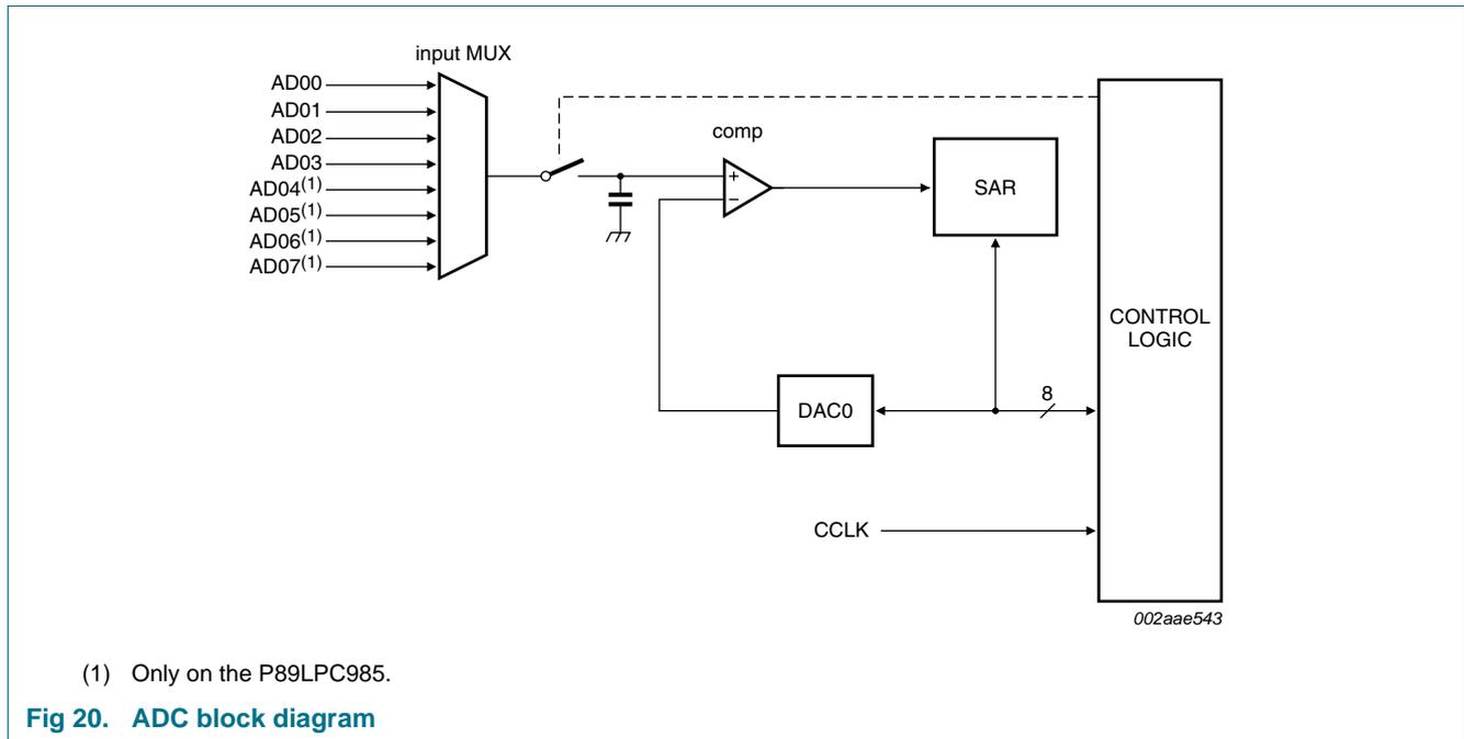
Fig 20. ADC block diagram
