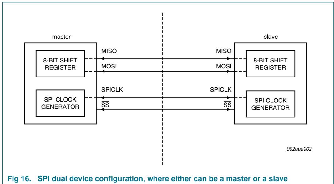
**Fig 16. SPI dual device configuration, where either can be a master or a slave**
