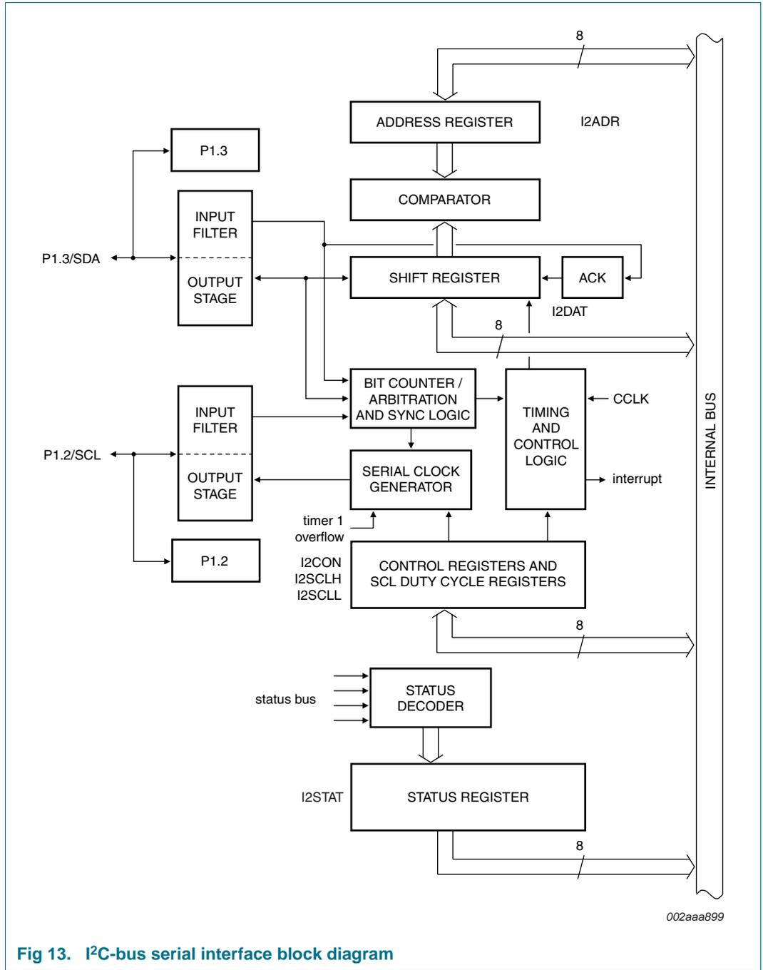
**Fig 13. I<sup>2</sup>C-bus serial interface block diagram**
