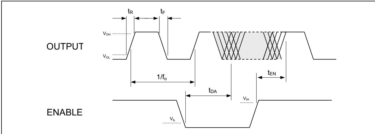
**FIGURE 3-1:** Output Waveform.
