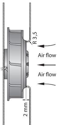
The air flow and sound level of the centrifugal fans without external housing depend on their individual installation conditions.
