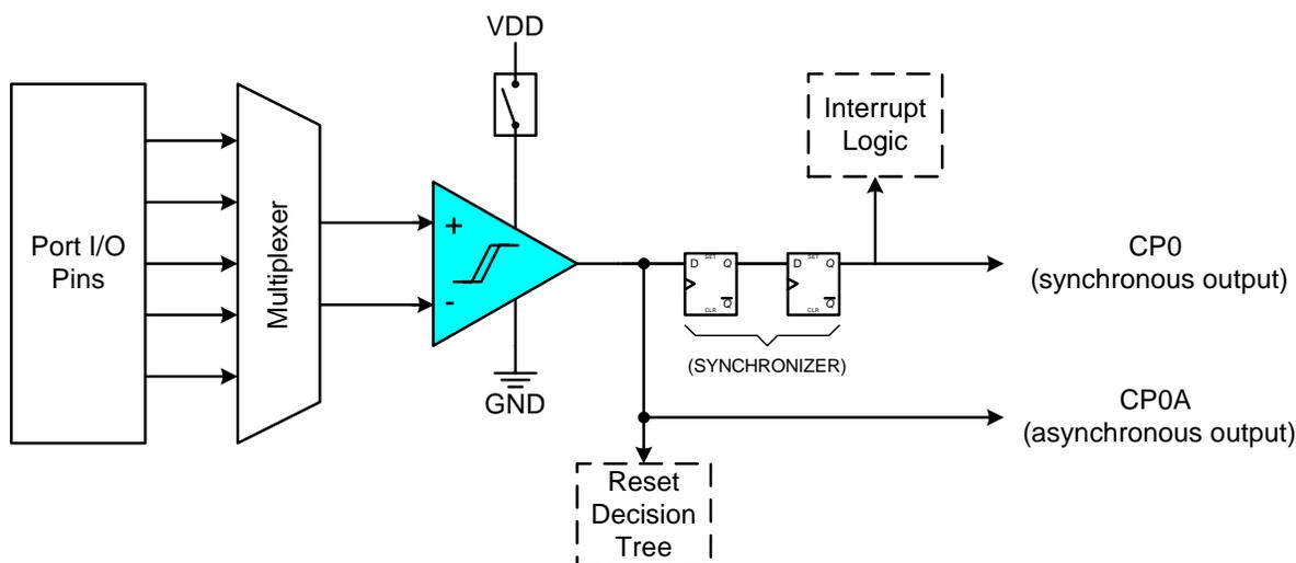
Figure 1.9. Comparator0 Block Diagram
