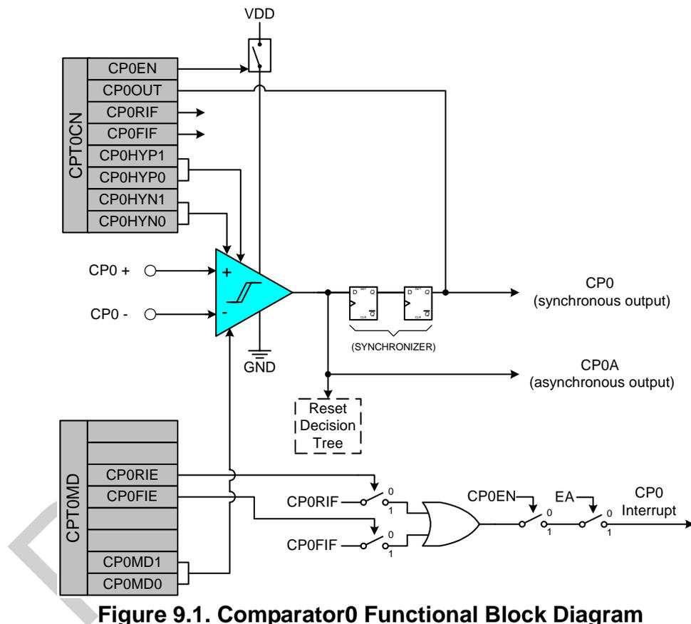
**Figure 9.1. Comparator0 Functional Block Diagram**
