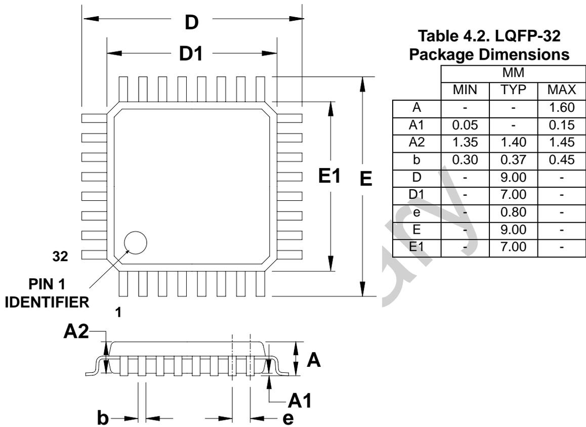
Figure 4.3. LQFP-32 Package Diagram
