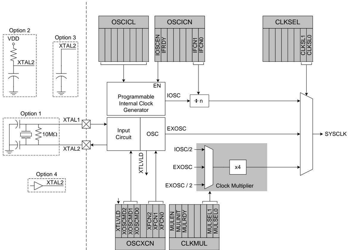
**Figure 17.1. Oscillator Diagram**
