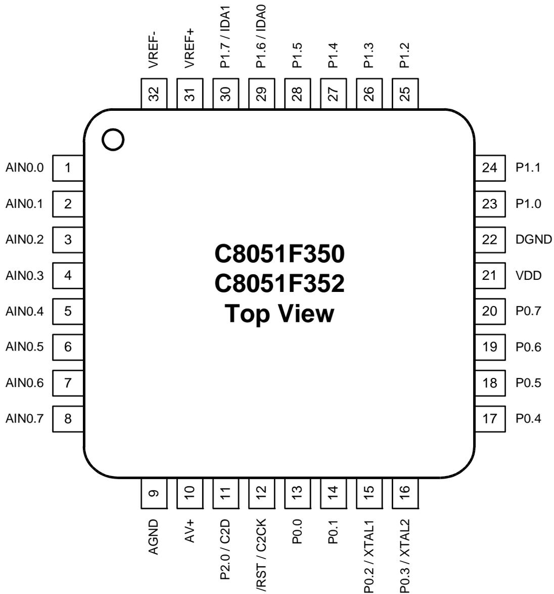
Figure 4.1. LQFP-32 Pinout Diagram (Top View)
