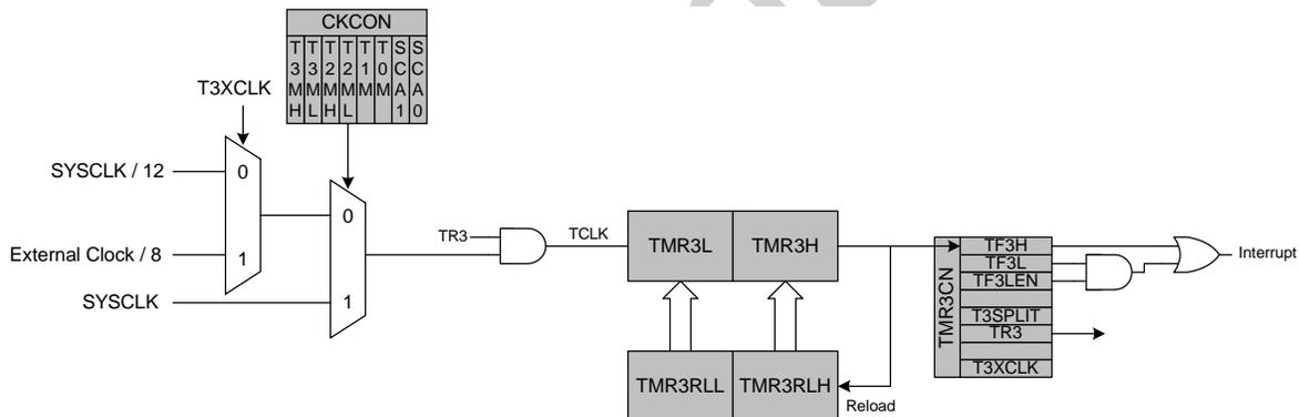
Figure 22.18. Timer 3 16-Bit Mode Block Diagram
