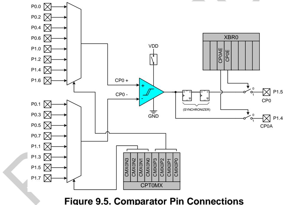
Figure 9.5. Comparator Pin Connections
