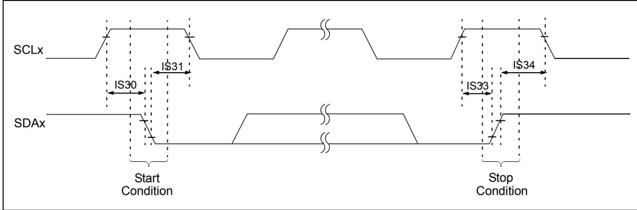
**FIGURE 22-20: I2Cx BUS DATA TIMING CHARACTERISTICS (SLAVE MODE)**
