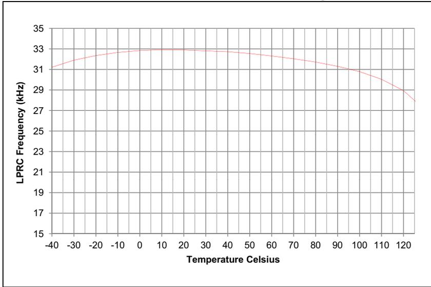
FIGURE 24-13: TYPICAL FRC FREQUENCY @ VDD = 3.3V
