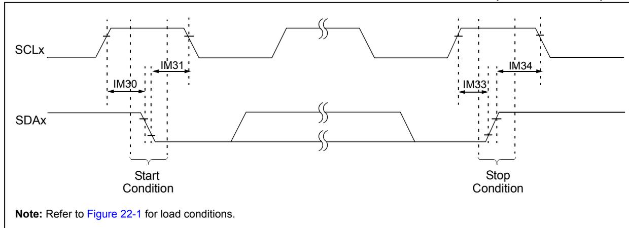
**FIGURE 22-18: I2Cx BUS DATA TIMING CHARACTERISTICS (MASTER MODE)**
