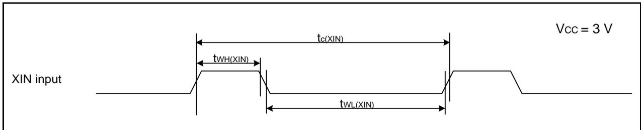
Figure 5.13 XIN Input Timing Diagram when  $V_{CC} = 3\text{ V}$ Table 5.24 CNTR0 Input, CNTR1 Input,  $\overline{INT1}$  Input
