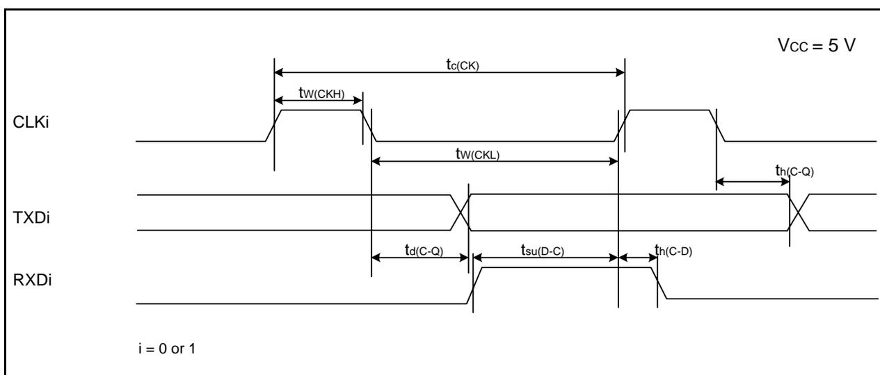
**Figure 5.11 Serial Interface Timing Diagram when Vcc = 5 V****Table 5.20 External Interrupt  $\overline{INT0}$  Input**
