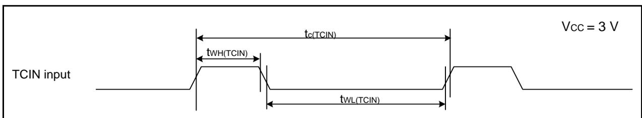
Figure 5.15 TCIN Input,  $\overline{INT3}$  Input Timing Diagram when  $V_{CC} = 3\text{ V}$
