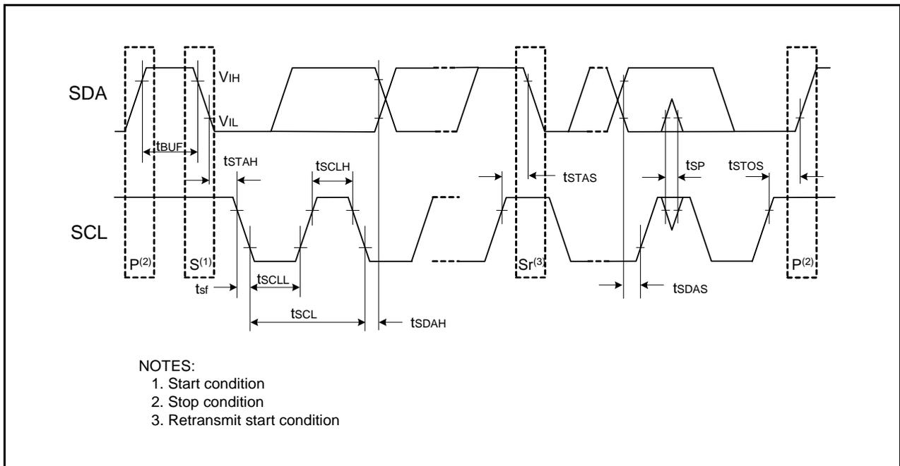
**Figure 5.7 I/O Timing of I<sup>2</sup>C bus Interface**
