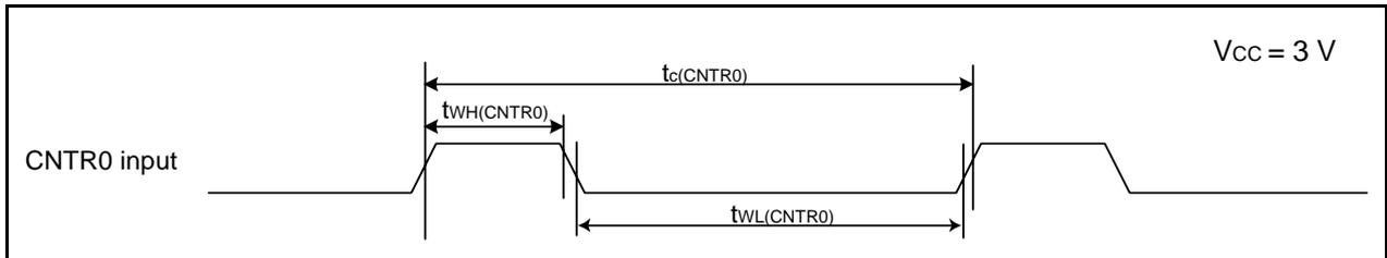
Figure 5.14 CNTR0 Input, CNTR1 Input,  $\overline{INT1}$  Input Timing Diagram when  $V_{CC} = 3\text{ V}$ Table 5.25 TCIN Input,  $\overline{INT3}$  Input
