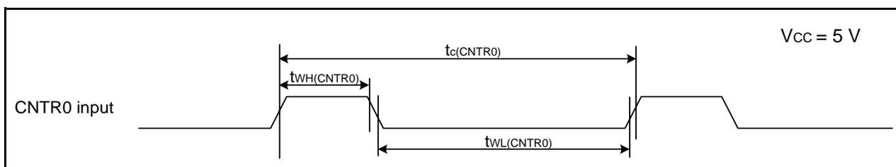
**Figure 5.9 CNTR0 Input, CNTR1 Input,  $\overline{INT1}$  Input Timing Diagram when  $V_{CC} = 5\text{ V}$** **Table 5.18 TCIN Input,  $\overline{INT3}$  Input**
