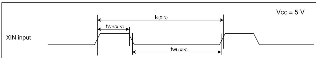
**Figure 5.8 XIN Input Timing Diagram when  $V_{CC} = 5\text{ V}$** **Table 5.17 CNTR0 Input, CNTR1 Input,  $\overline{INT1}$  Input**
