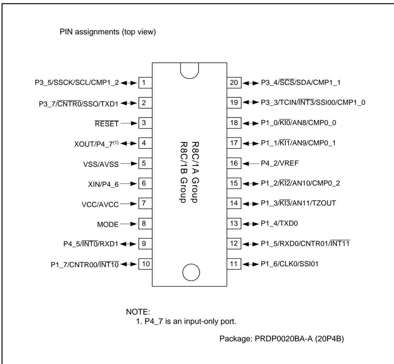
Figure 1.5 Pin Assignments for PRDP0020BA-A Package (Top View)
