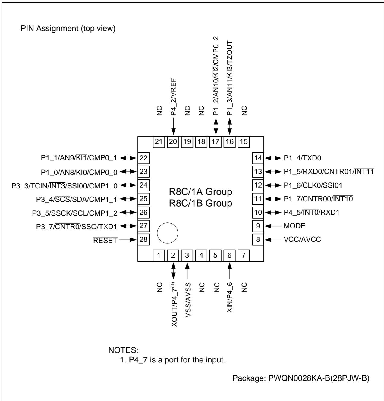
Figure 1.6 Pin Assignments for PWQN0028KA-B Package (Top View)
