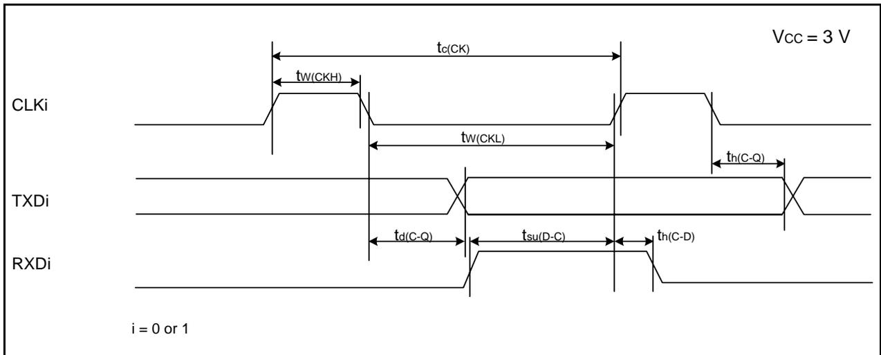
**Figure 5.16 Serial Interface Timing Diagram when Vcc = 3 V**
