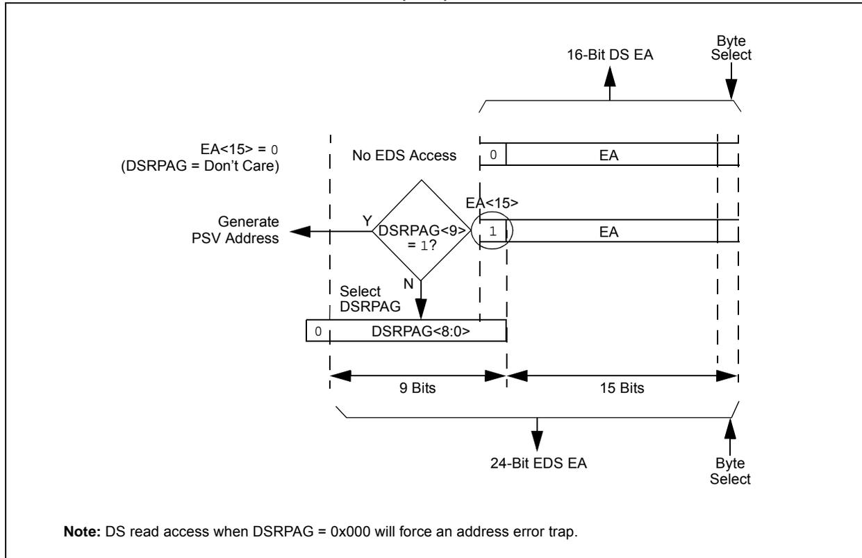
**FIGURE 4-9: EXTENDED DATA SPACE (EDS) WRITE ADDRESS GENERATION**
