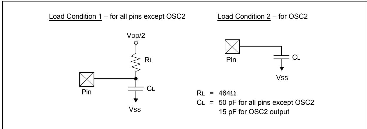
**TABLE 33-15: CAPACITIVE LOADING REQUIREMENTS ON OUTPUT PINS**
