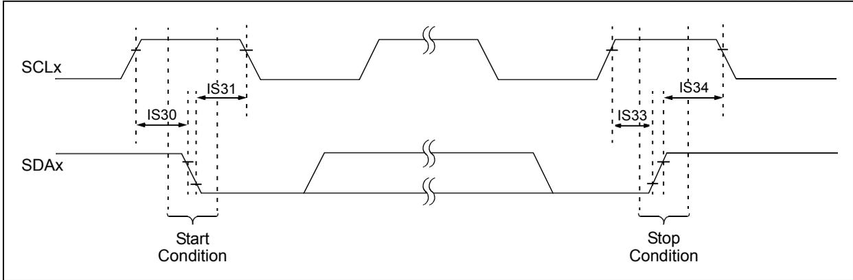
**FIGURE 33-34: I2Cx BUS DATA TIMING CHARACTERISTICS (SLAVE MODE)**
