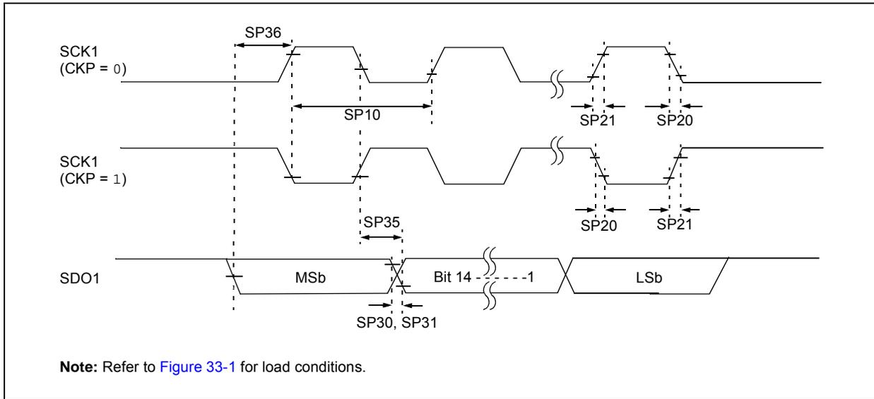
**TABLE 33-41: SPI1 MASTER MODE (HALF-DUPLEX, TRANSMIT ONLY) TIMING REQUIREMENTS**
