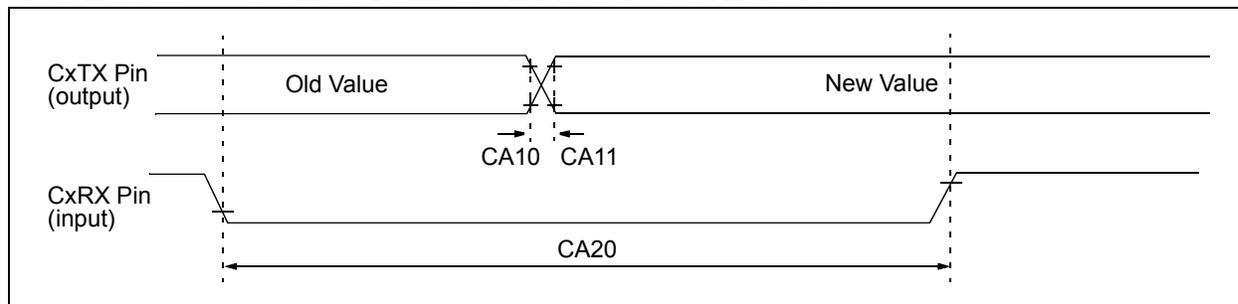
**TABLE 33-50: CANx MODULE I/O TIMING REQUIREMENTS**
