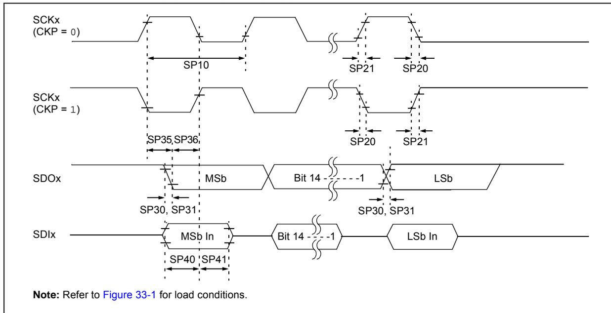
**TABLE 33-35: SPI2 AND SPI3 MASTER MODE (FULL-DUPLEX, CKE = 0, CKP = x, SMP = 1) TIMING REQUIREMENTS**
