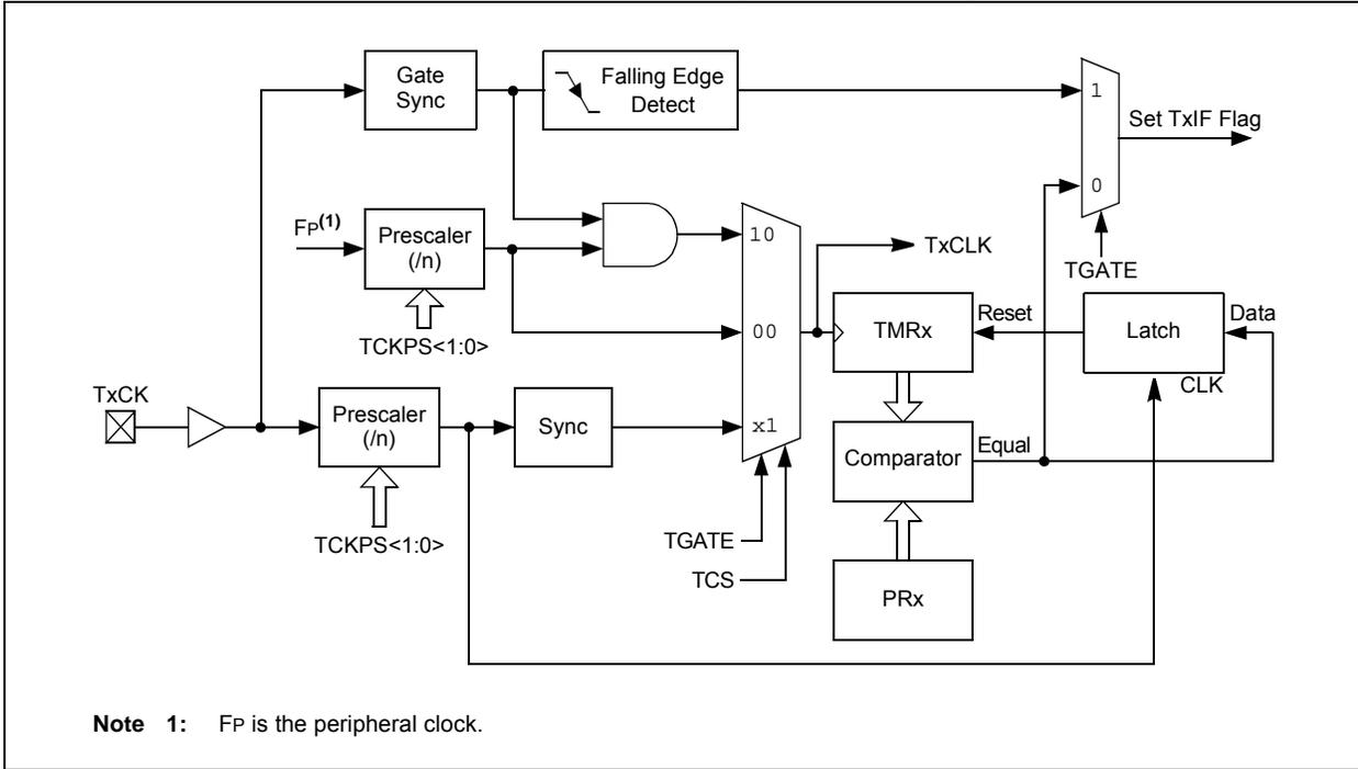
**FIGURE 13-2: TYPE C TIMER BLOCK DIAGRAM (x = 3, 5, 7 AND 9)**
