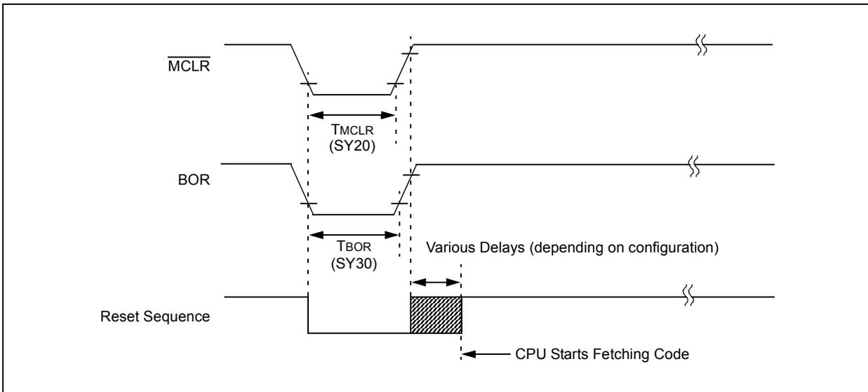
**FIGURE 33-5: POWER-ON RESET TIMING CHARACTERISTICS**
