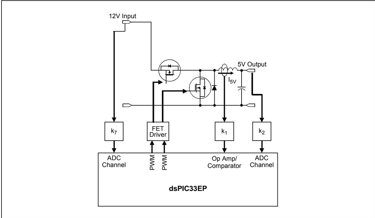
**FIGURE 2-6: MULTIPHASE SYNCHRONOUS BUCK CONVERTER**
