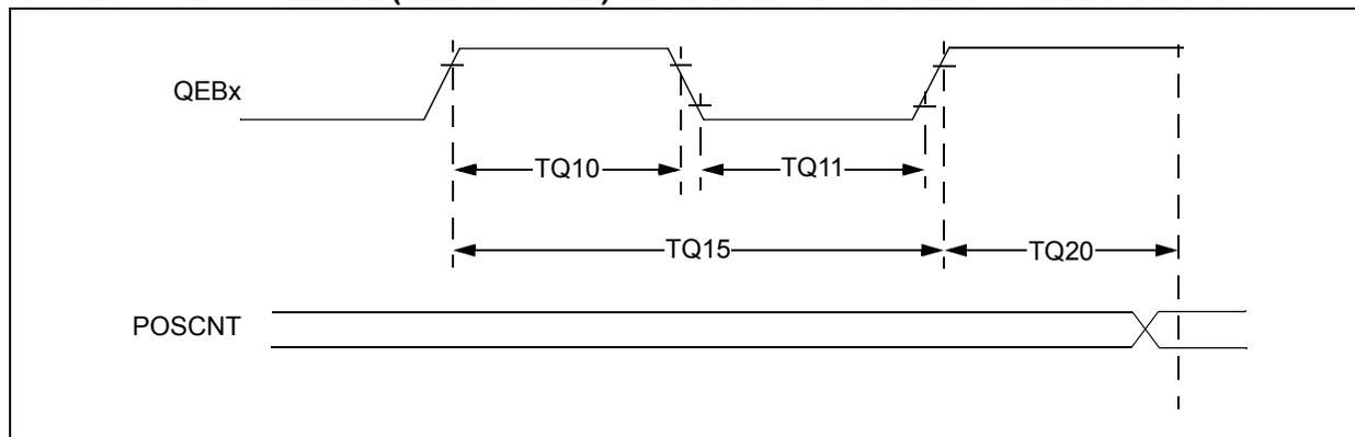
**TABLE 33-29: QEIX MODULE EXTERNAL CLOCK TIMING REQUIREMENTS**
