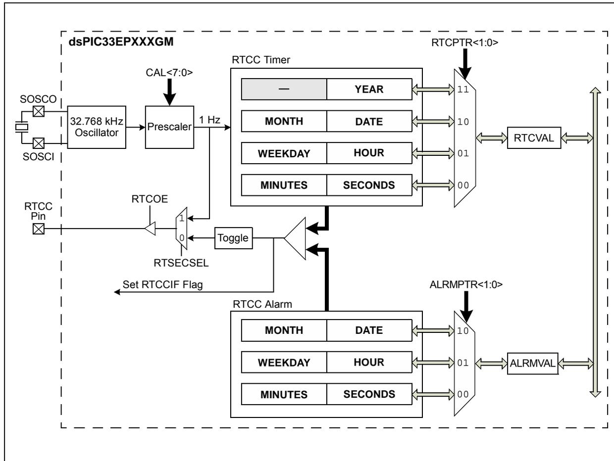
**Note:** The RTCC is only operational on devices which include the SOSC; therefore, the RTCC module is not available on 44-pin devices.
