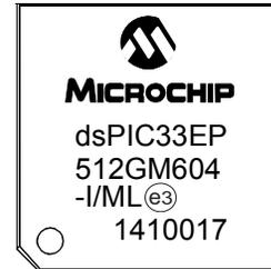
44-Lead QFN (8x8x0.9 mm)
