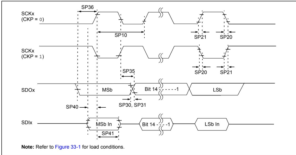
**TABLE 33-34: SPI2 AND SPI3 MASTER MODE (FULL-DUPLEX, CKE = 1, CKP = x, SMP = 1) TIMING REQUIREMENTS**
