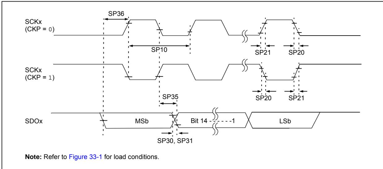
**TABLE 33-33: SPI2 AND SPI3 MASTER MODE (HALF-DUPLEX, TRANSMIT ONLY) TIMING REQUIREMENTS**
