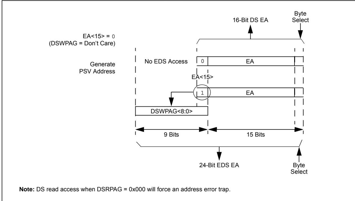
The paged memory scheme provides access to multiple 32-Kbyte windows in the EDS and PSV memory. The Data Space Page registers, DSxPAG, in combination with the upper half of the Data Space address, can provide up to 16 Mbytes of additional address space in the EDS and 8 Mbytes (DSRPAG only) of PSV address space. The paged data memory space is shown in [Figure 4-10](#).
