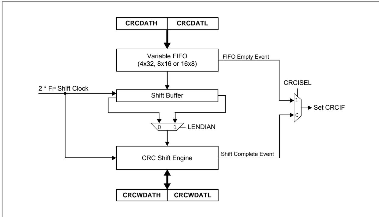
**FIGURE 29-2: CRC SHIFT ENGINE DETAIL**
