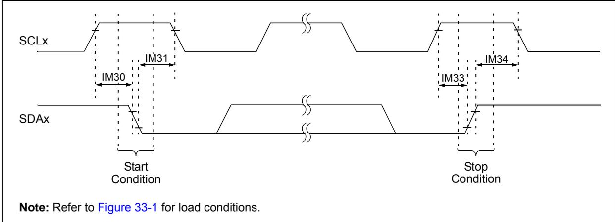
**FIGURE 33-32: I2Cx BUS DATA TIMING CHARACTERISTICS (MASTER MODE)**
