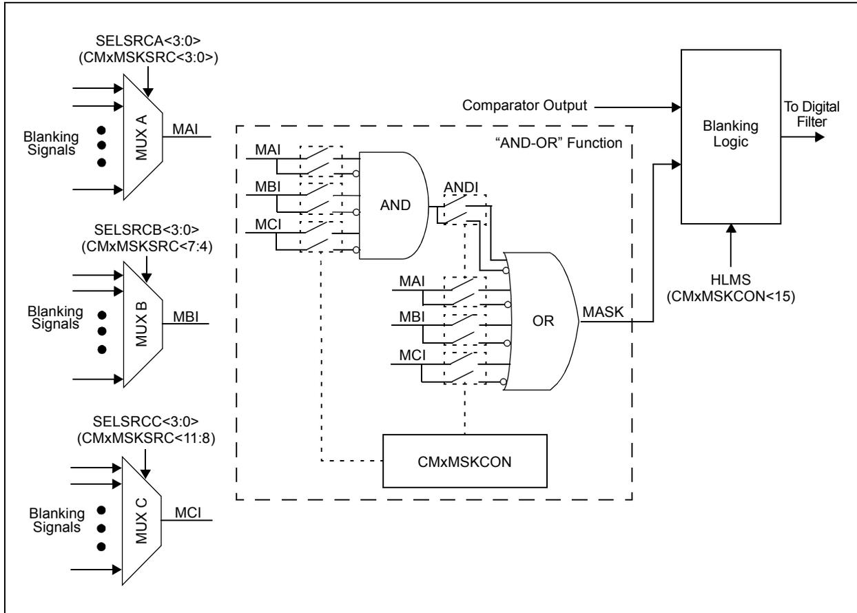
**FIGURE 26-4: DIGITAL FILTER INTERCONNECT BLOCK DIAGRAM**
