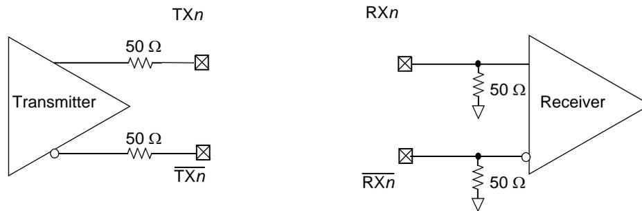
**Figure 26. SerDes Transmitter and Receiver Reference Circuits**
