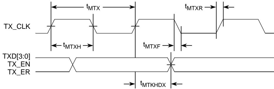
Figure 8. MII Transmit AC Timing Diagram
