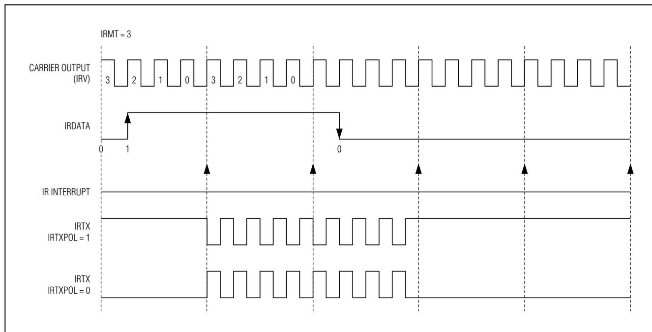
Figure 3. IR Transmission Waveform (IRCFME = 0)
