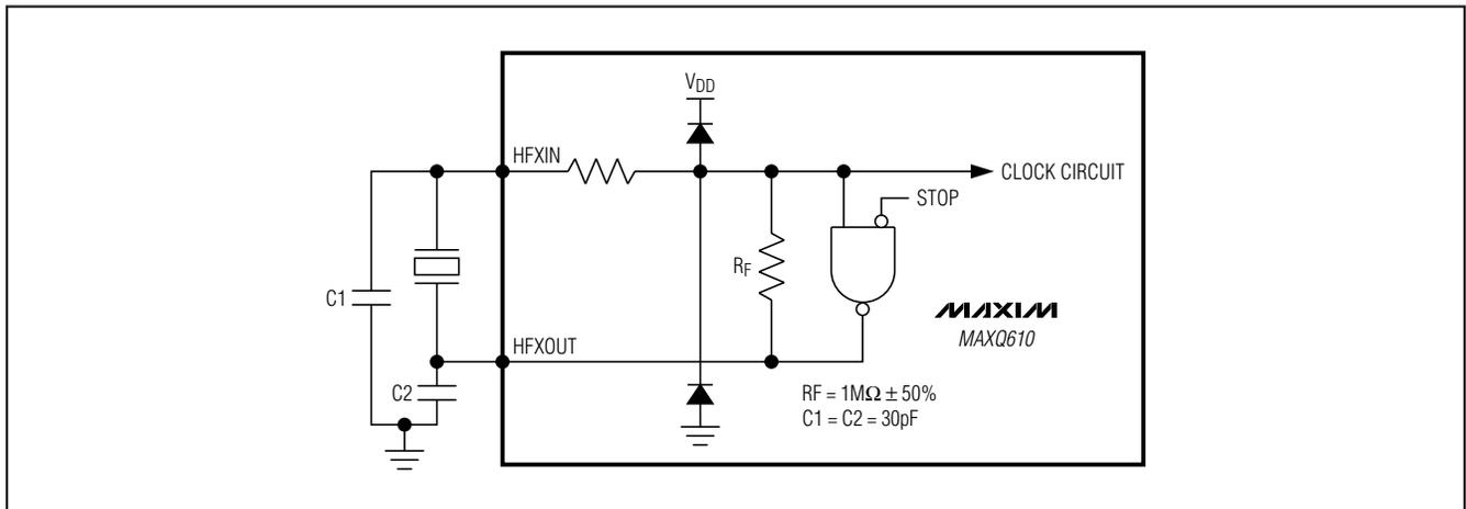
Figure 9. On-Chip Oscillator
