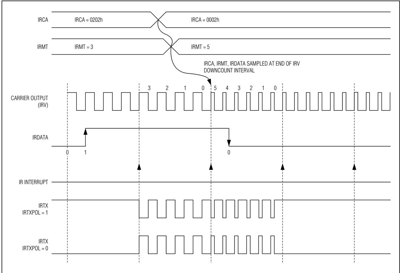
Figure 1. IR Transmit Frequency Shifting Example (IRCFME = 0)
