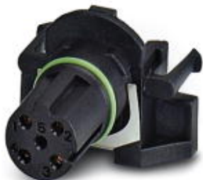
Bus system flush-type socket, Ethernet, 4-pos., shielded, D-coded, with straight solder connection, only contact insert
