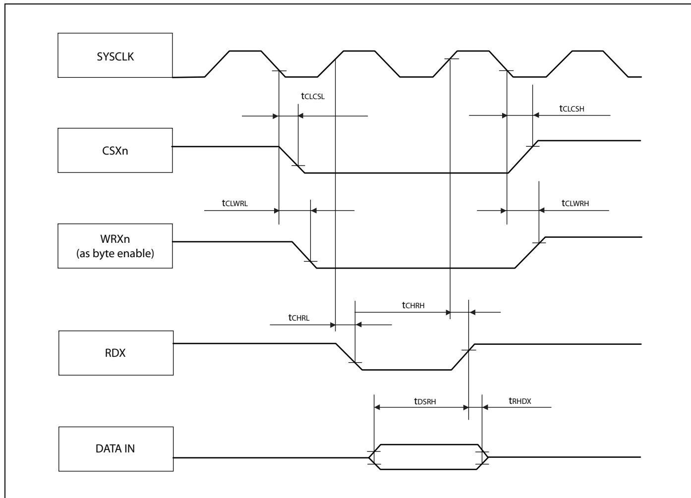
**Synchronous write access - byte control type**
