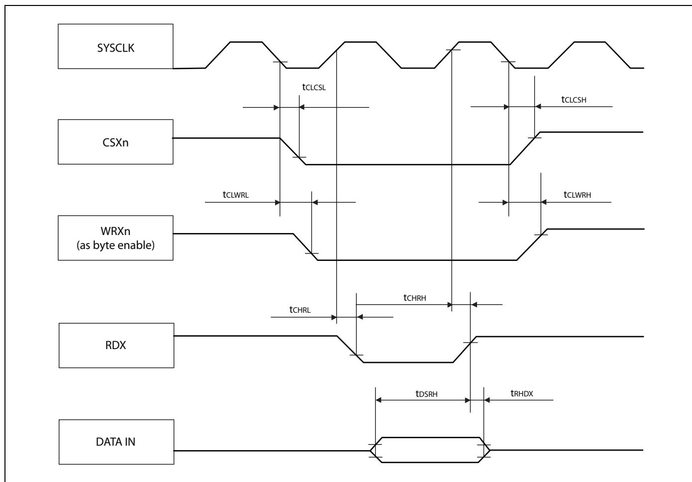
**Synchronous write access - byte control type**
