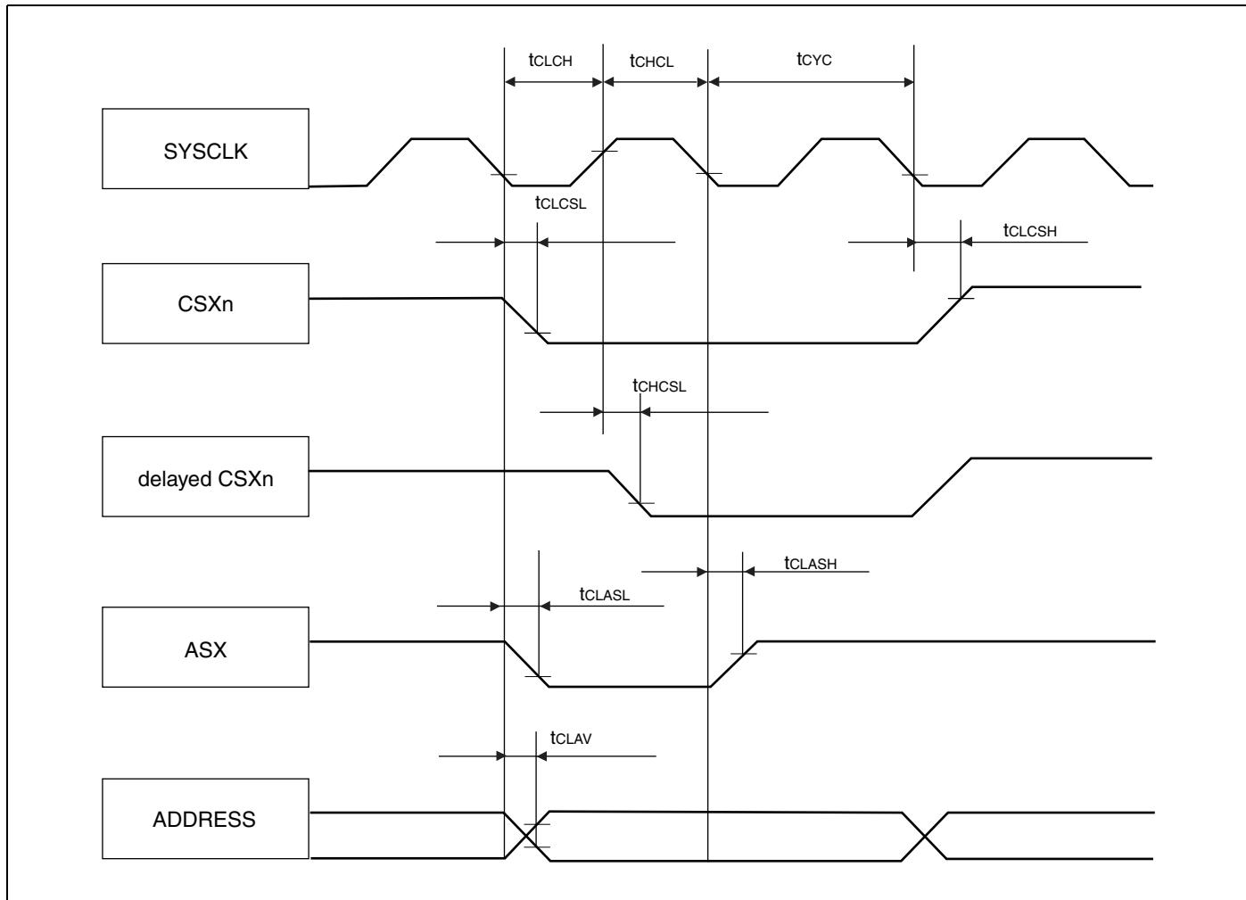
**Synchronous/Asynchronous read access**
