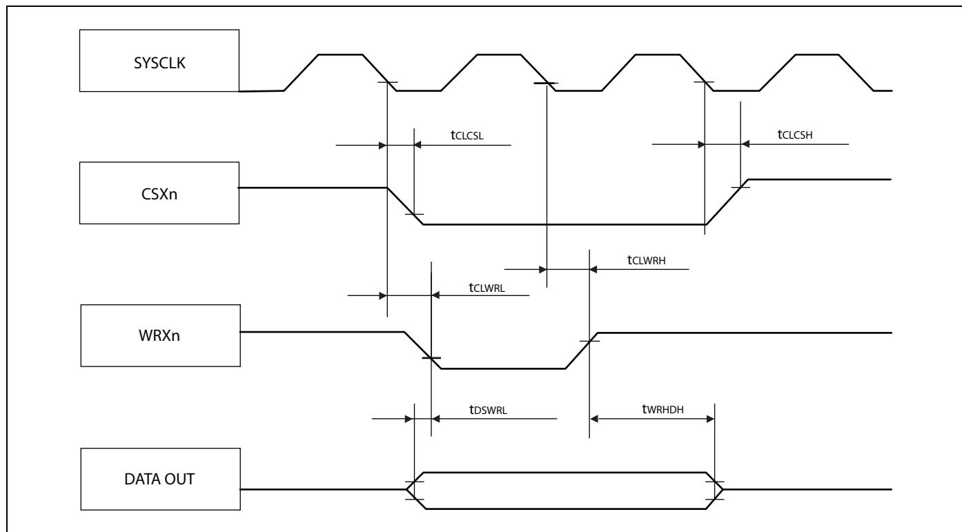
**Asynchronous write access - byte control type**
