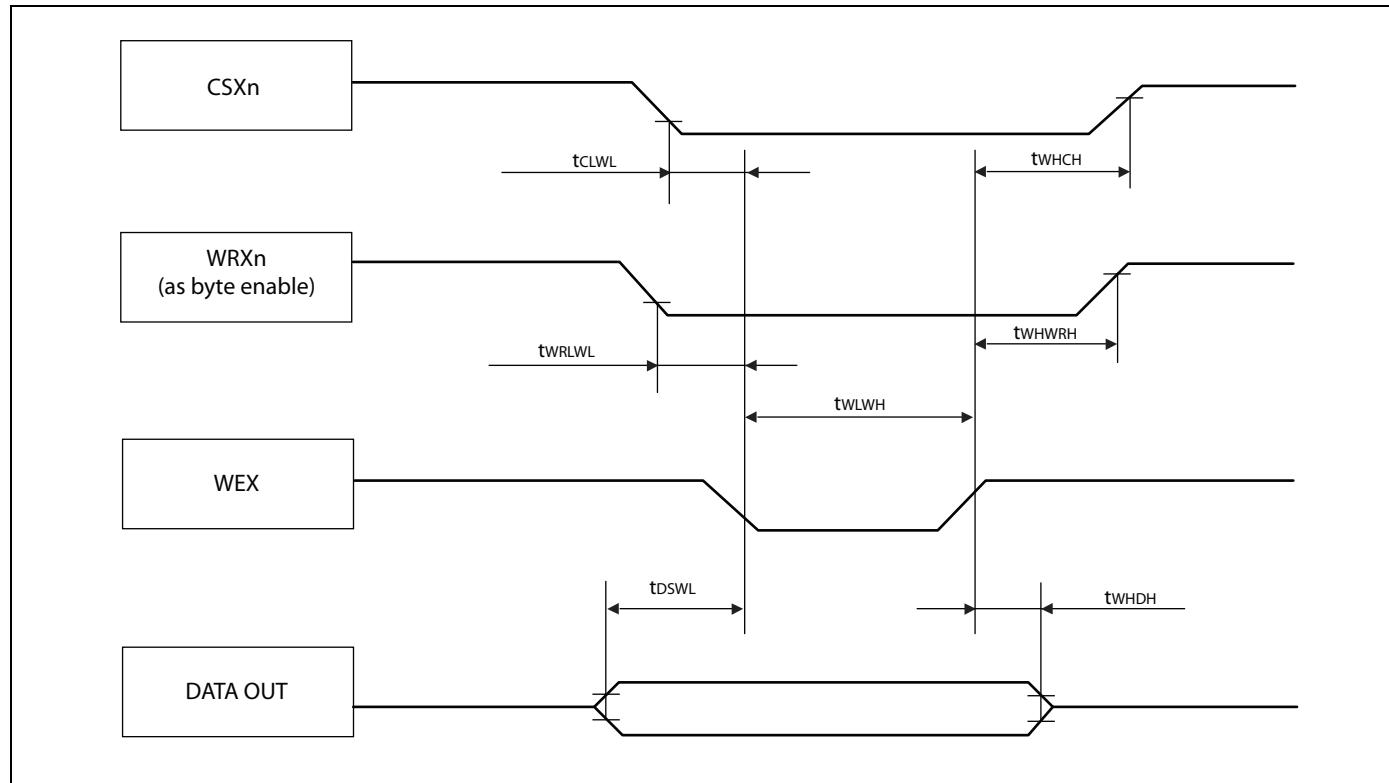
**Asynchronous write access - no byte control type**
