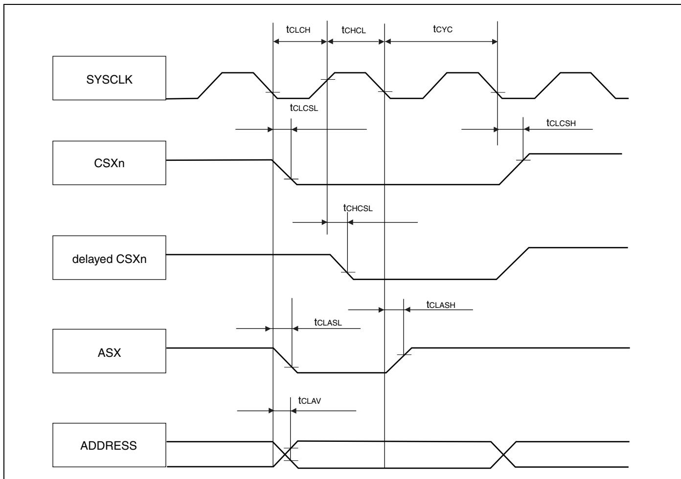
**Synchronous/Asynchronous read access**
