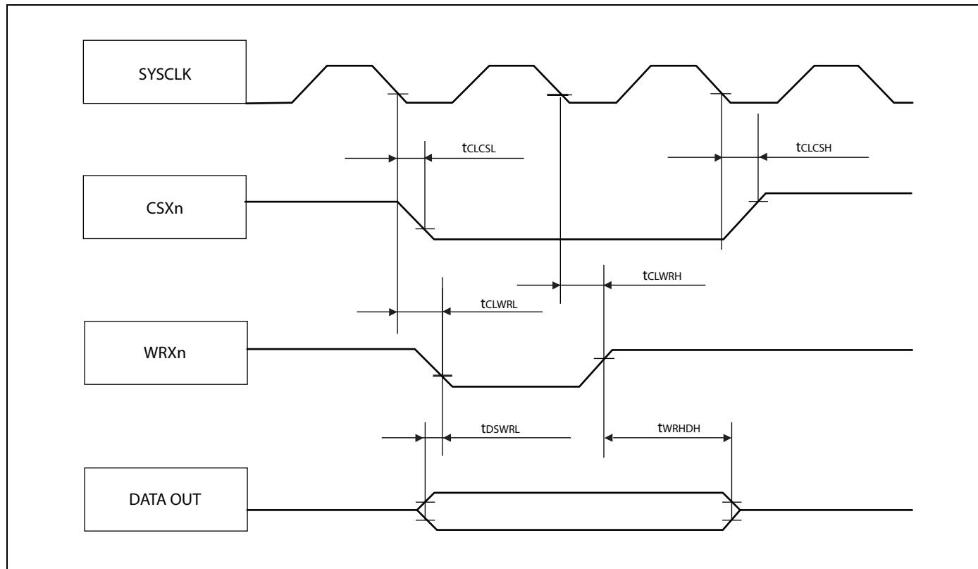
**Asynchronous write access - byte control type**
