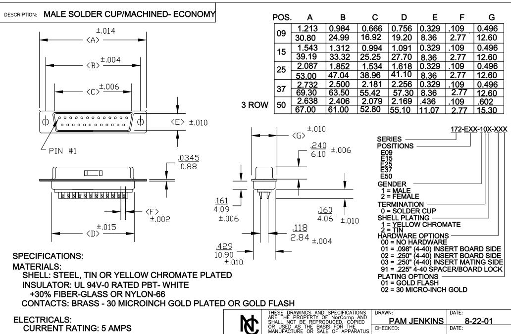
CONTACT RESISTANCE: 15 mOHMS MAX INSULTOR RESISTANCE: 1000 MOHMS MIN VOLTAGE: 500V AC FOR 1 MINUTE TEMPERATURE: -50°C TO +100°C
