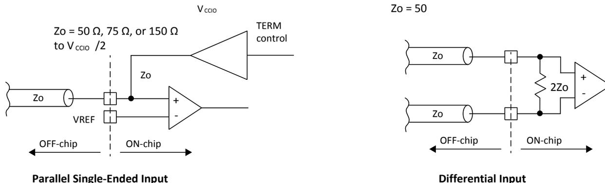
Figure 2.26. On-Chip Termination
