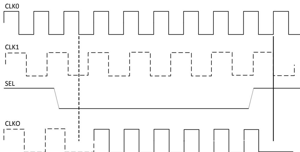
**Figure 2.7. DCS Waveforms**
