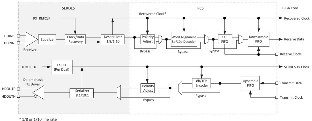
**Figure 2.28. Simplified Channel Block Diagram for SERDES/PCS Block**
