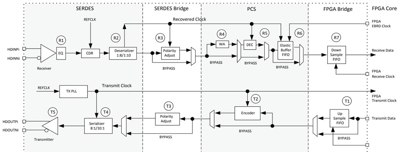
**Figure 3.13. Transmitter and Receiver Latency Block Diagram**
