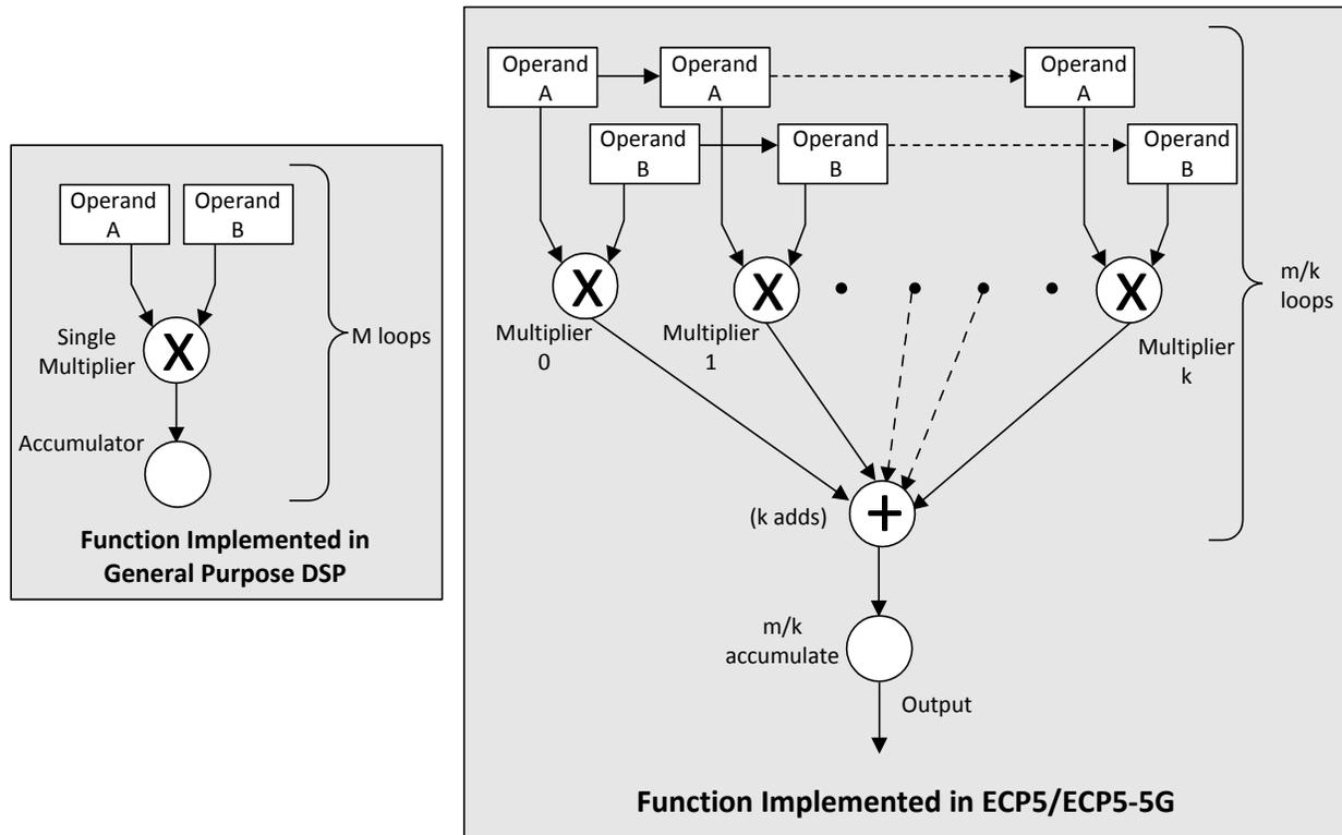
Figure 2.13. Comparison of General DSP and ECP5/ECP5-5G Approaches
