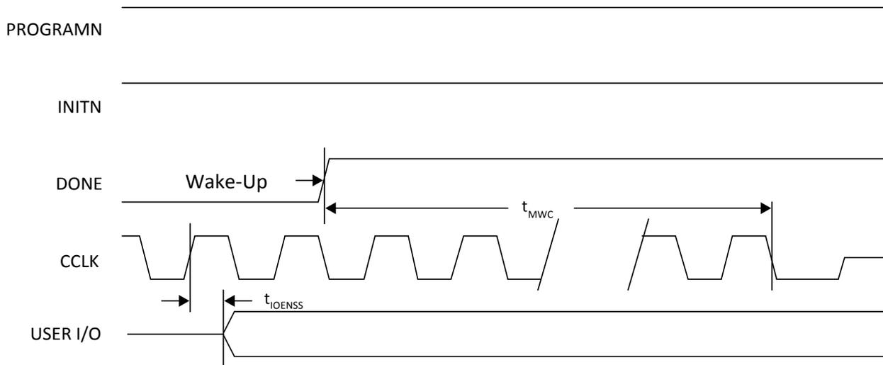
**Figure 3.21. Wake-Up Timing**
