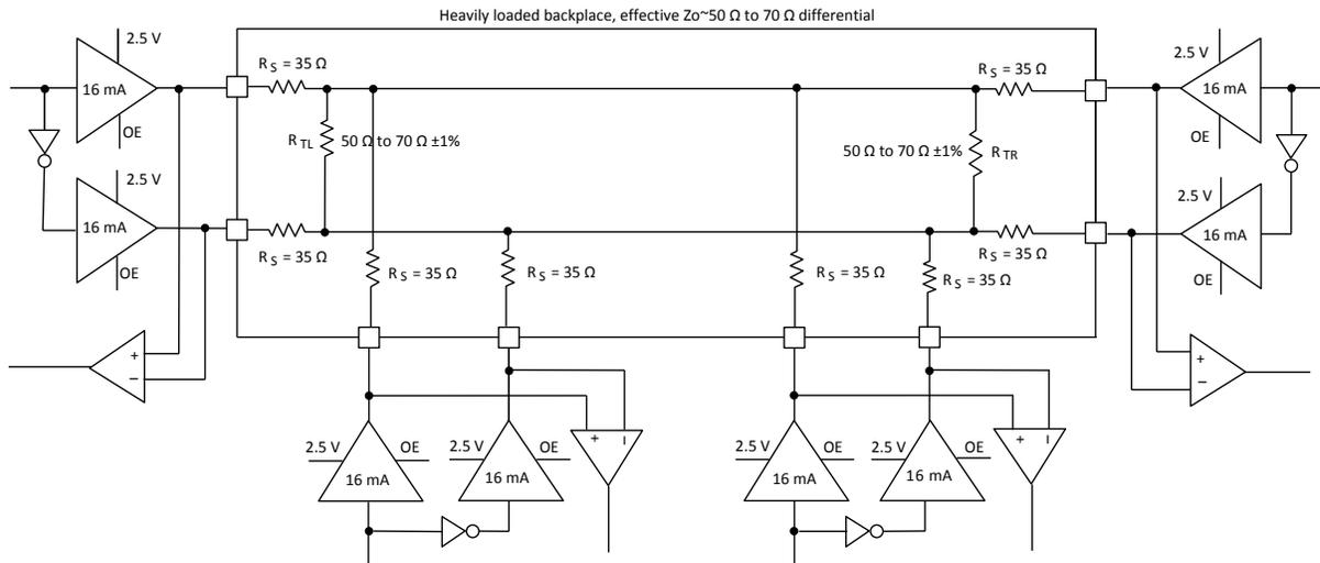
**Figure 3.4. MLVDS25 (Multipoint Low Voltage Differential Signaling)**
