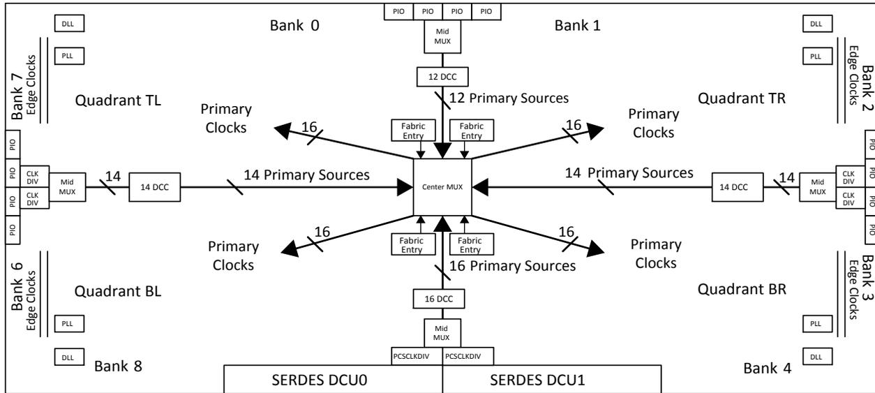
Figure 2.6. LFE5UM/LFE5UM5G-85 Clocking
