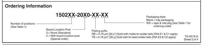
2 mm x 2 mm Straight Surface Mount, Straight and Right Angle Plated Through-Hole 1502 Series
