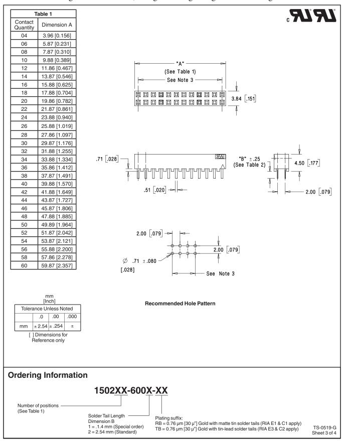
2 mm x 2 mm Straight Surface Mount, Straight and Right Angle Plated Through-Hole 1502 Series
