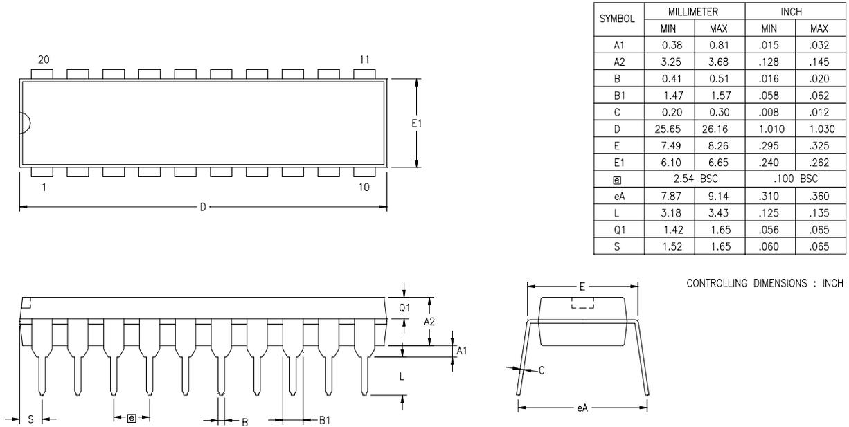
Figure 42. 20-Pin Plastic Dual Inline Package (PDIP)
