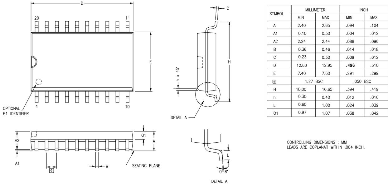
Figure 43. 20-Pin Small Outline Integrated Circuit Package (SOIC)
