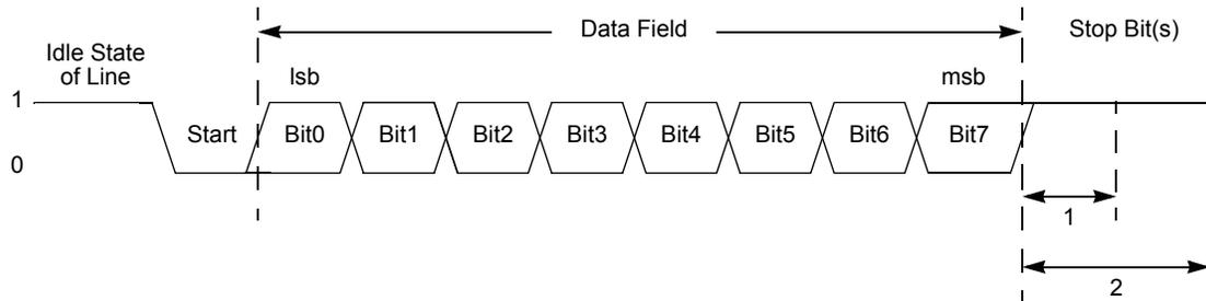
**Figure 11. UART Asynchronous Data Format without Parity**
