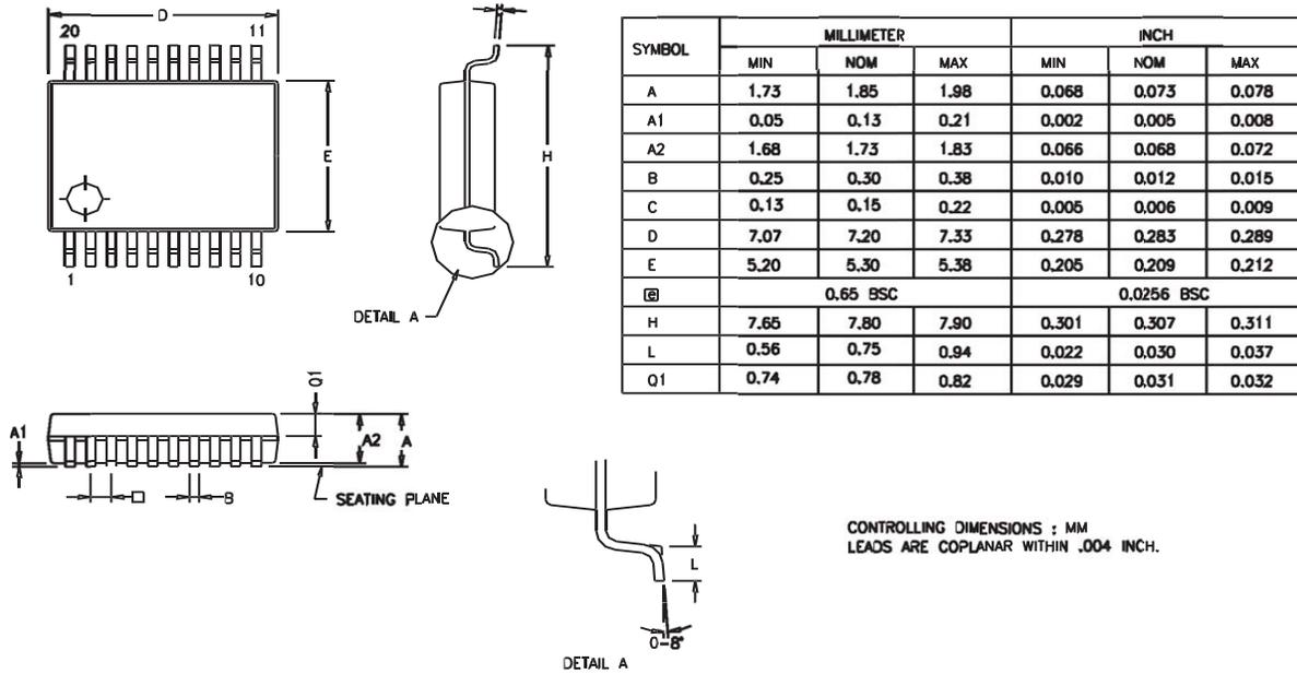
Figure 44. 20-Pin Small Shrink Outline Package (SSOP)
