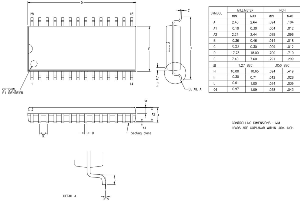
Figure 46. 28-Pin Small Outline Integrated Circuit Package (SOIC)
