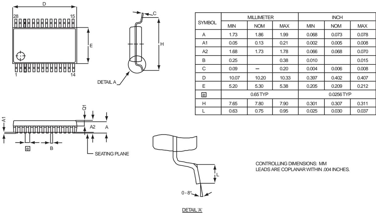
Figure 47. 28-Pin Small Shrink Outline Package (SSOP)
