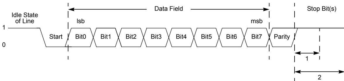
**Figure 12. UART Asynchronous Data Format with Parity**
