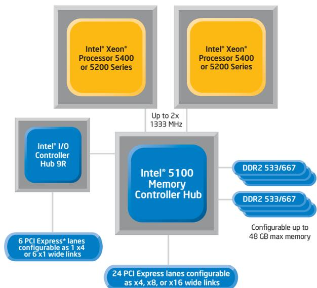
Figure 3: Intel® 5100 Memory Controller Hub chipset-based platforms
