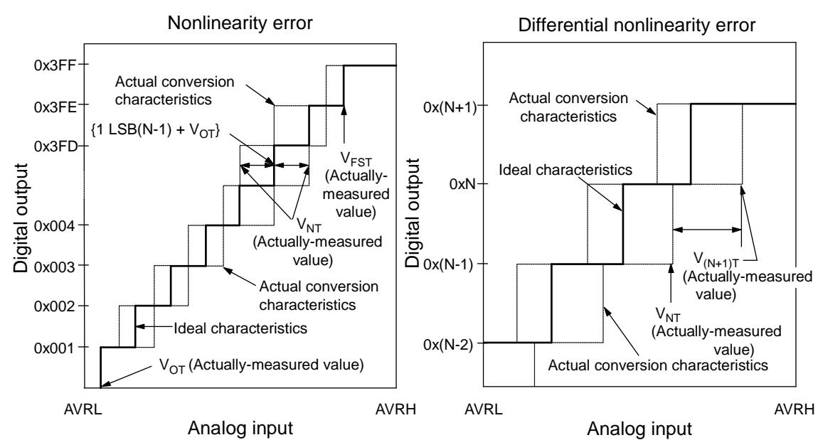
$$\text{Nonlinearity error of digital output } N = \frac{V_{NT} - \{1 \text{ LSB} \times (N - 1) + V_{OT}\}}{1 \text{ LSB}} \text{ [LSB]}$$
