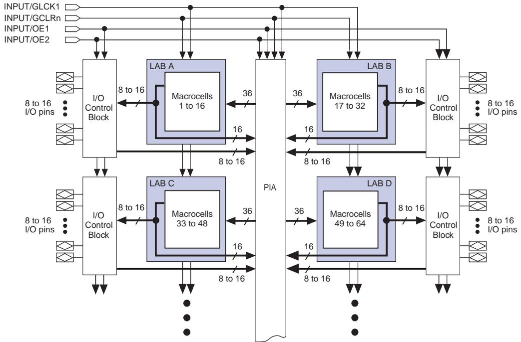
Figure 2 shows the architecture of MAX 7000E and MAX 7000S devices.
