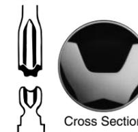
The cross section is in the shape of the letter W. The two points on the bottom work as guide rails, preventing the pins from becoming twisted. The fin parts on the upper part change shape to fit into the through hole of the PCB.
