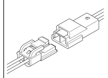
The YLN connector adds variations in shape to the existing color variations of the YL connector in order to improve identification of connectors. Moreover, this connector has a mechanism to prevent incomplete mating by utilizing the inertial force generated when the plug and receptacle are mated and therefore, ensures complete mating.
