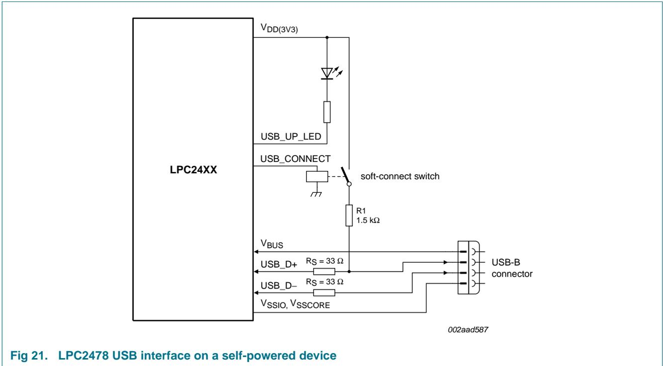
Fig 21. LPC2478 USB interface on a self-powered device
