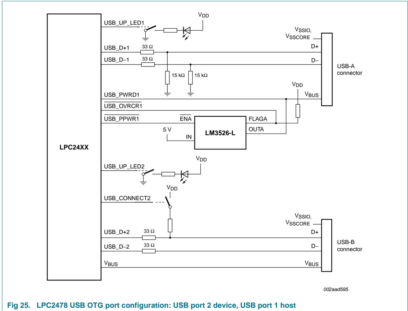
Fig 25. LPC2478 USB OTG port configuration: USB port 2 device, USB port 1 host
