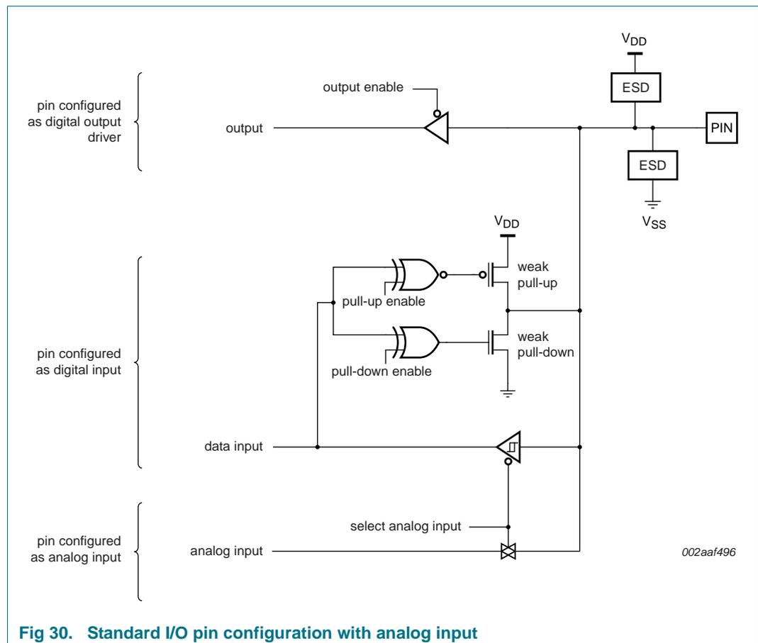
Fig 30. Standard I/O pin configuration with analog input
