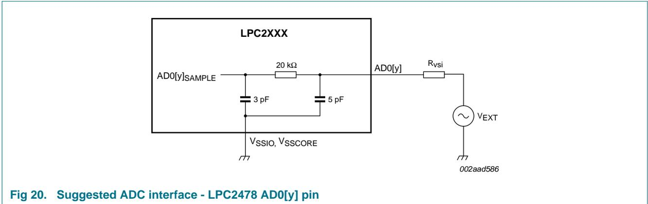
Fig 20. Suggested ADC interface - LPC2478 AD0[y] pin
