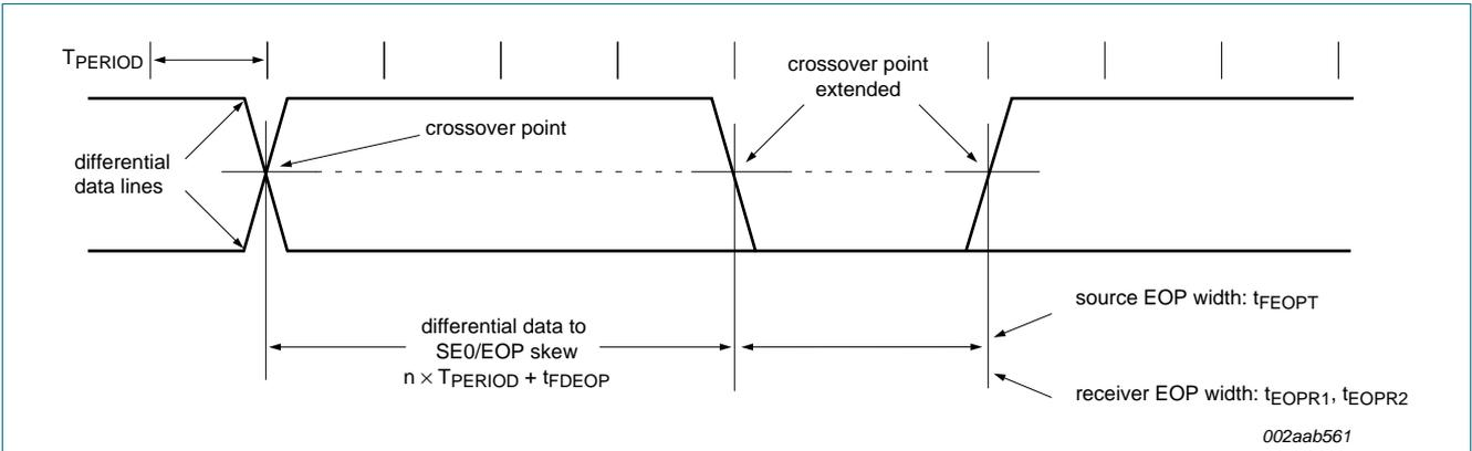
Fig 16. Differential data-to-EOP transition skew and EOP width
