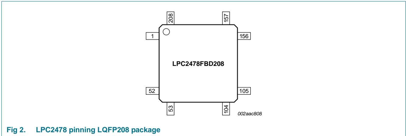
Fig 2. LPC2478 pinning LQFP208 package
