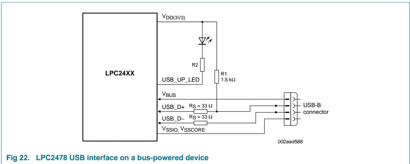
Fig 22. LPC2478 USB interface on a bus-powered device
