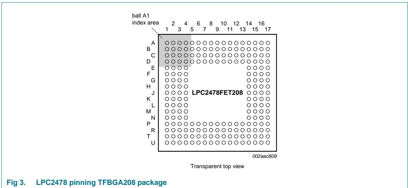
Fig 3. LPC2478 pinning TFBGA208 package
