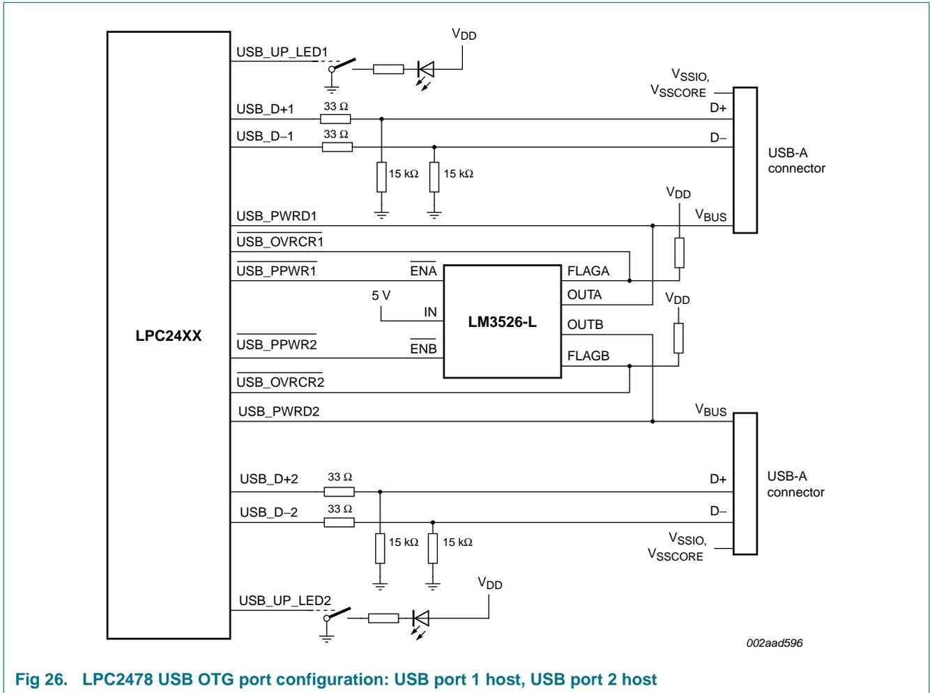
Fig 26. LPC2478 USB OTG port configuration: USB port 1 host, USB port 2 host
