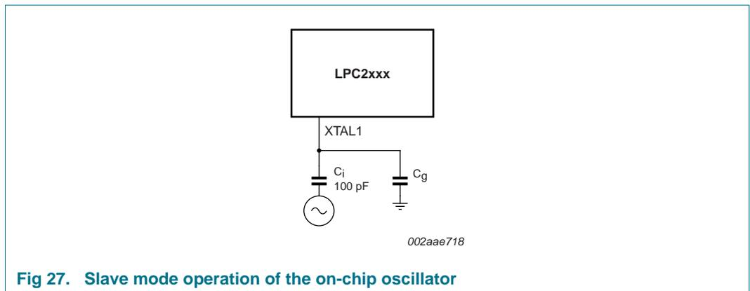
Fig 27. Slave mode operation of the on-chip oscillator
