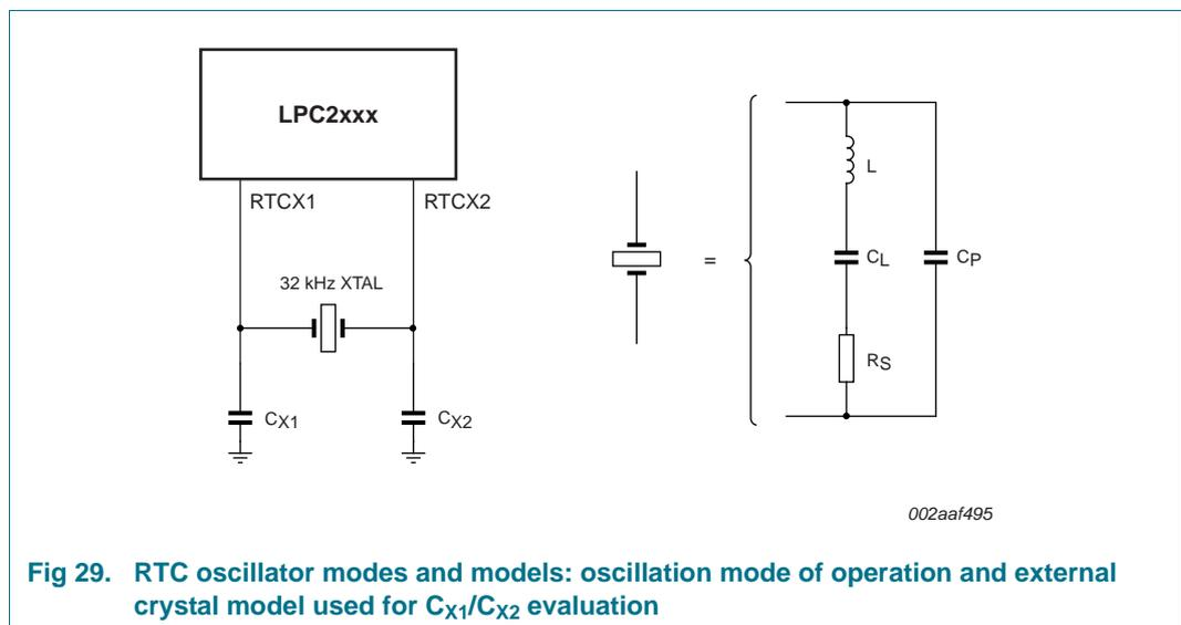
The RTC external oscillator circuit is shown in [Figure 29](#). Since the feedback resistance is integrated on chip, only a crystal, the capacitances  $C_{X1}$  and  $C_{X2}$  need to be connected externally to the microcontroller.
