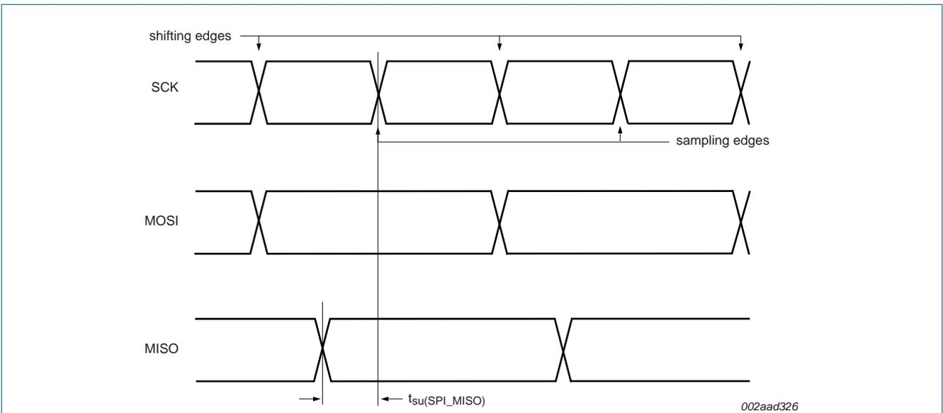
Fig 17. MISO line set-up time in SSP Master mode
