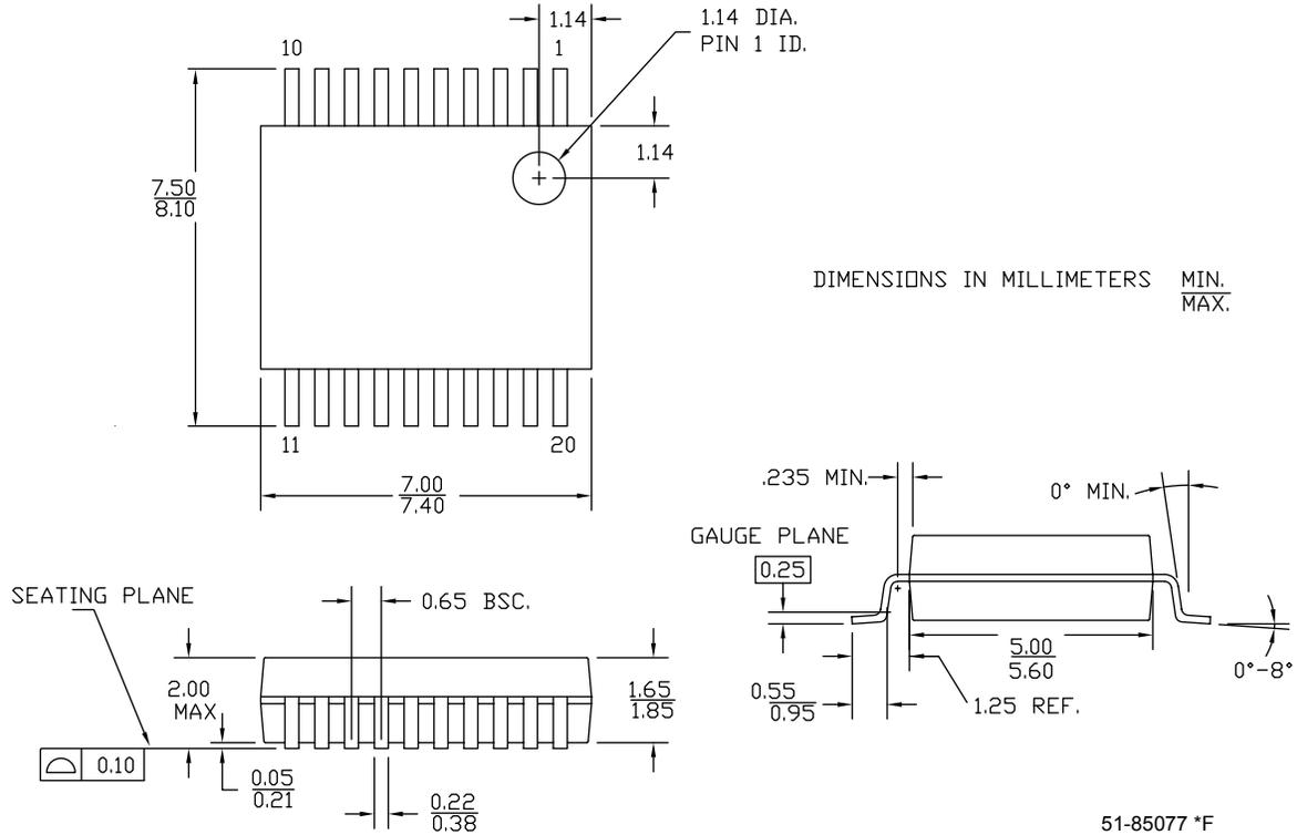
**Figure 21. 20-Pin (300-Mil) Molded SOIC**
