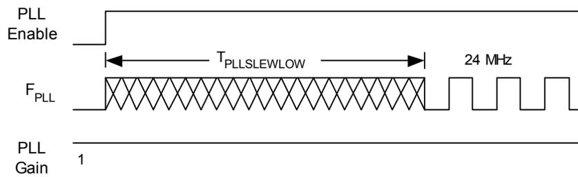
**Figure 13. External Crystal Oscillator Startup Timing Diagram**
